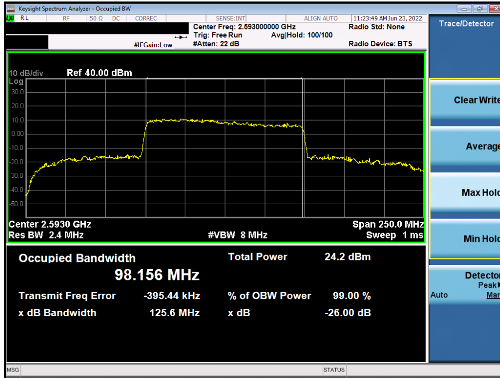
Plot 7-82. Occupied Bandwidth Plot (NR Band n41 - 100MHz 16-QAM - Full RB – Ant8)
