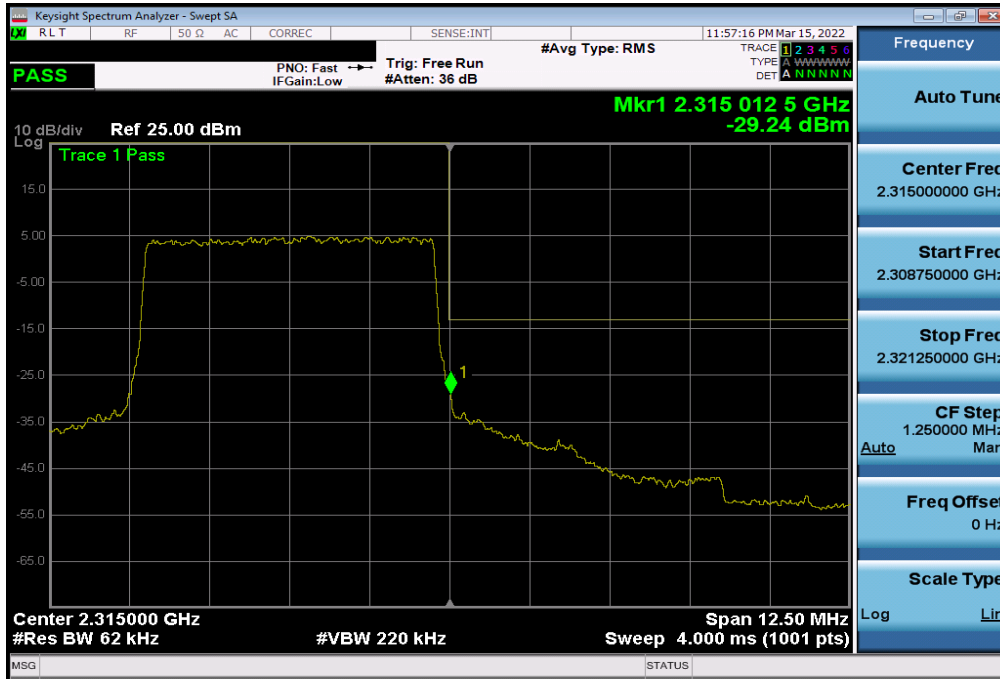
Plot 7-169. Upper Band Edge Plot (LTE Band 30 - 10MHz QPSK – Full RB - Ant1)
