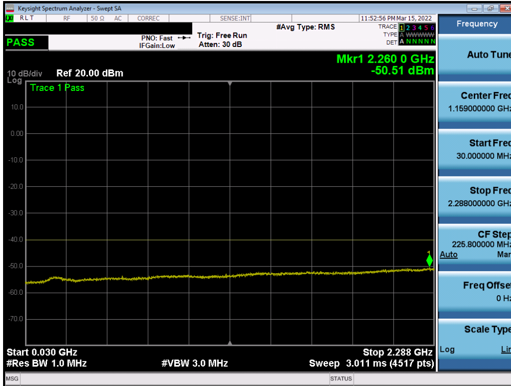
Plot 7-83. Conducted Spurious Plot (LTE Band 30 - 10MHz QPSK - RB Size 1, RB Offset 0 - Ant1)
