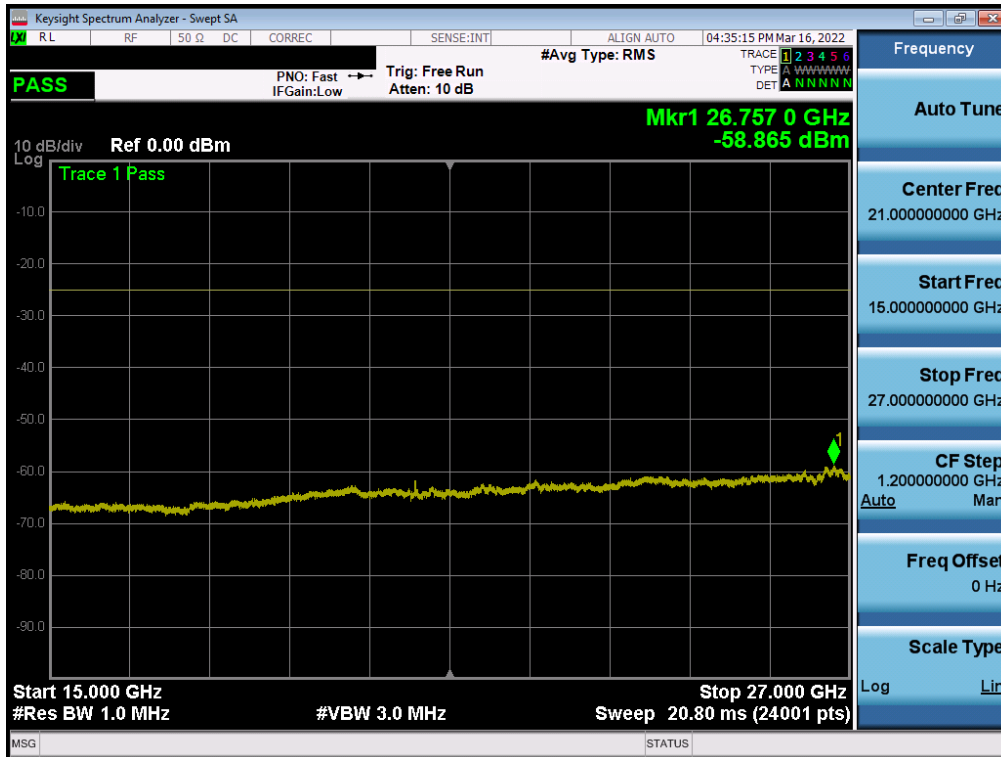
Plot 7-94. Conducted Spurious Plot (LTE Band 7 - 20MHz QPSK - RB Size 1, RB Offset 0 - High Channel - Ant1)
