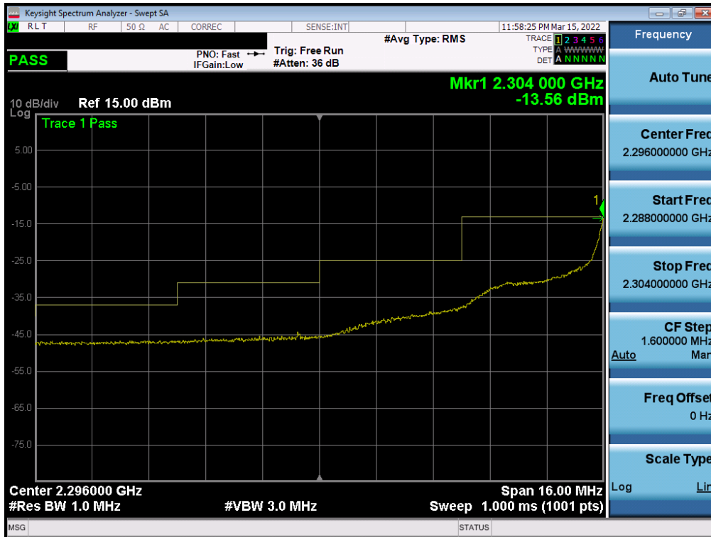
Plot 7-172. Extended Lower Band Edge Plot (LTE Band 30 - 5MHz QPSK – Full RB - Ant1)
