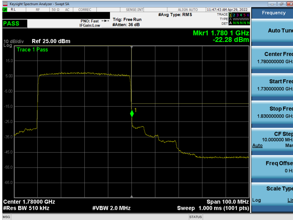
Plot 7-245. Upper Band Edge Plot (NR Band n66 – 40.0MHz - Full RB - Ant4)
