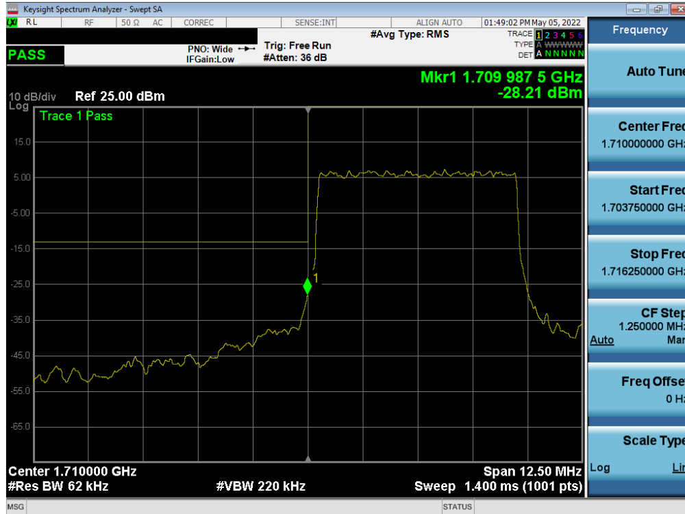
Plot 7-263. Lower Band Edge Plot (NR Band n66 – 5.0MHz - Full RB - Ant4)
