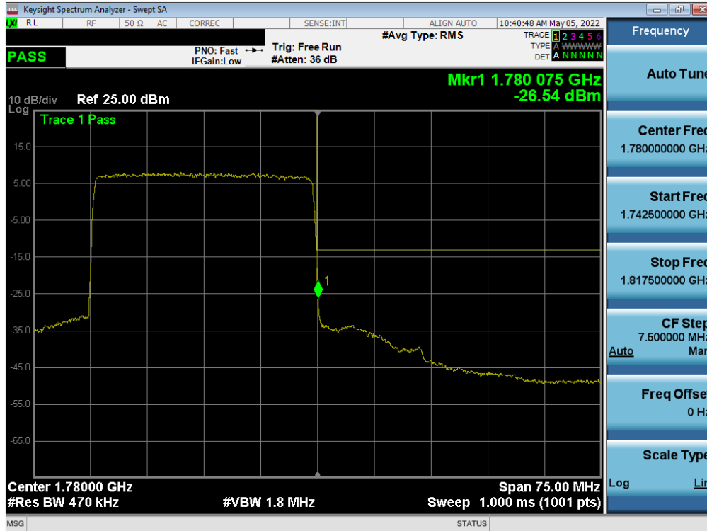
Plot 7-249. Upper Band Edge Plot (NR Band n66 – 30.0MHz - Full RB - Ant4)
