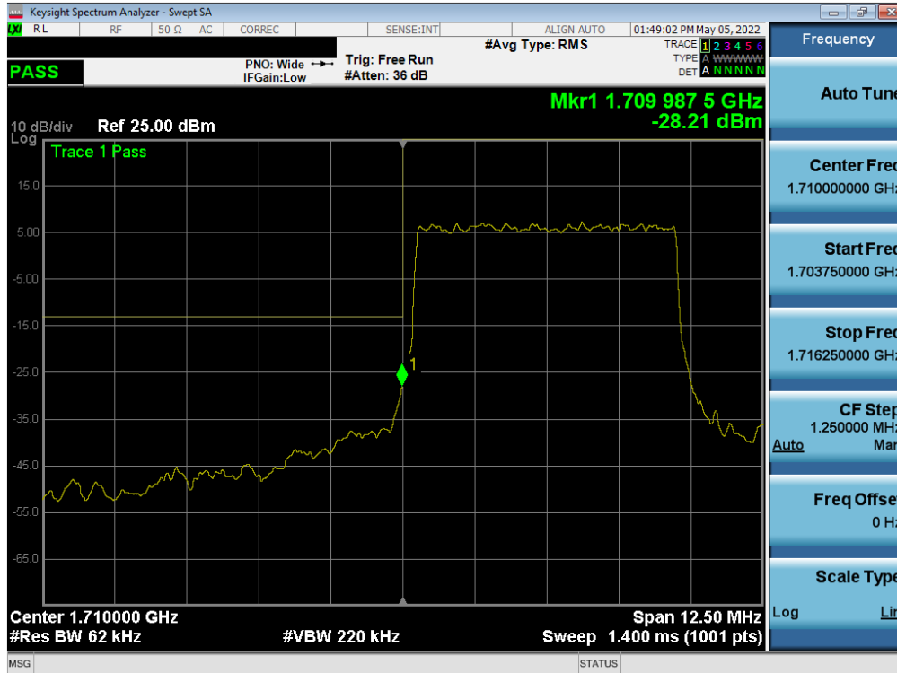
Plot 7-235. Lower Band Edge Plot (NR Band n66 – 5.0MHz - Full RB - Ant1)
