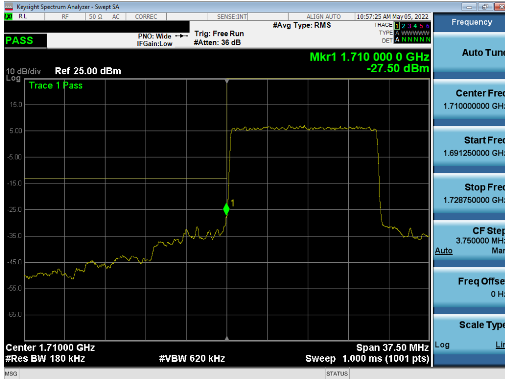
Plot 7-255. Lower Band Edge Plot (NR Band n66 – 15.0MHz - Full RB - Ant4)
