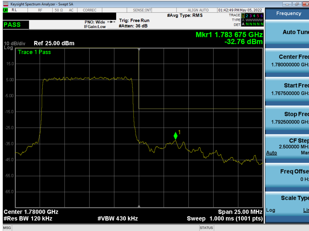
Plot 7-233. Upper Band Edge Plot (NR Band n66 - 10.0MHz - Full RB - Ant1)
