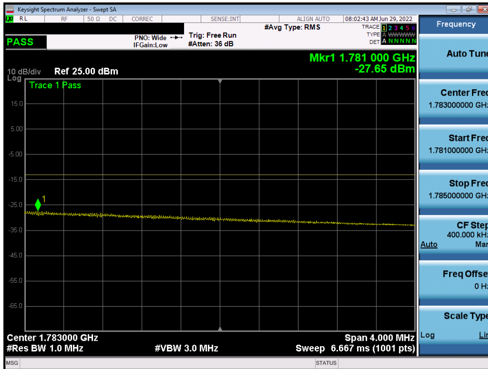
Plot 7-250. Upper Extended Band Edge Plot (NR Band n66 – 30.0MHz - Full RB - Ant4)
