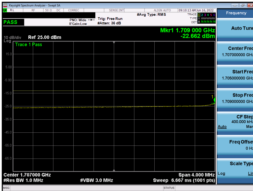
Plot 7-240. Lower Extended Band Edge Plot (ULCA LTE Band 66 - Ant1)
