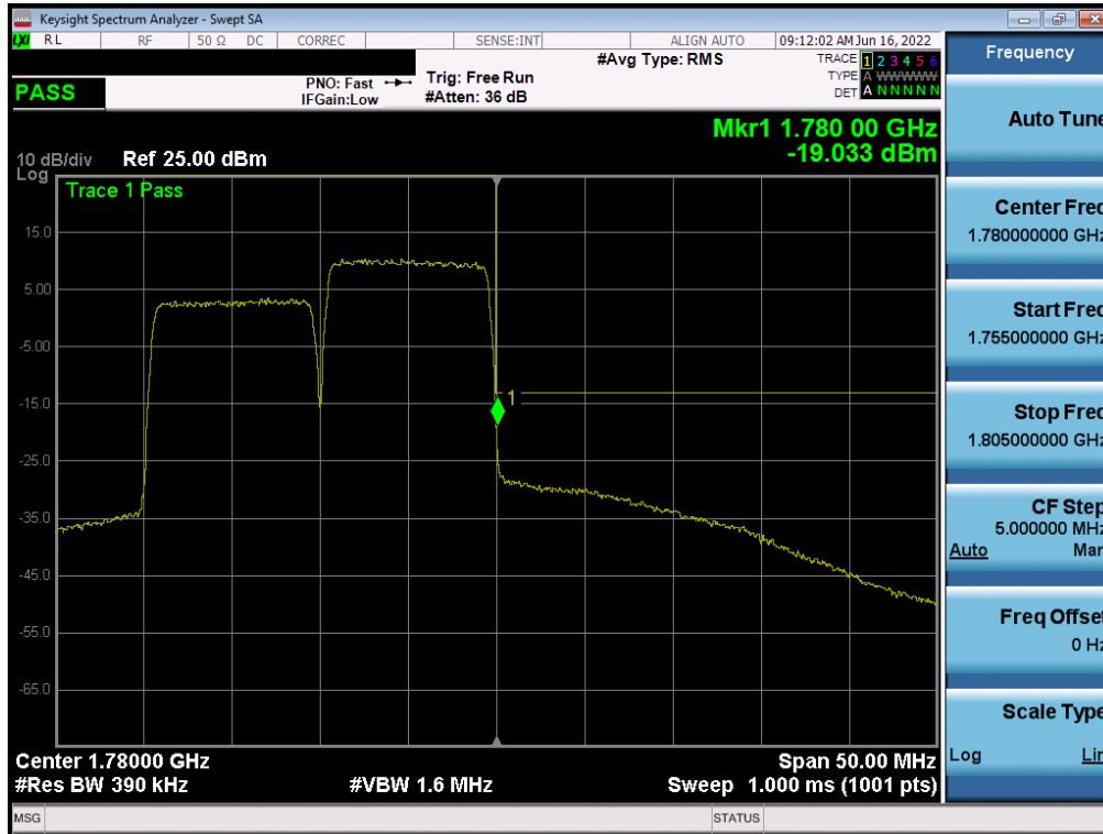
Plot 7-241. Upper Band Edge Plot (ULCA LTE Band 66 - Ant1)
