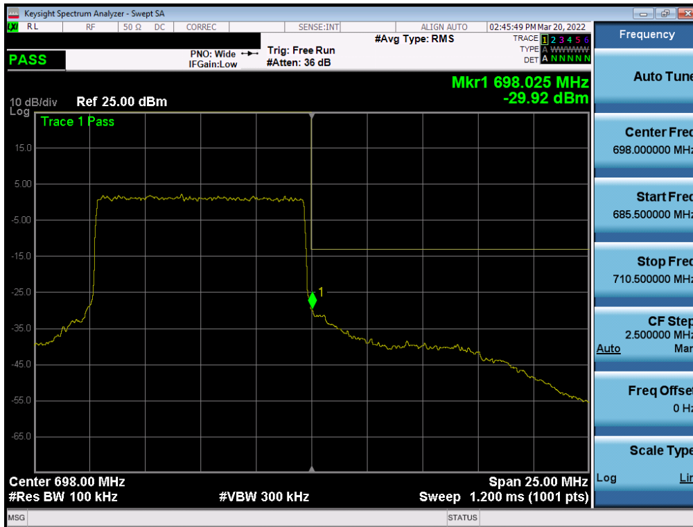
Plot 7-176. Upper Band Edge Plot (NR Band n71 – 10.0MHz - Full RB - Ant1)
