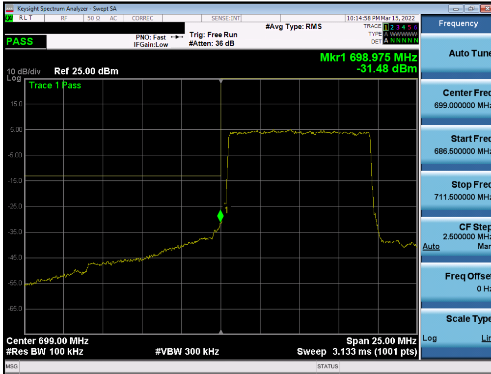
Plot 7-155. Lower Band Edge Plot (LTE Band 12 - 10MHz QPSK – Full RB - Ant1)
