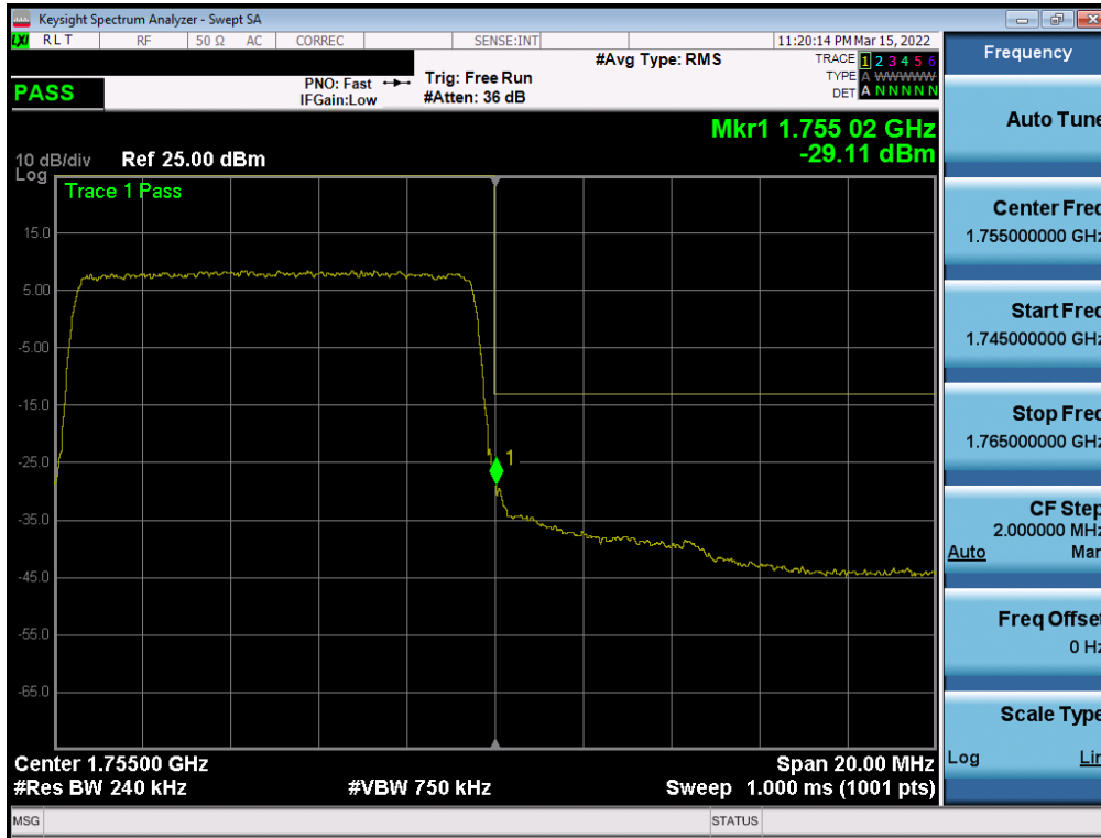
Plot 7-193. Upper Band Edge Plot (LTE Band 4 - 10MHz QPSK – Full RB - Ant1)
