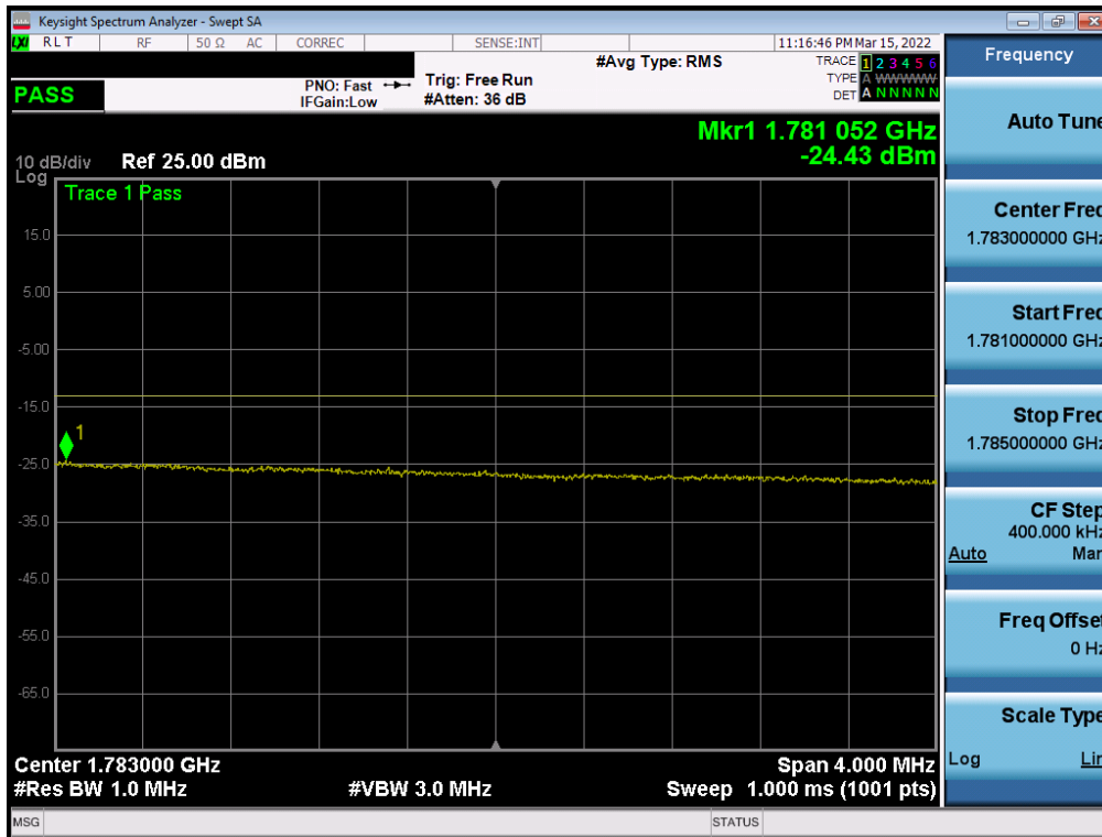
Plot 7-190. Upper Extended Band Edge Plot (LTE Band 66 - 15MHz QPSK – Full RB - Ant1)
