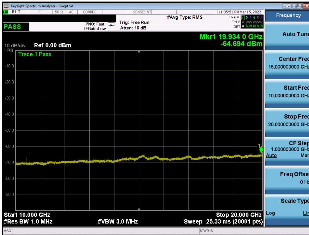
Plot 7-116. Conducted Spurious Plot (LTE Band 66/4 - 20MHz QPSK - 1 RB - Mid Channel – Ant1)
