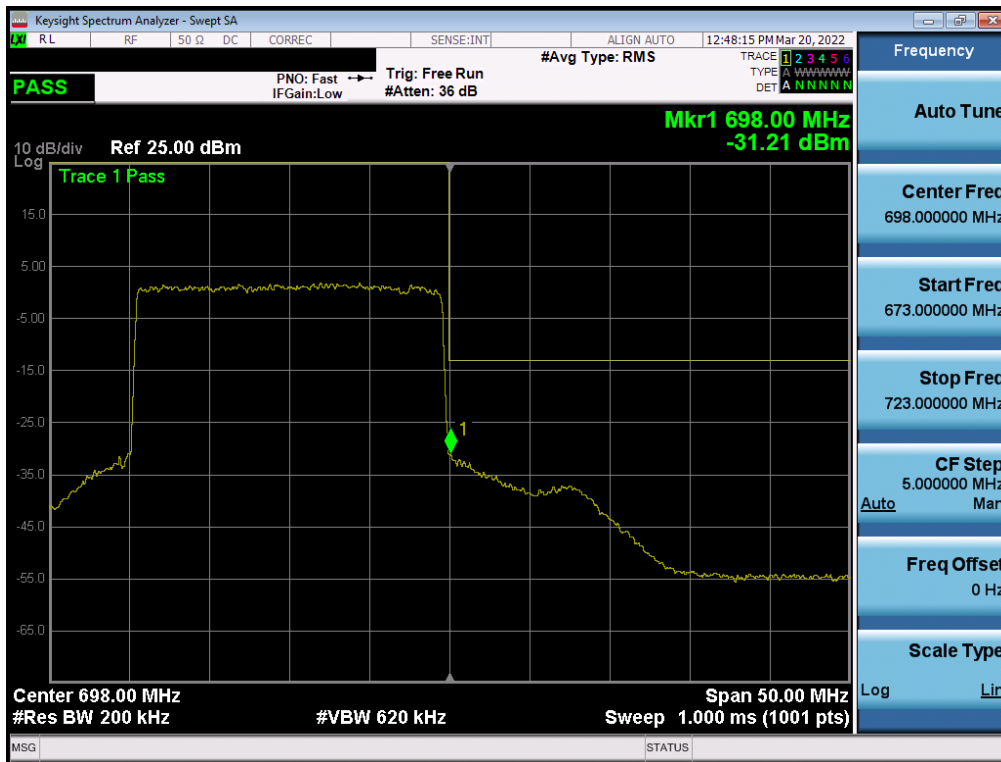
Plot 7-172. Upper Band Edge Plot (NR Band n71 – 20.0MHz - Full RB - Ant1)
