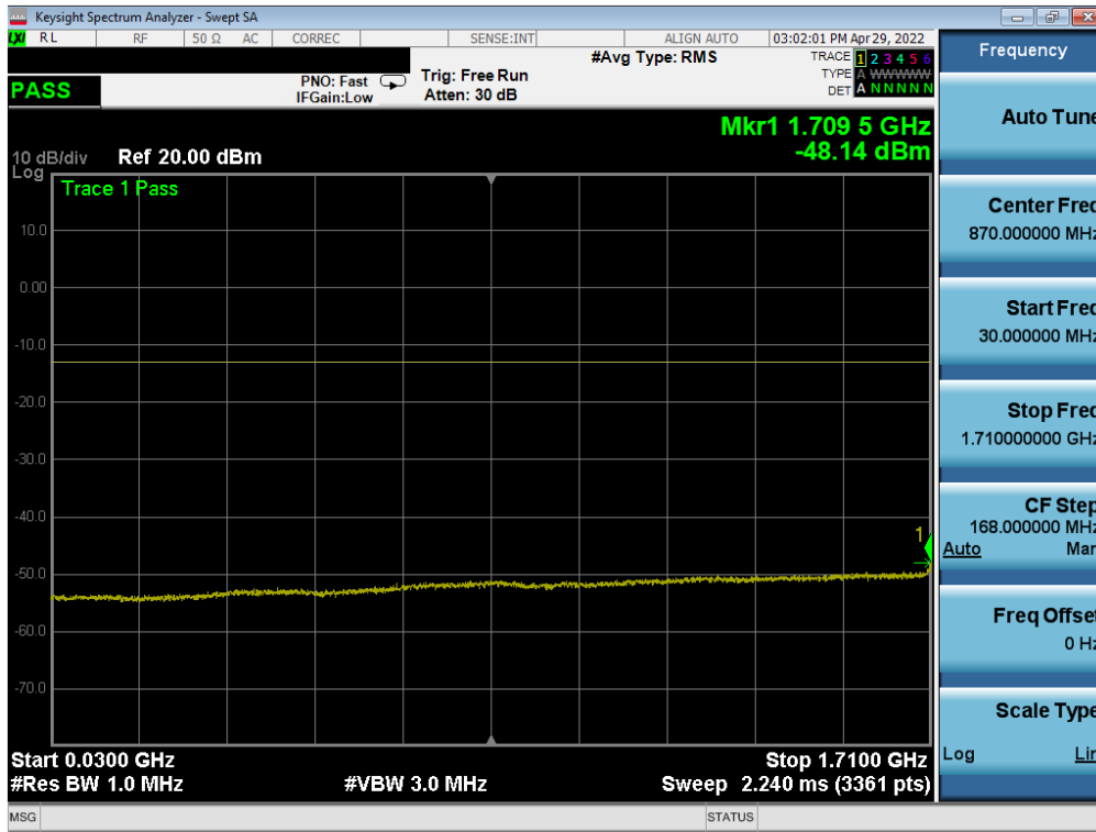
Plot 7-120. Conducted Spurious Plot (NR Band n66 -40.0MHz - 1 RB - Low Channel - Ant1)
