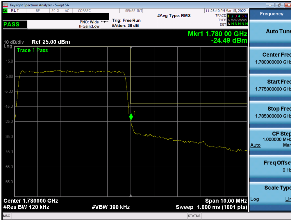
Plot 7-201. Upper Band Edge Plot (LTE Band 66 - 5MHz QPSK – Full RB - Ant1)
