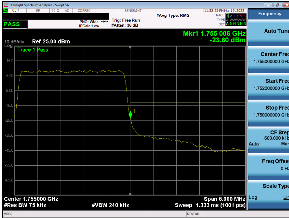
Plot 7-205. Upper Band Edge Plot (LTE Band 4 - 3MHz QPSK – Full RB - Ant1)
