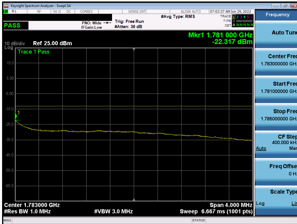
Plot 7-230. Upper Extended Band Edge Plot (NR Band n66 - 15.0MHz - Full RB - Ant1)
