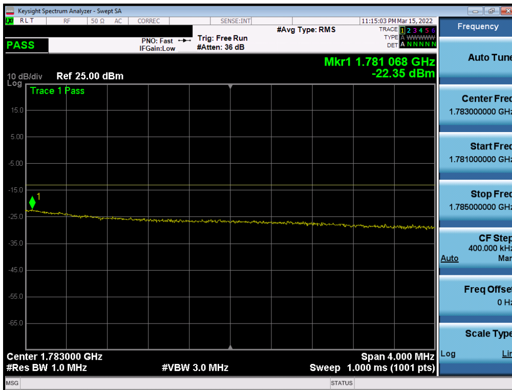
Plot 7-184. Channel Edge Plot (LTE Band 66 - 20MHz QPSK – Full RB - Ant1)
