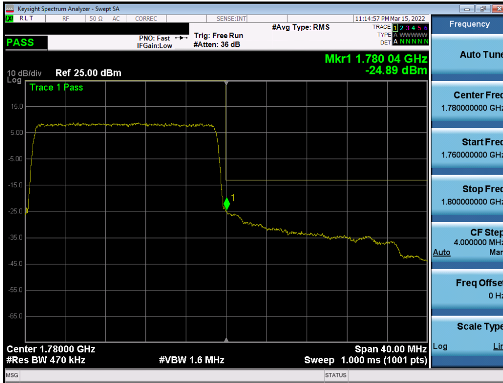
Plot 7-183. Upper Band Edge Plot (LTE Band 66 - 20MHz QPSK – Full RB - Ant1)
