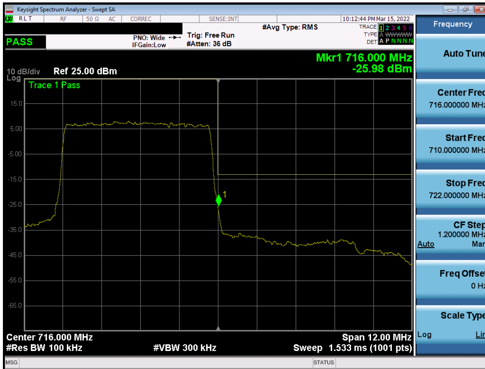
Plot 7-158. Upper Band Edge Plot (LTE Band 12 - 5MHz QPSK – Full RB - Ant1)
