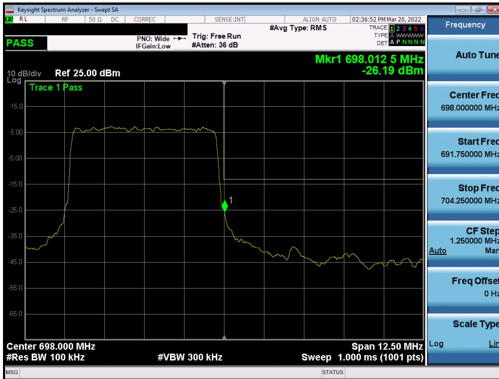
Plot 7-178. Upper Band Edge Plot (NR Band n71 – 5.0MHz - Full RB - Ant1)
