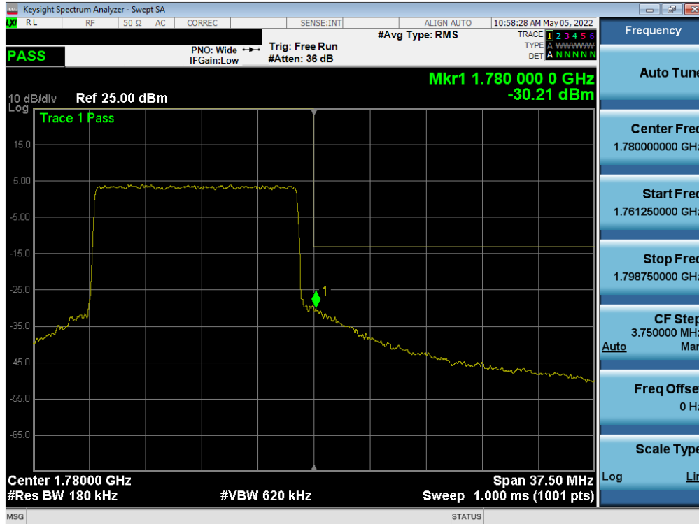
Plot 7-229. Upper Band Edge Plot (NR Band n66 - 15.0MHz - Full RB - Ant1)
