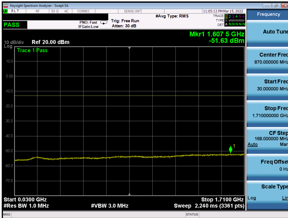
Plot 7-114. Conducted Spurious Plot (LTE Band 66/4 - 20MHz QPSK - 1 RB - Mid Channel – Ant1)
