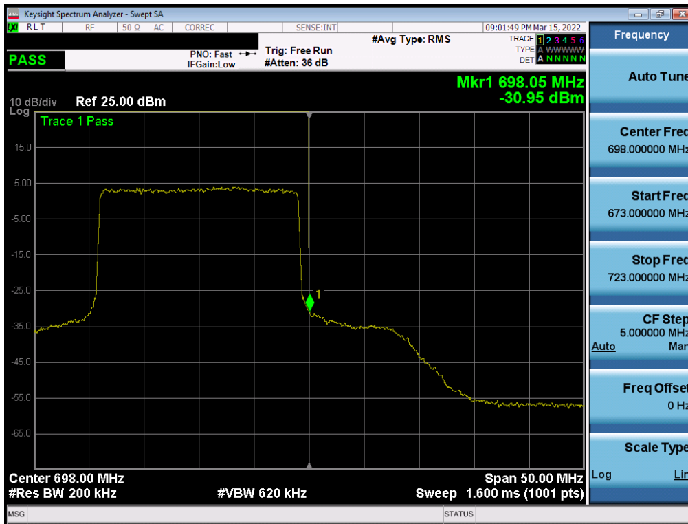
Plot 7-148. Upper Band Edge Plot (LTE Band 71 - 20MHz QPSK – Full RB - Ant1)
