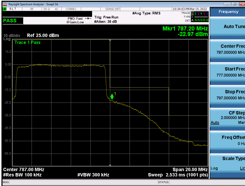
Plot 7-165. Upper Band Edge Plot (LTE Band 13 - 10MHz QPSK – Full RB - Ant1)
