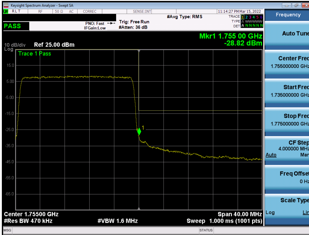
Plot 7-181. Upper Band Edge Plot (LTE Band 4 - 20MHz QPSK – Full RB - Ant1)
