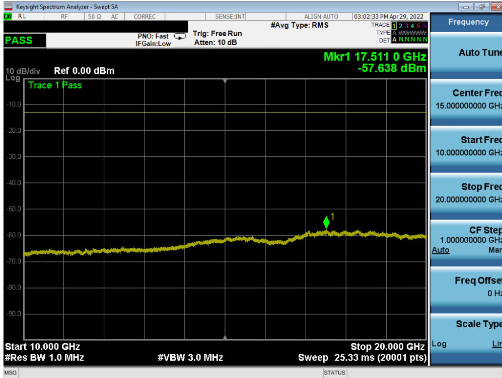
Plot 7-122. Conducted Spurious Plot (NR Band n66 - 40.0MHz - 1 RB - Low Channel - Ant1)
