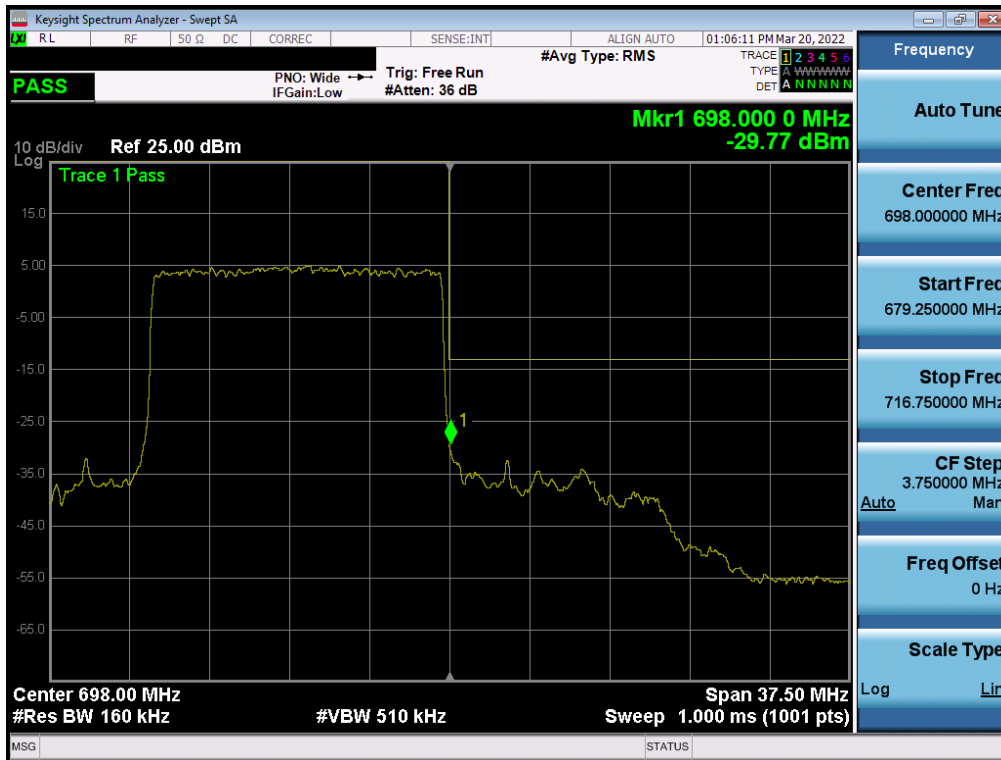
Plot 7-174. Upper Band Edge Plot (NR Band n71 – 15.0MHz - Full RB - Ant1)
