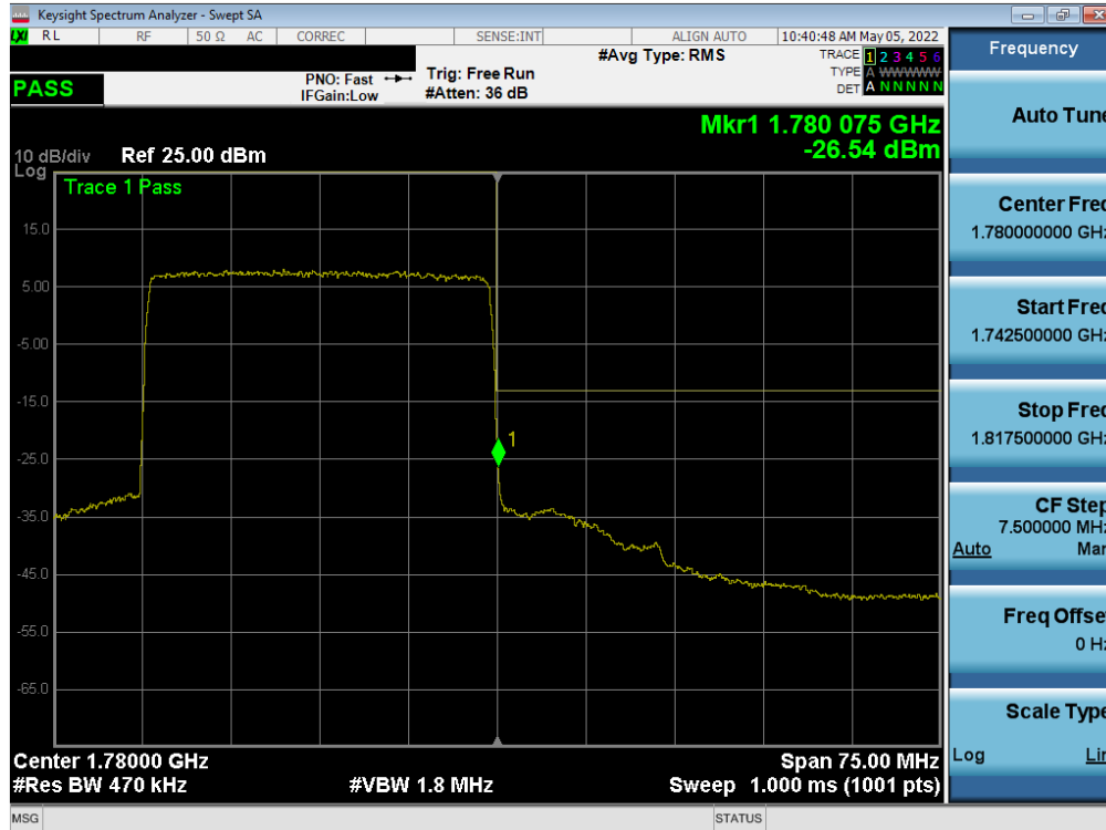
Plot 7-221. Upper Band Edge Plot (NR Band n66 - 30.0MHz - Full RB - Ant1)
