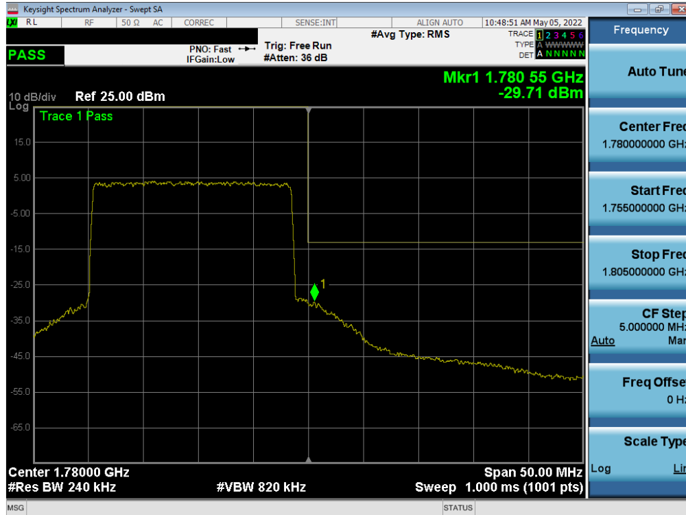
Plot 7-225. Upper Band Edge Plot (NR Band n66 - 20.0MHz - Full RB - Ant1)
