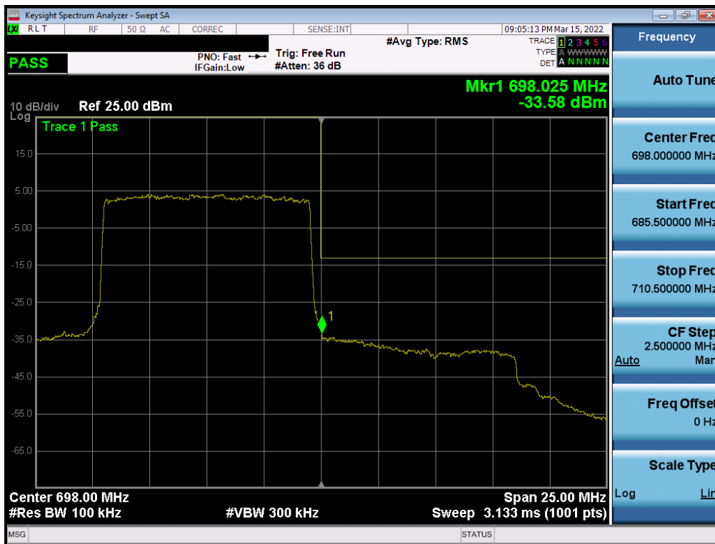
Plot 7-152. Upper Band Edge Plot (LTE Band 71 - 10MHz QPSK – Full RB - Ant1)
