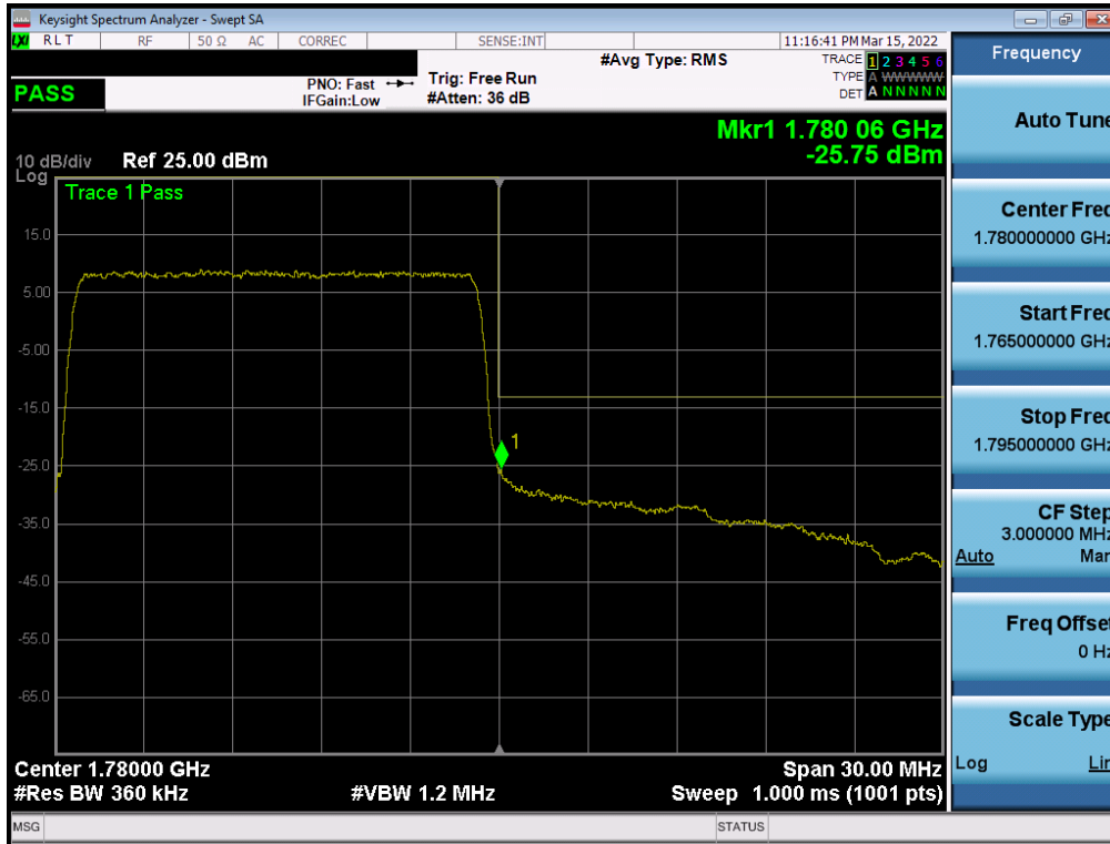
Plot 7-189. Upper Band Edge Plot (LTE Band 66 - 15MHz QPSK – Full RB - Ant1)
