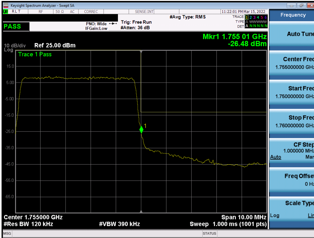
Plot 7-199. Upper Band Edge Plot (LTE Band 4 - 5MHz QPSK – Full RB - Ant1)
