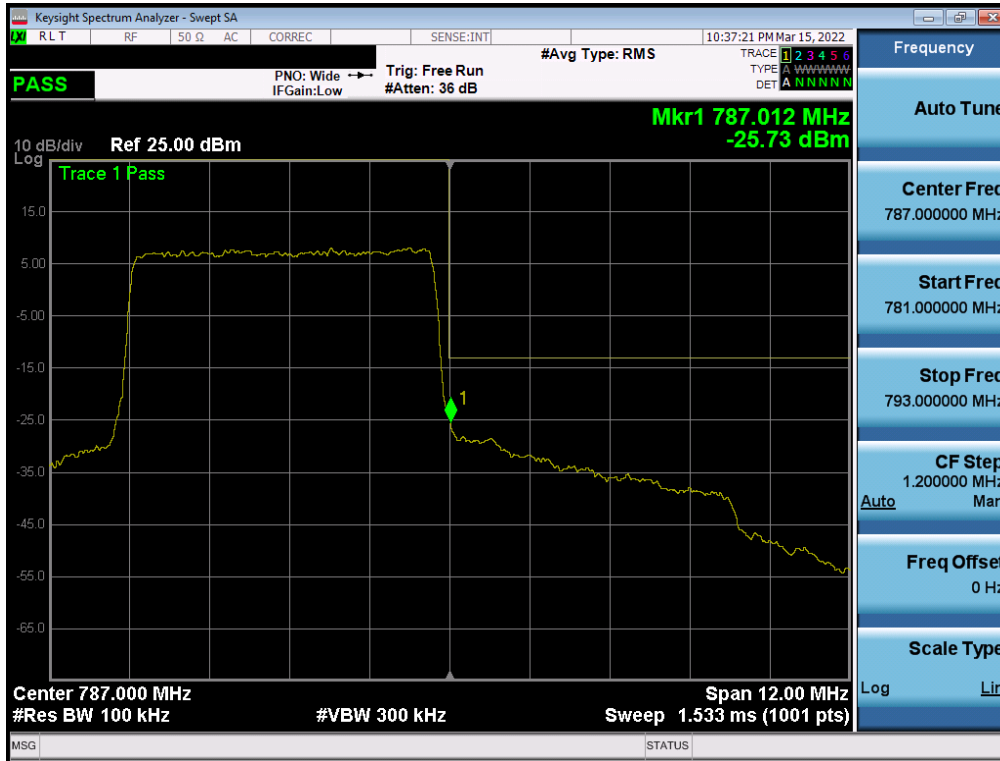
Plot 7-169. Upper Band Edge Plot (LTE Band 13 - 5MHz QPSK – Full RB - Ant1)
