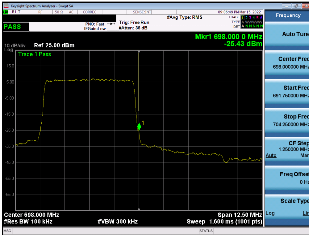
Plot 7-154. Upper Band Edge Plot (LTE Band 71 - 5MHz QPSK – Full RB - Ant1)
