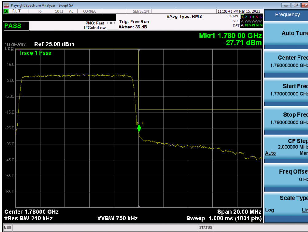
Plot 7-195. Upper Band Edge Plot (LTE Band 66 - 10MHz QPSK – Full RB - Ant1)
