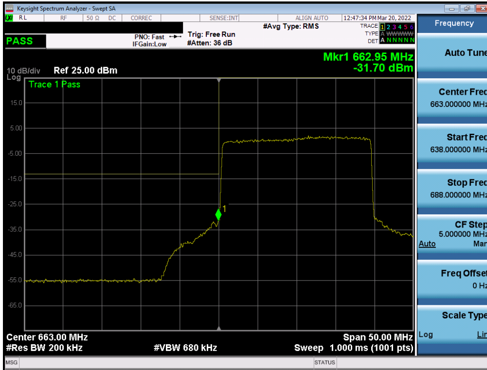
Plot 7-171. Lower Band Edge Plot (NR Band n71 – 20.0MHz - Full RB - Ant1)
