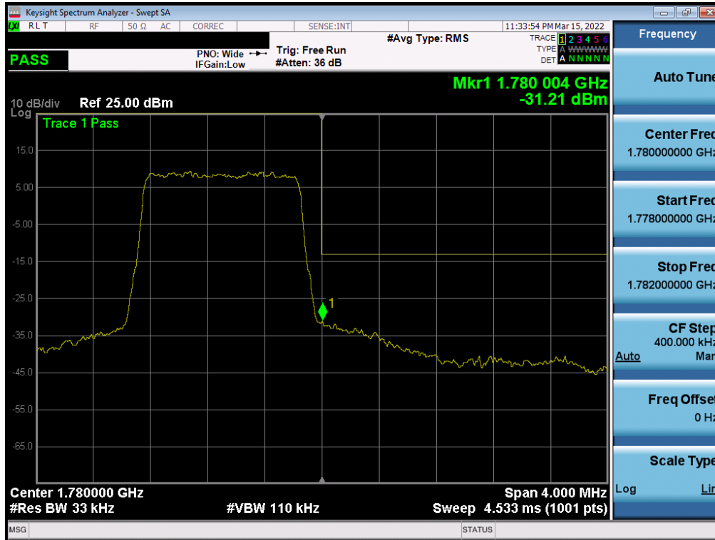
Plot 7-213. Upper Band Edge Plot (LTE Band 66 – 1.4MHz QPSK – Full RB - Ant1)
