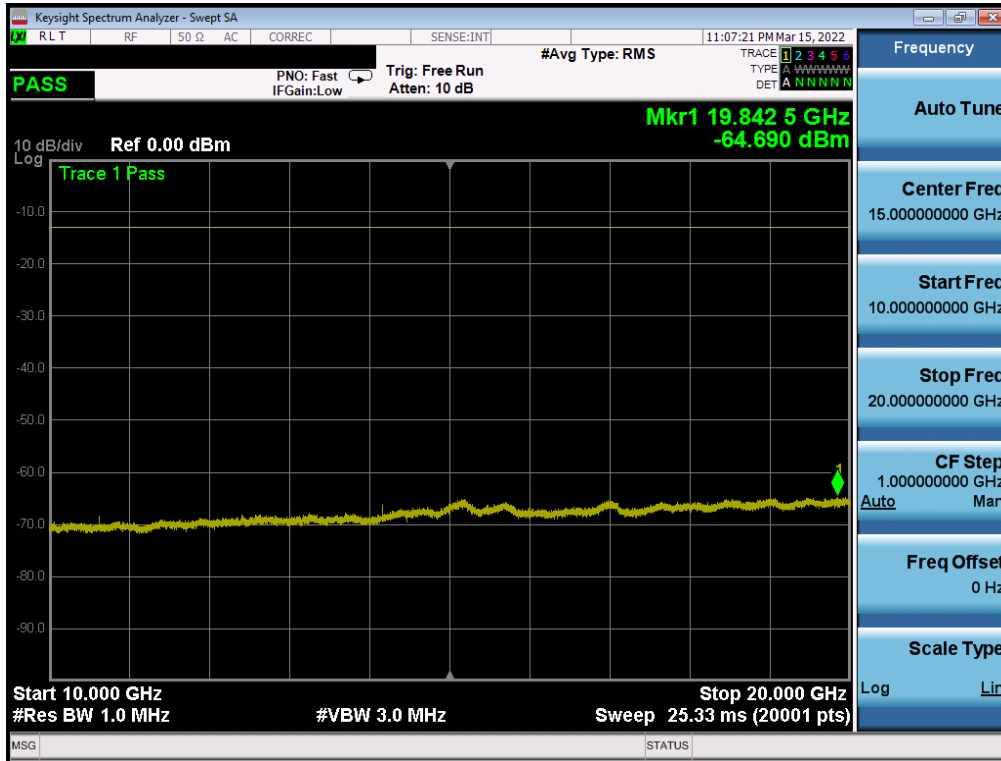
Plot 7-119. Conducted Spurious Plot (LTE Band 66/4 - 20MHz QPSK - 1 RB - High Channel – Ant1)
