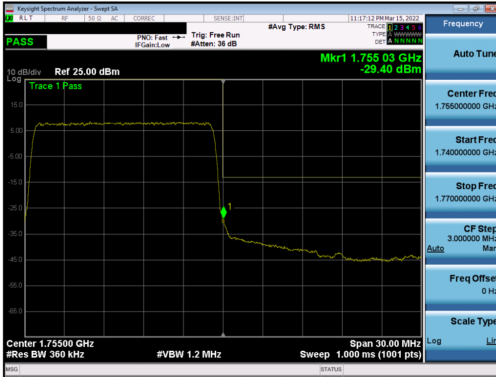
Plot 7-187. Upper Band Edge Plot (LTE Band 4 - 15MHz QPSK – Full RB - Ant1)
