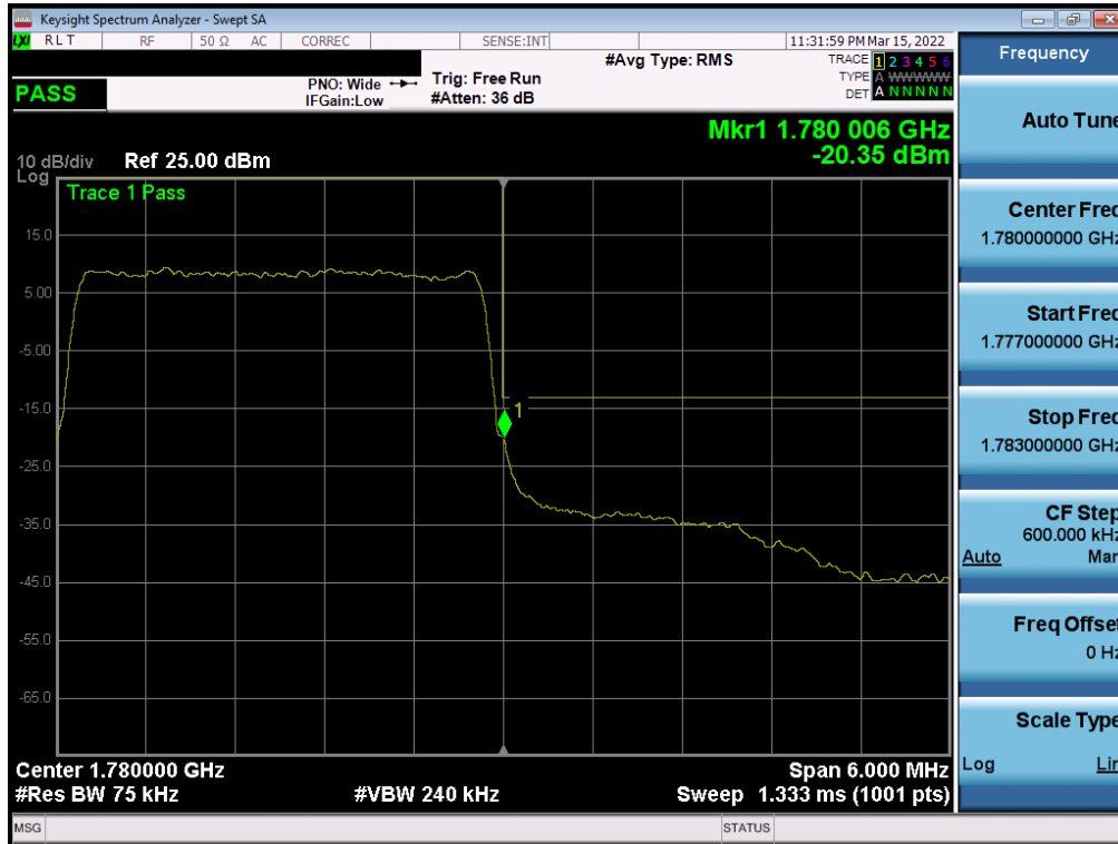
Plot 7-207. Upper Band Edge Plot (LTE Band 66 - 3MHz QPSK – Full RB - Ant1)
