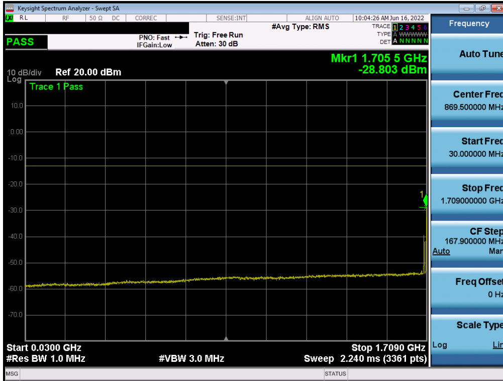
Plot 7-129. Conducted Spurious Plot (ULCA LTE Band 66 Low Channel - Ant1)
