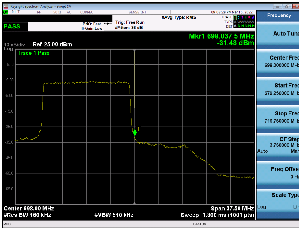
Plot 7-150. Upper Band Edge Plot (LTE Band 71 - 15MHz QPSK – Full RB - Ant1)
