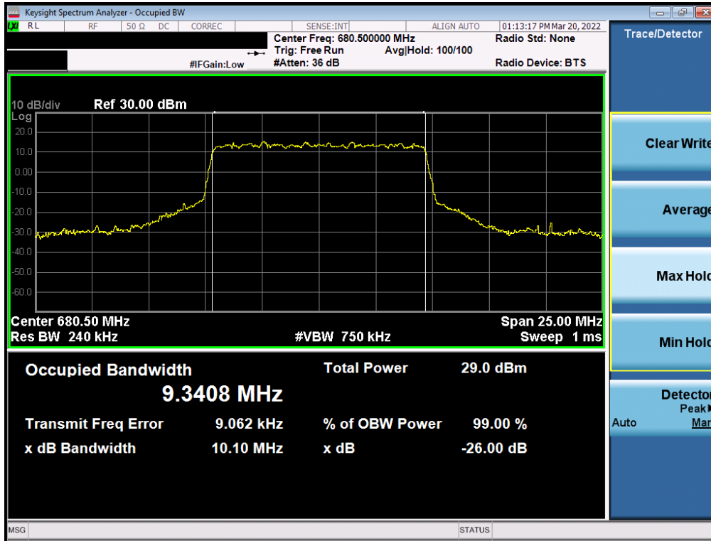
Plot 7-29. Occupied Bandwidth Plot (NR Band n71 - 10MHz CP-OFDM 16-QAM - Full RB - Ant1)
