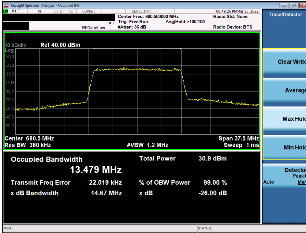
Plot 7-3. Occupied Bandwidth Plot (LTE Band 71 - 15MHz QPSK - Full RB – Ant1)
