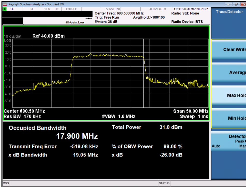
Plot 7-21. Occupied Bandwidth Plot (NR Band n71 - 20MHz DFT-s-OFDM BPSK - Full RB – Ant1)
