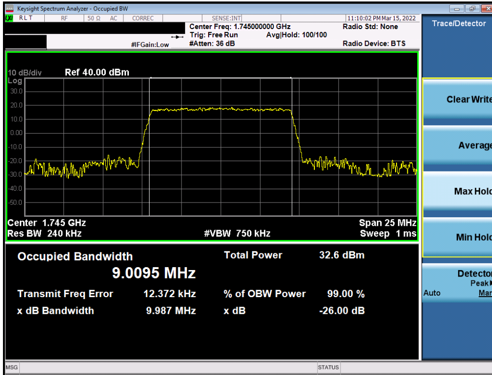
Plot 7-37. Occupied Bandwidth Plot (LTE Band 66/4 - 10MHz QPSK - Full RB - Ant1)
