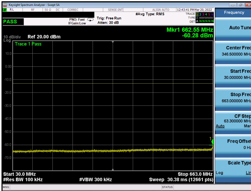
Plot 7-102. Conducted Spurious Plot (NR Band n71 -20.0MHz - 1 RB - Low Channel - Ant1)
