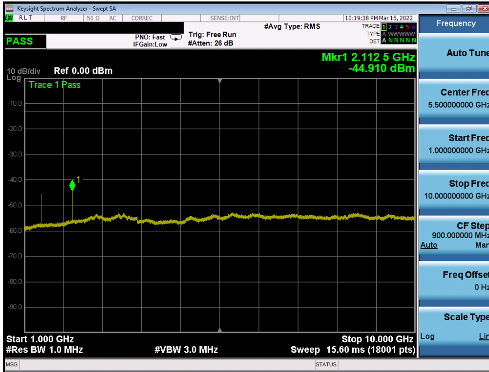
Plot 7-92. Conducted Spurious Plot (LTE Band 12 - 10MHz QPSK - 1 RB - Low Channel - Ant1)
