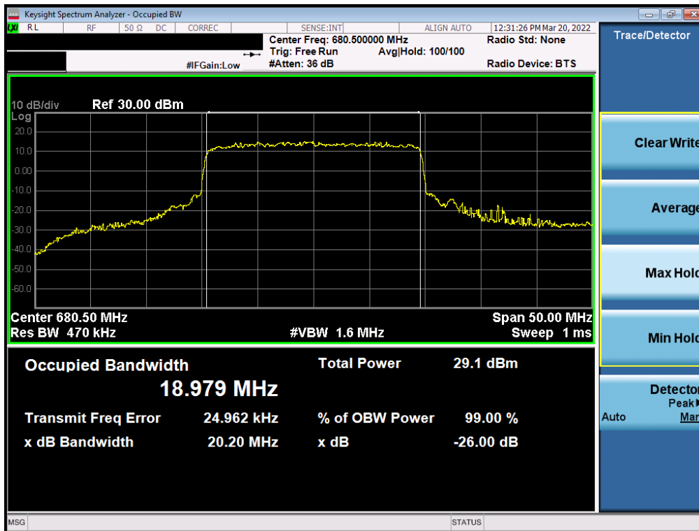
Plot 7-22. Occupied Bandwidth Plot (NR Band n71 - 20MHz CP-OFDM QPSK - Full RB – Ant1)
