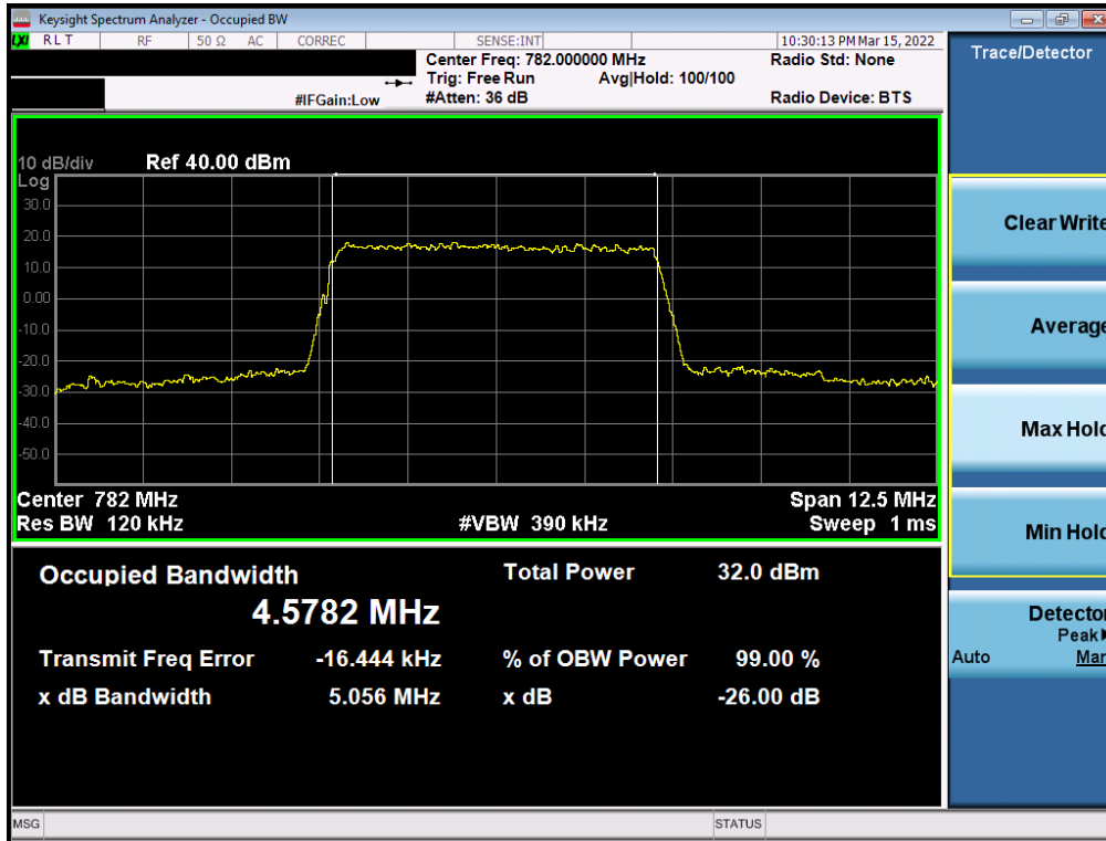
Plot 7-19. Occupied Bandwidth Plot (LTE Band 13 - 5MHz QPSK - Full RB – Ant1)
