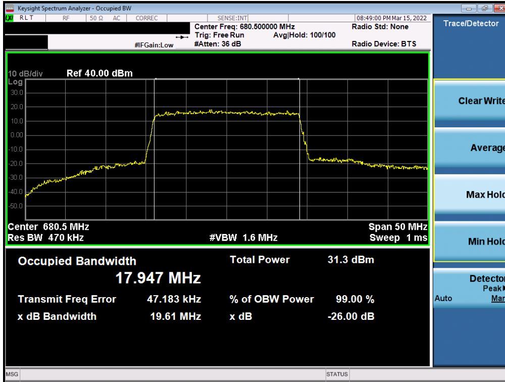
Plot 7-1. Occupied Bandwidth Plot (LTE Band 71 - 20MHz QPSK - Full RB – Ant1)
