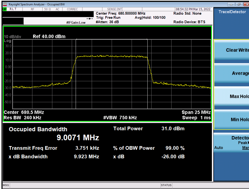
Plot 7-5. Occupied Bandwidth Plot (LTE Band 71 - 10MHz QPSK - Full RB – Ant1)
