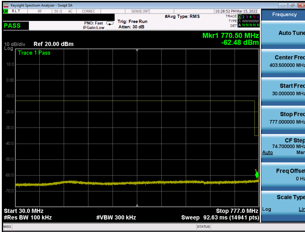
Plot 7-99. Conducted Spurious Plot (LTE Band 13 - 10MHz QPSK - 1 RB)
