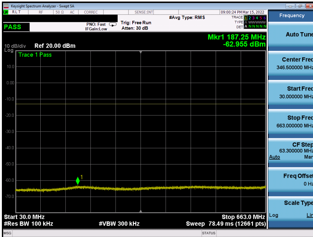
Plot 7-84. Conducted Spurious Plot (LTE Band 71 - 20MHz QPSK - 1 RB - Mid Channel - Ant1)
