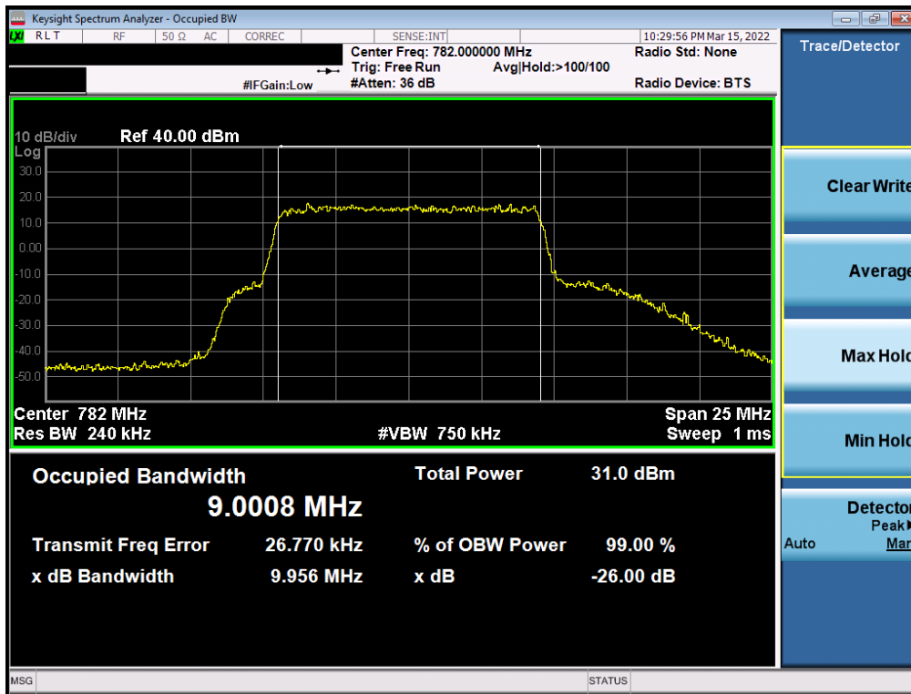
Plot 7-18. Occupied Bandwidth Plot (LTE Band 13 - 10MHz 16-QAM - Full RB – Ant1)
