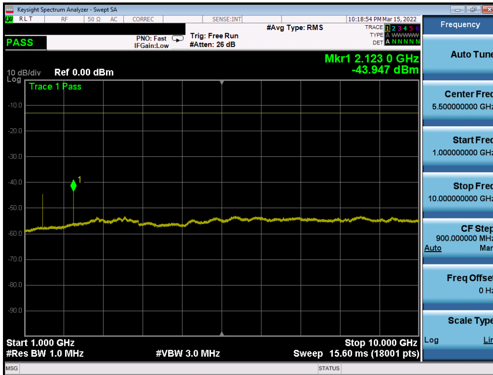
Plot 7-95. Conducted Spurious Plot (LTE Band 12 - 10MHz QPSK - 1 RB - Mid Channel - Ant1)
