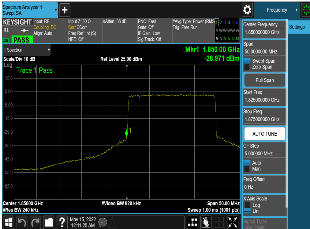
Plot 7-176. Lower Band Edge Plot (NR Band n25/2 - 20MHz QPSK – Full RB - Ant4)
