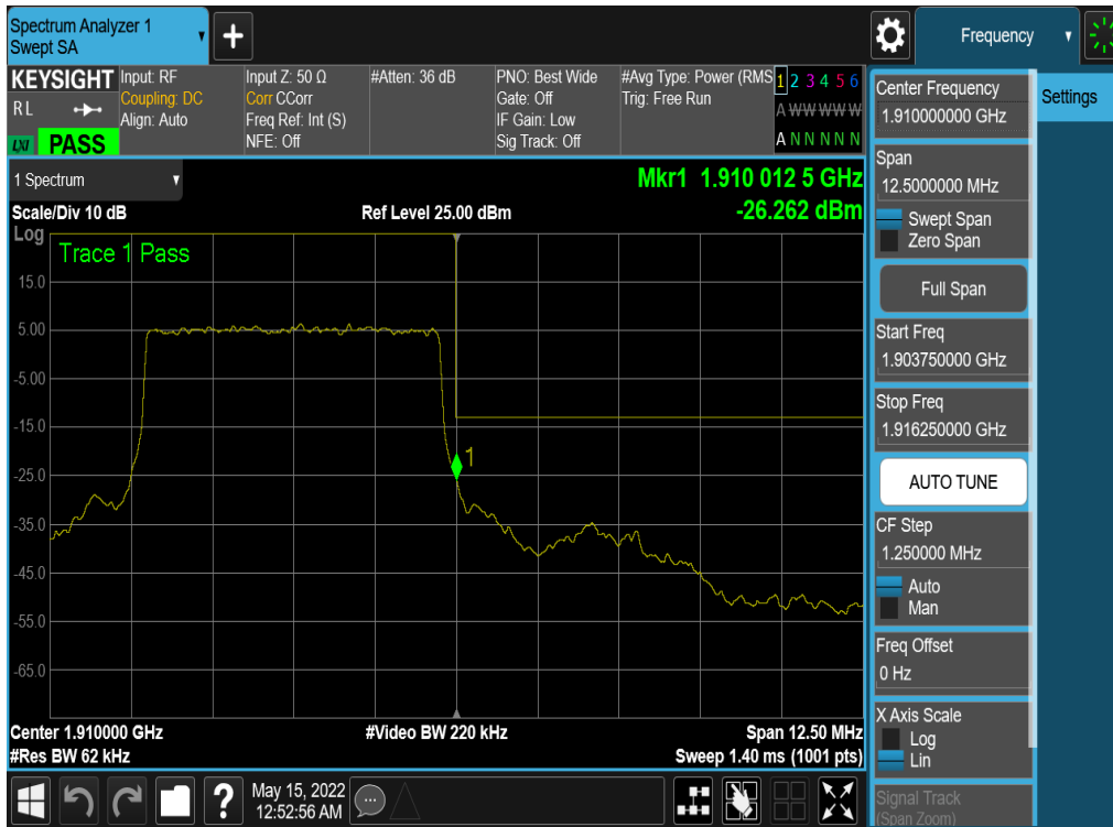
Plot 7-196. Upper Band Edge Plot (NR Band n2 – 5MHz QPSK – Full RB - Ant4)
