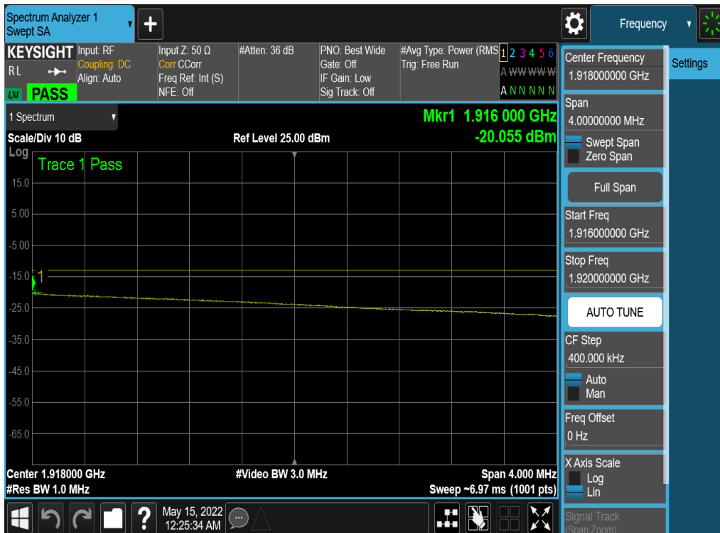
Plot 7-181. Extended Upper Band Edge Plot (NR Band n25 - 20MHz QPSK – Full RB - Ant4)
