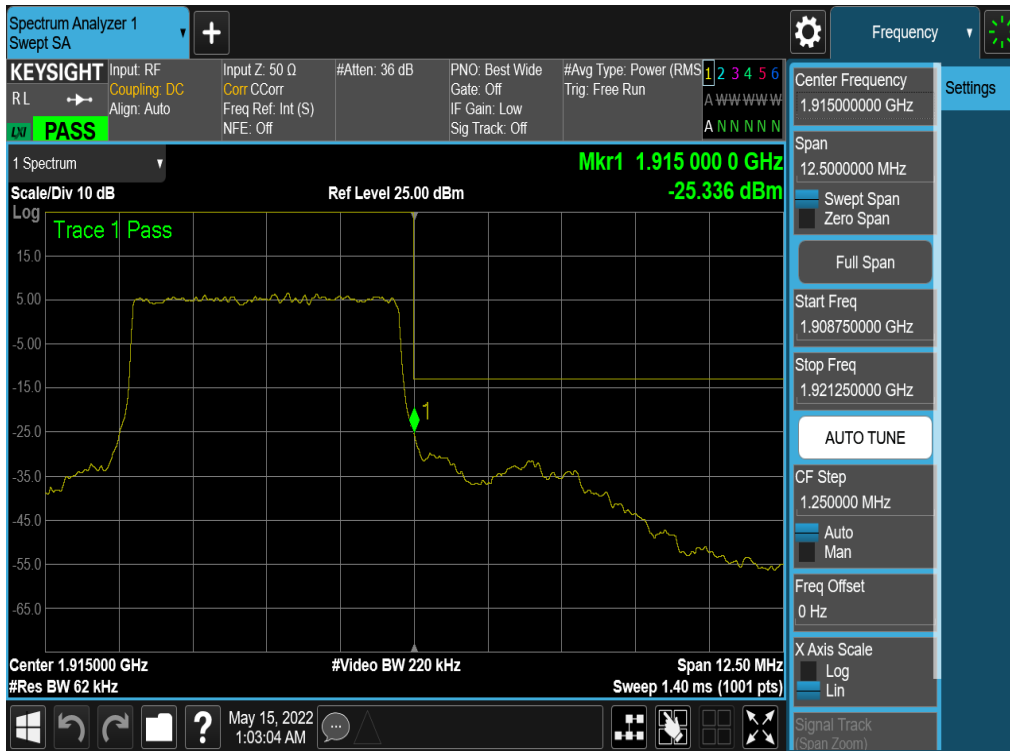
Plot 7-198. Upper Band Edge Plot (NR Band n25 – 5MHz QPSK – Full RB - Ant4)
