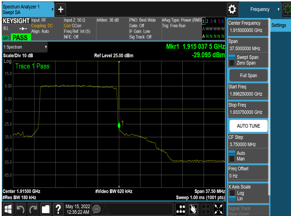
Plot 7-186. Upper Band Edge Plot (NR Band n25 - 15MHz QPSK – Full RB - Ant4)
