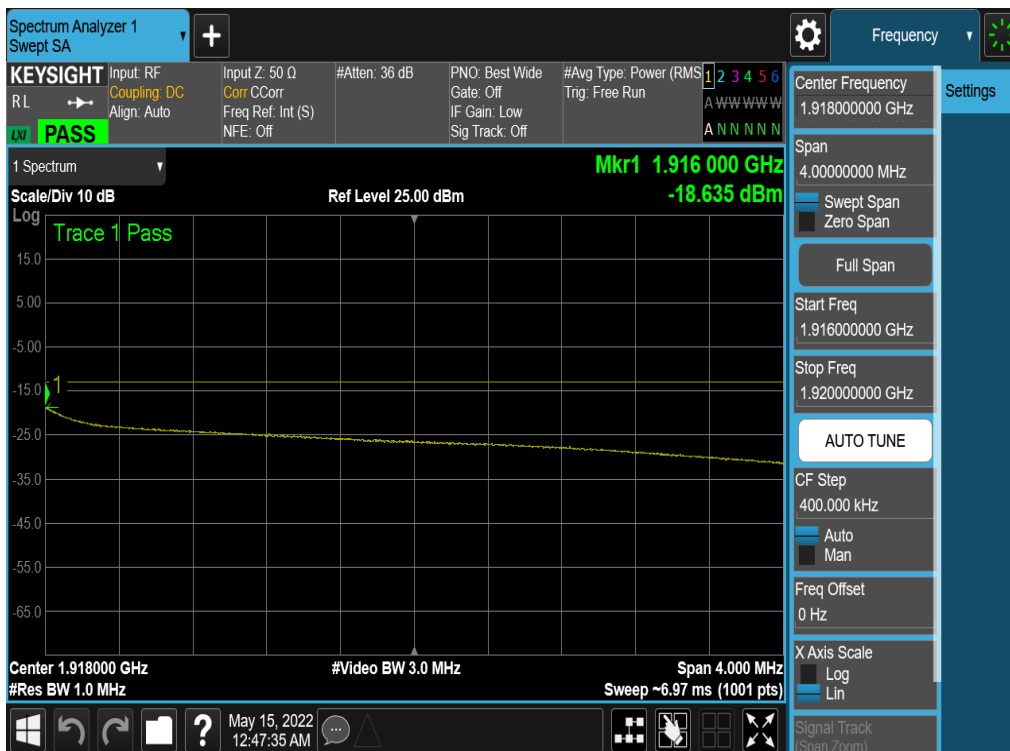
Plot 7-193. Extended Upper Band Edge Plot (NR Band n25 - 10MHz QPSK – Full RB - Ant4)
