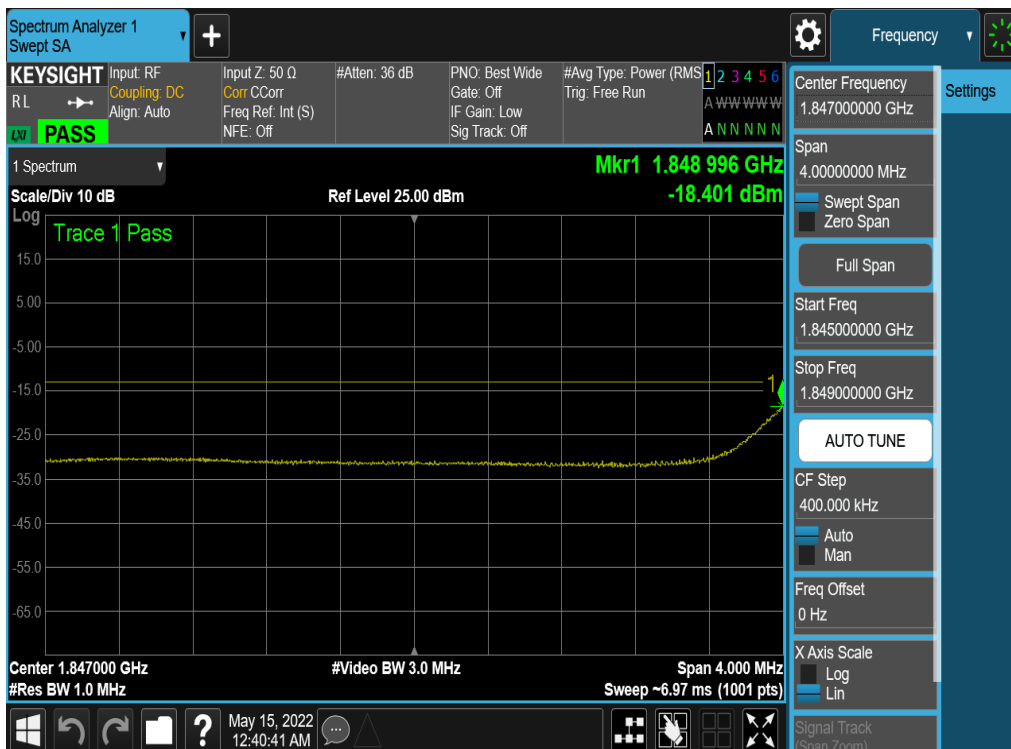
Plot 7-189. Extended Lower Band Edge Plot (NR Band n25/2 - 10MHz QPSK – Full RB - Ant4)
