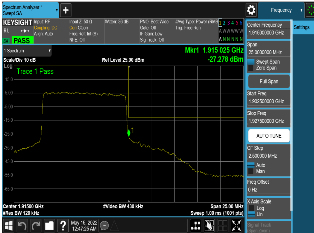
Plot 7-192. Upper Band Edge Plot (NR Band n25 - 10MHz QPSK – Full RB - Ant4)
