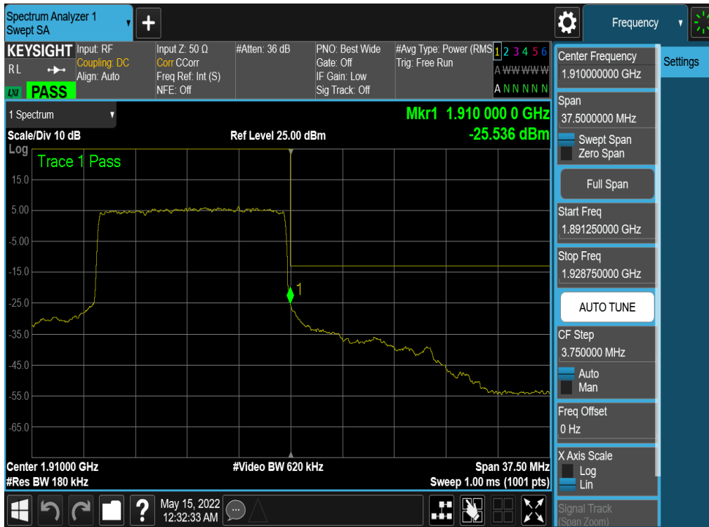
Plot 7-184. Upper Band Edge Plot (NR Band n2 - 15MHz QPSK – Full RB - Ant4)
