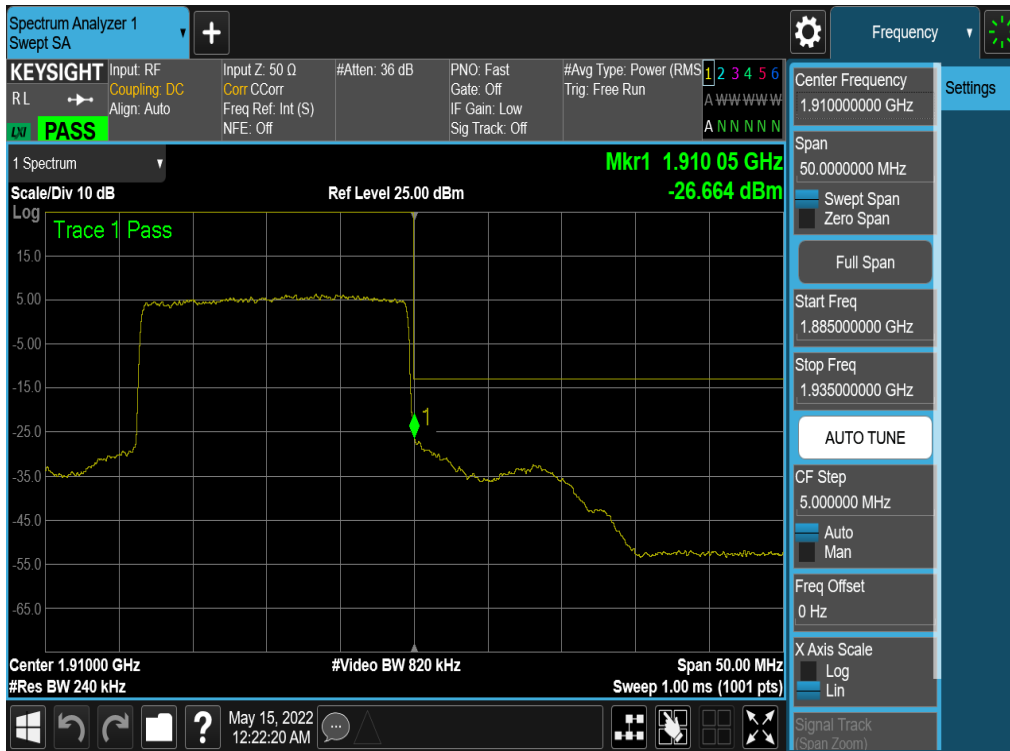
Plot 7-178. Upper Band Edge Plot (NR Band n2 - 20MHz QPSK – Full RB - Ant4)
