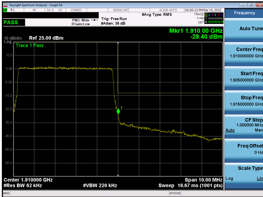
Plot 7-112. Upper Band Edge Plot (LTE Band 2 - 5MHz QPSK – Full RB - Ant1)
