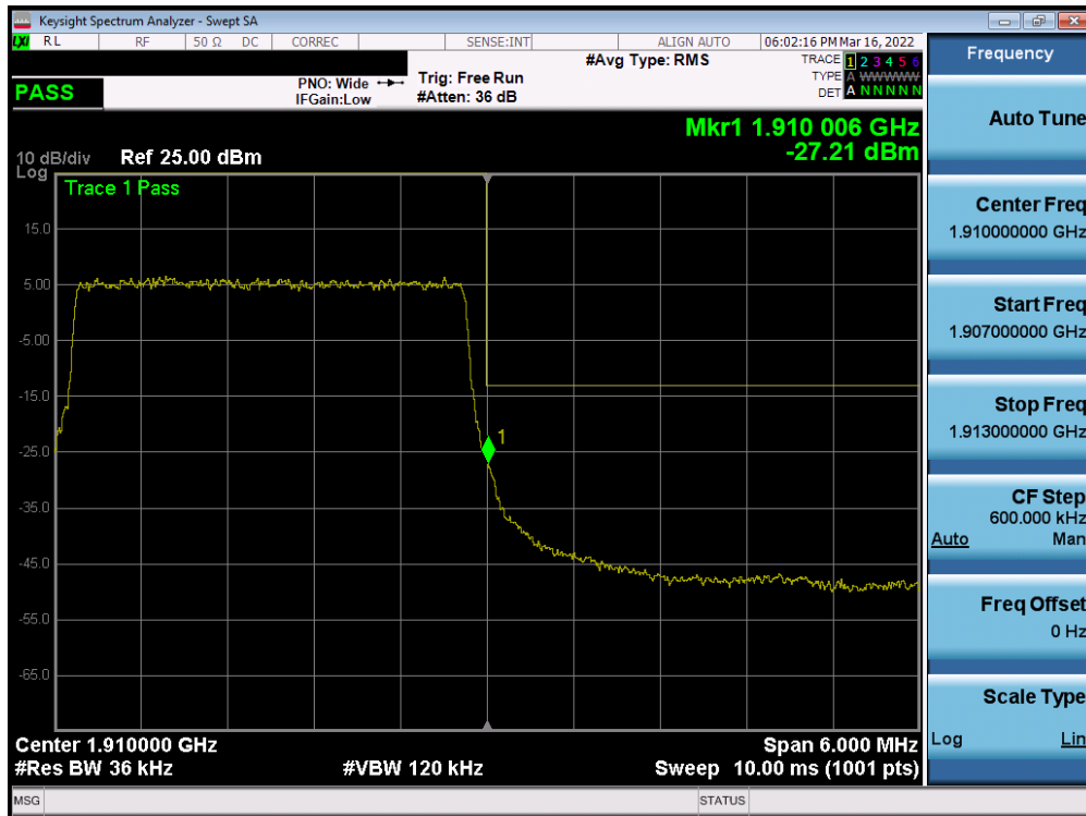
Plot 7-118. Upper Band Edge Plot (LTE Band 2 - 3MHz QPSK – Full RB - Ant1)
