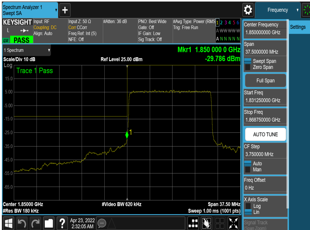
Plot 7-146. Lower Band Edge Plot (NR Band n25/2 - 15MHz QPSK – Full RB - Ant1)
