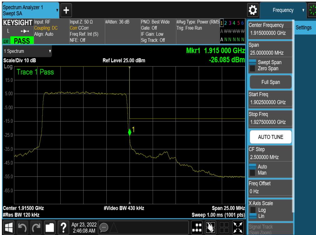
Plot 7-156. Upper Band Edge Plot (NR Band n25 - 10MHz QPSK – Full RB - Ant1)
