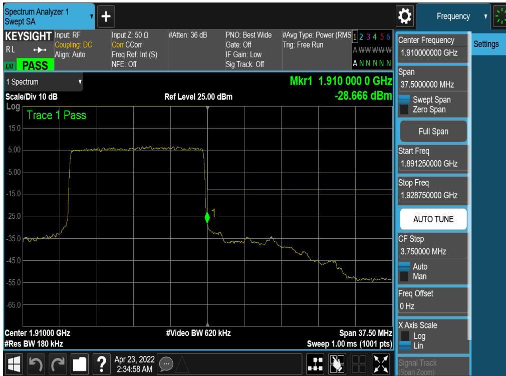
Plot 7-148. Upper Band Edge Plot (NR Band n2 - 15MHz QPSK – Full RB - Ant1)
