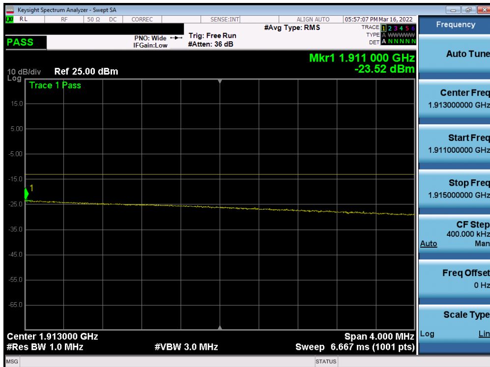
Plot 7-101. Extended Upper Band Edge Plot (LTE Band 2 - 15MHz QPSK – Full RB - Ant1)
