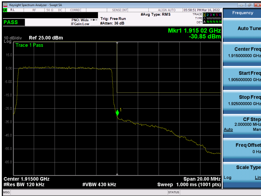
Plot 7-108. Upper Band Edge Plot (LTE Band 25 - 10MHz QPSK – Full RB - Ant1)
