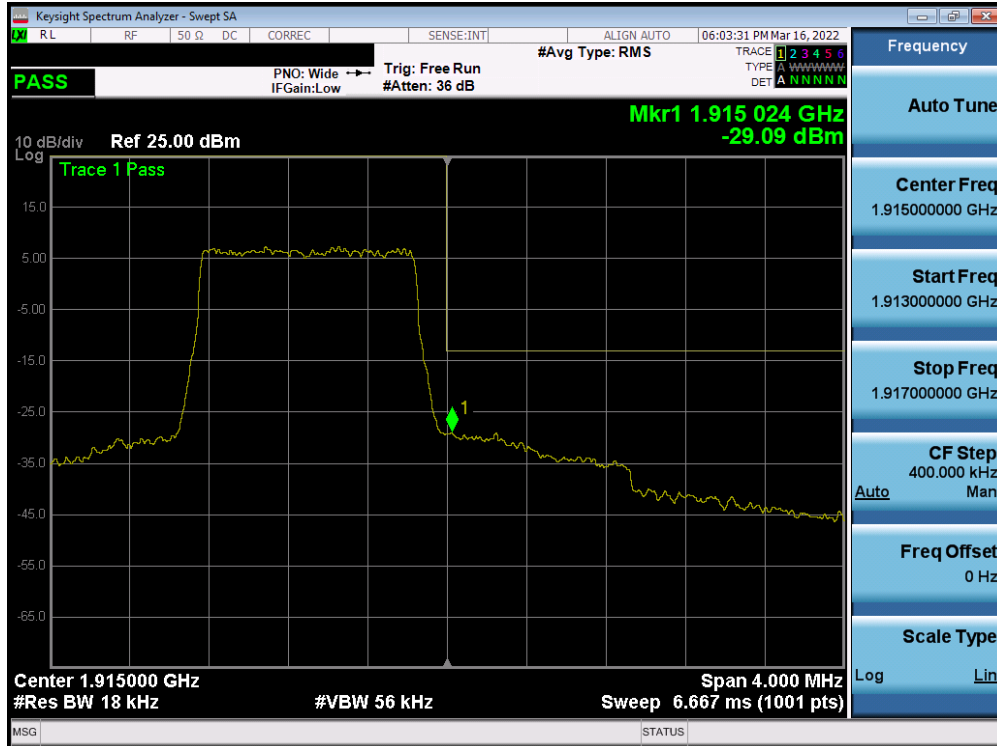
Plot 7-126. Upper Band Edge Plot (LTE Band 25 – 1.4MHz QPSK – Full RB - Ant1)
