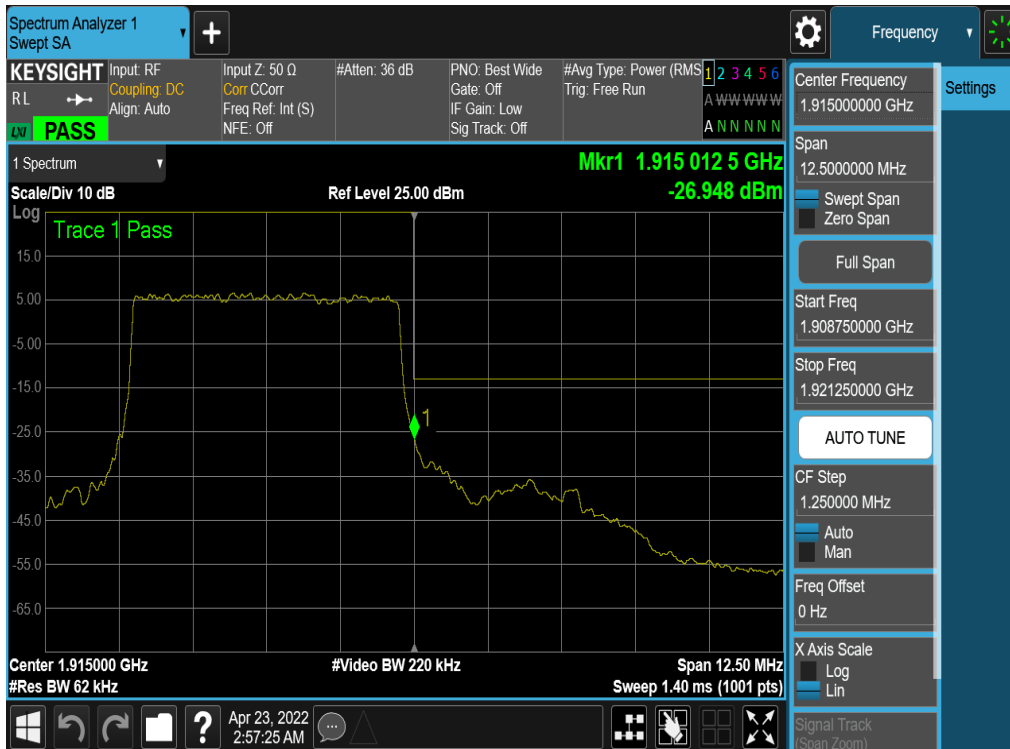
Plot 7-162. Upper Band Edge Plot (NR Band n25 – 5MHz QPSK – Full RB - Ant1)
