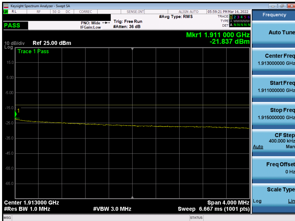
Plot 7-107. Extended Upper Band Edge Plot (LTE Band 2 - 10MHz QPSK – Full RB - Ant1)
