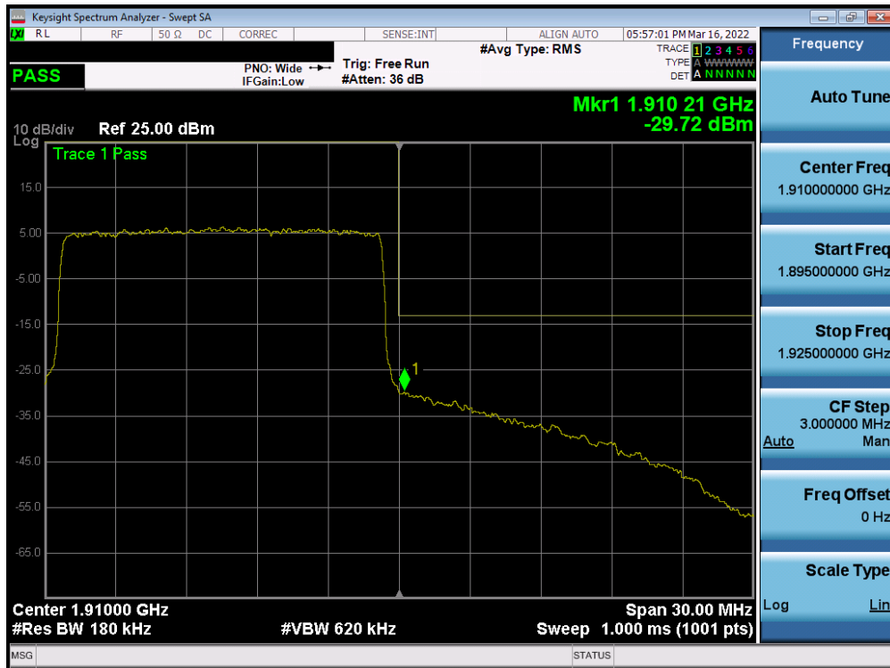
Plot 7-100. Upper Band Edge Plot (LTE Band 2 - 15MHz QPSK – Full RB - Ant1)
