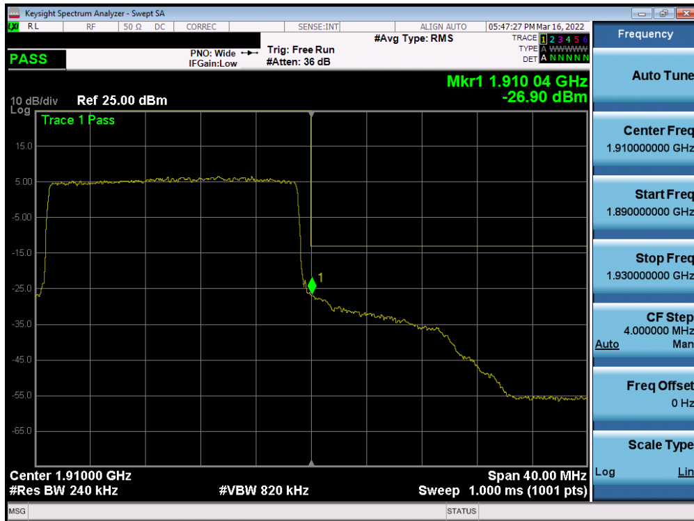
Plot 7-94. Upper Band Edge Plot (LTE Band 2 - 20MHz QPSK – Full RB - Ant1)
