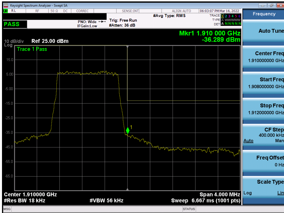
Plot 7-124. Upper Band Edge Plot (LTE Band 2 – 1.4MHz QPSK – Full RB - Ant1)
