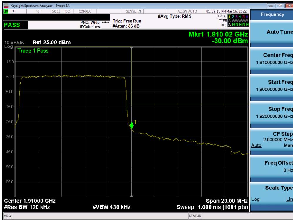
Plot 7-106. Upper Band Edge Plot (LTE Band 2 - 10MHz QPSK – Full RB - Ant1)
