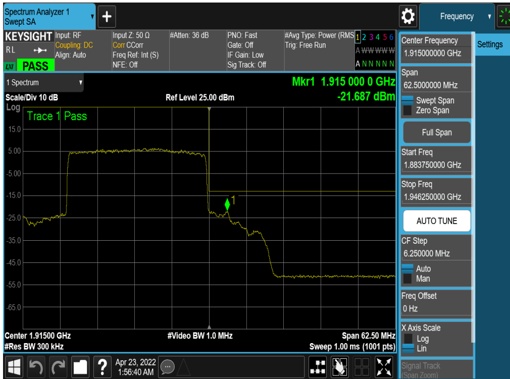
Plot 7-134. Upper Band Edge Plot (NR Band n25 - 30MHz QPSK – Full RB - Ant1)
