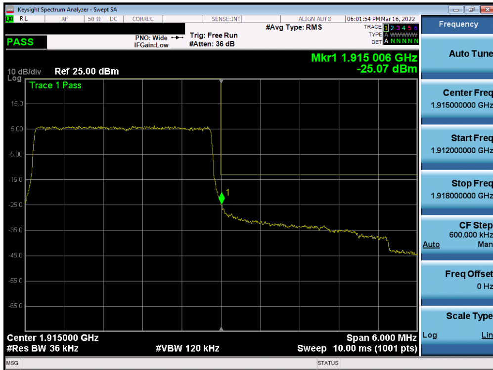
Plot 7-120. Upper Band Edge Plot (LTE Band 25 - 3MHz QPSK – Full RB - Ant1)
