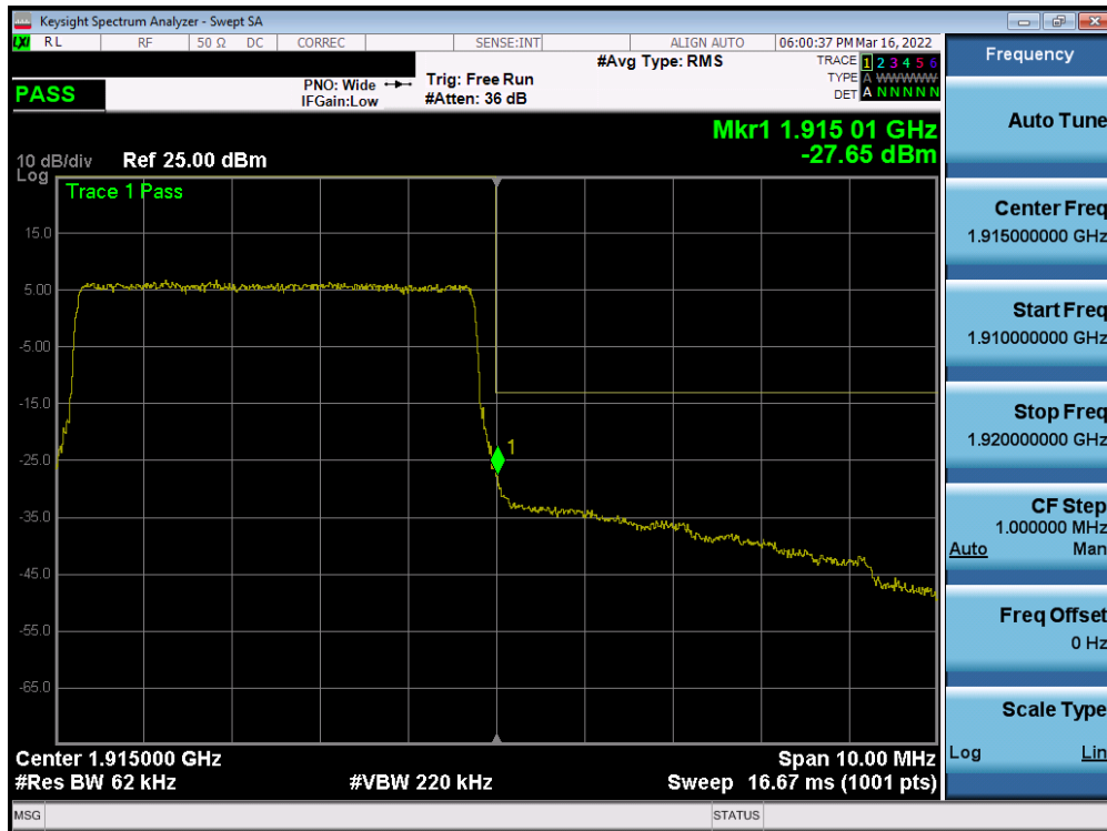
Plot 7-114. Upper Band Edge Plot (LTE Band 25 - 5MHz QPSK – Full RB - Ant1)
