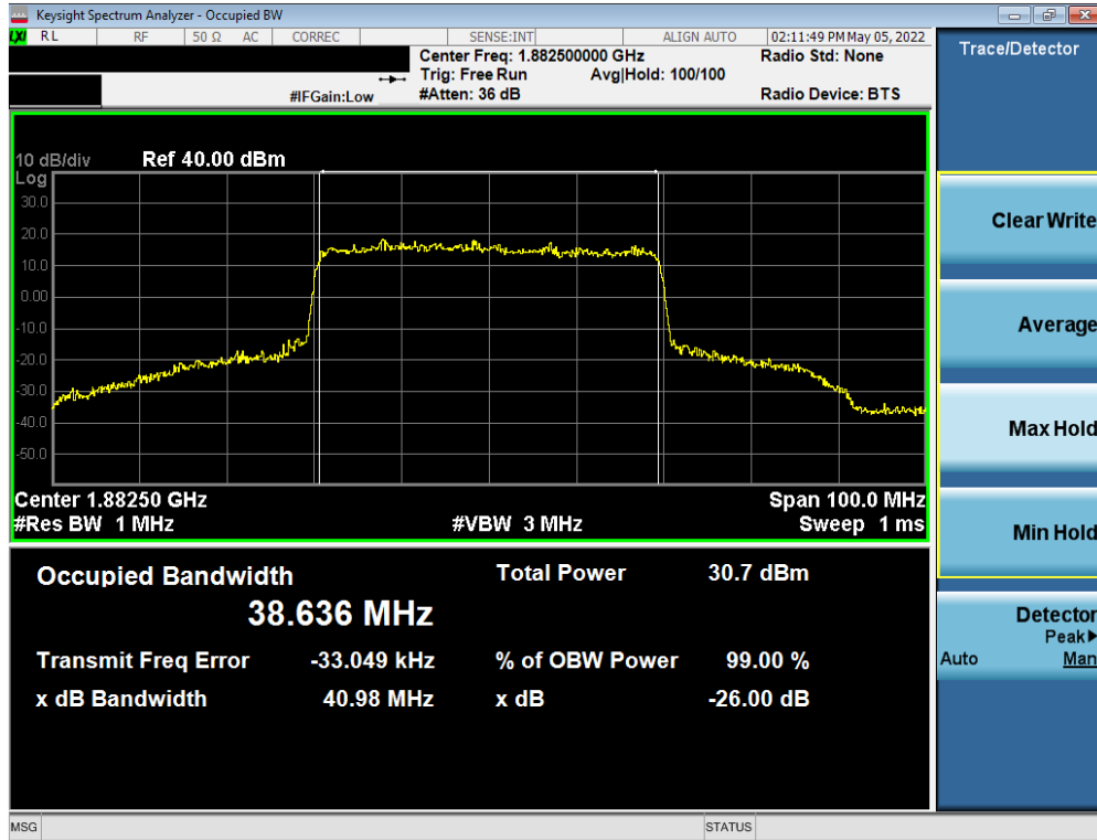
Plot 7-36. Occupied Bandwidth Plot (NR Band n25 - 40.0MHz CP-OFDM 16QAM - Full RB - ANT4)
