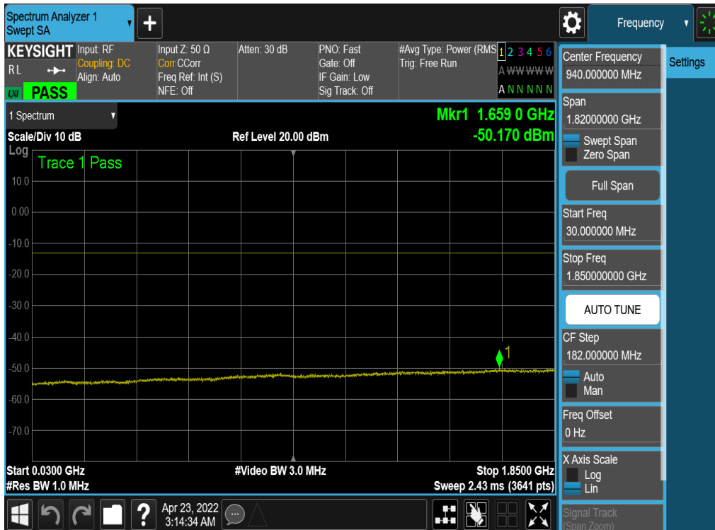
Plot 7-71. Conducted Spurious Plot (NR Band n25 - 40.0MHz - 1RB - High Channel - Ant1)
