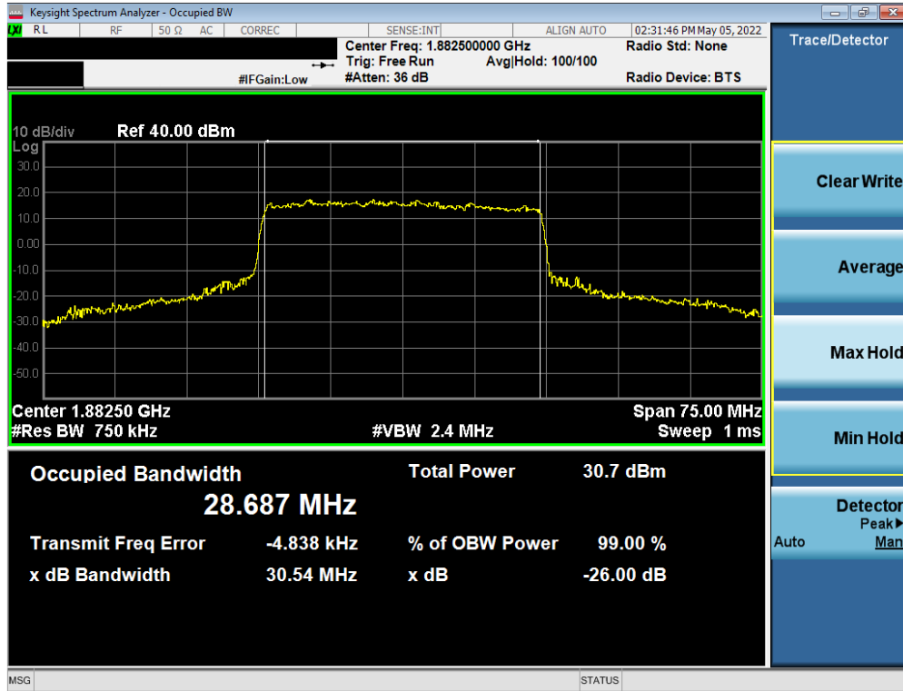
Plot 7-38. Occupied Bandwidth Plot (NR Band n25 - 30.0MHz CP-OFDM QPSK - Full RB - ANT4)
