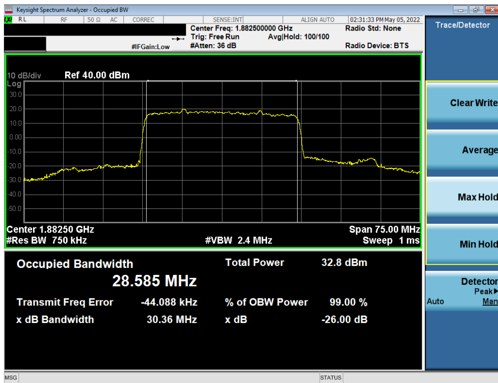
Plot 7-37. Occupied Bandwidth Plot (NR Band n25 - 30.0MHz DFT-s-OFDM BPSK - Full RB - ANT4)
