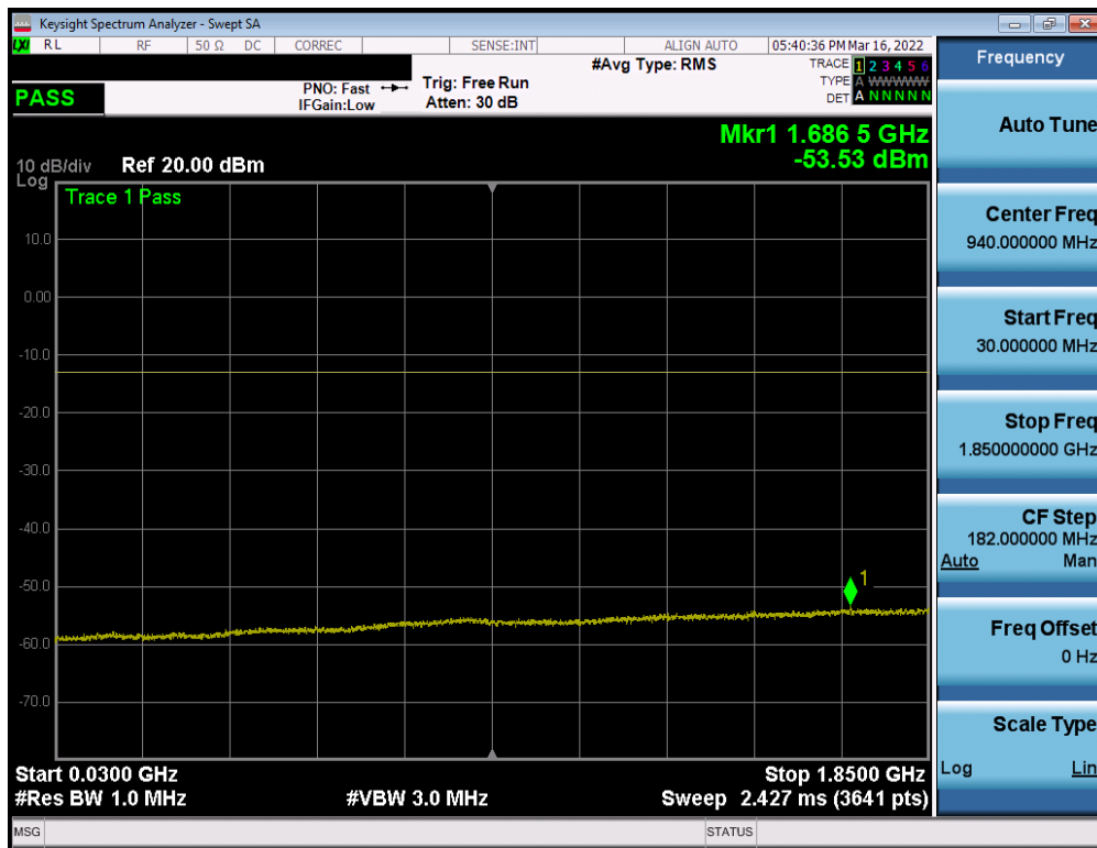
Plot 7-59. Conducted Spurious Plot (LTE Band 25/2 - 20MHz QPSK - 1RB - Mid Channel - Ant1)
