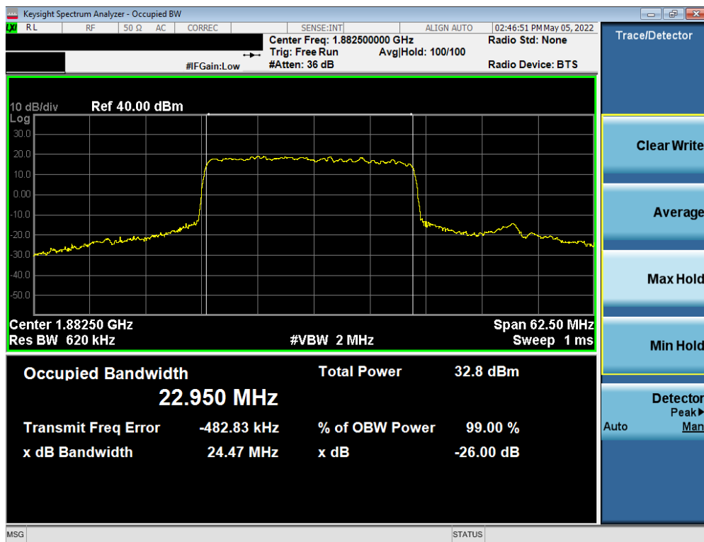
Plot 7-41. Occupied Bandwidth Plot (NR Band n25 - 25.0MHz CP-OFDM QPSK - Full RB - ANT4)
