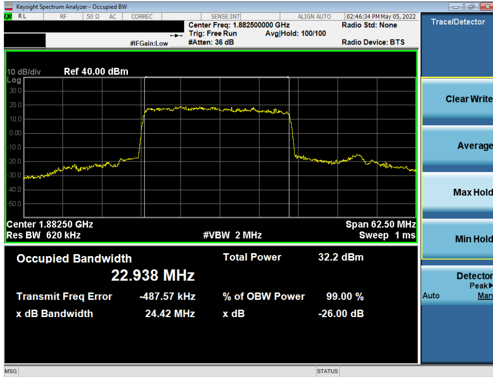
Plot 7-40. Occupied Bandwidth Plot (NR Band n25 - 25.0MHz DFT-s-OFDM BPSK - Full RB - ANT4)
