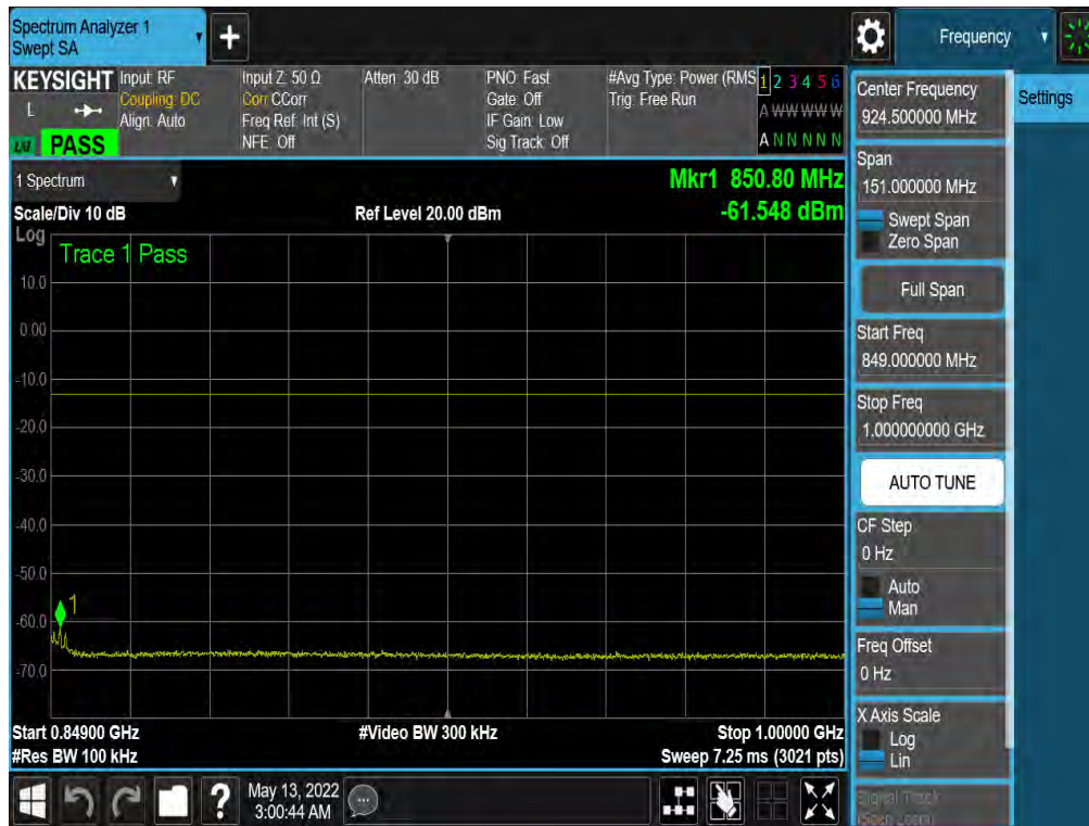
Plot 7-34. Conducted Spurious Plot (ULCA LTE Band 5 – 10+10MHz QPSK – PCC 1/49 SCC 1/0 - Low Channel)
