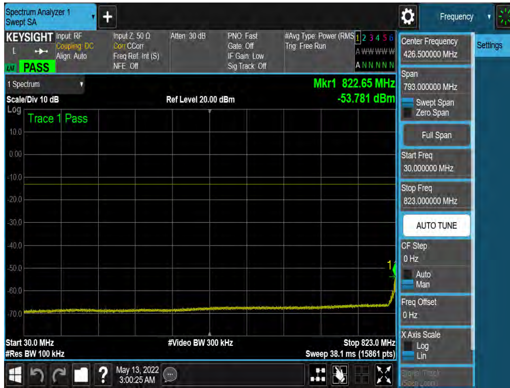
Plot 7-33. Conducted Spurious Plot (ULCA LTE Band 5 – 10+10MHz QPSK – PCC 1/49 SCC 1/0 - Low Channel)
