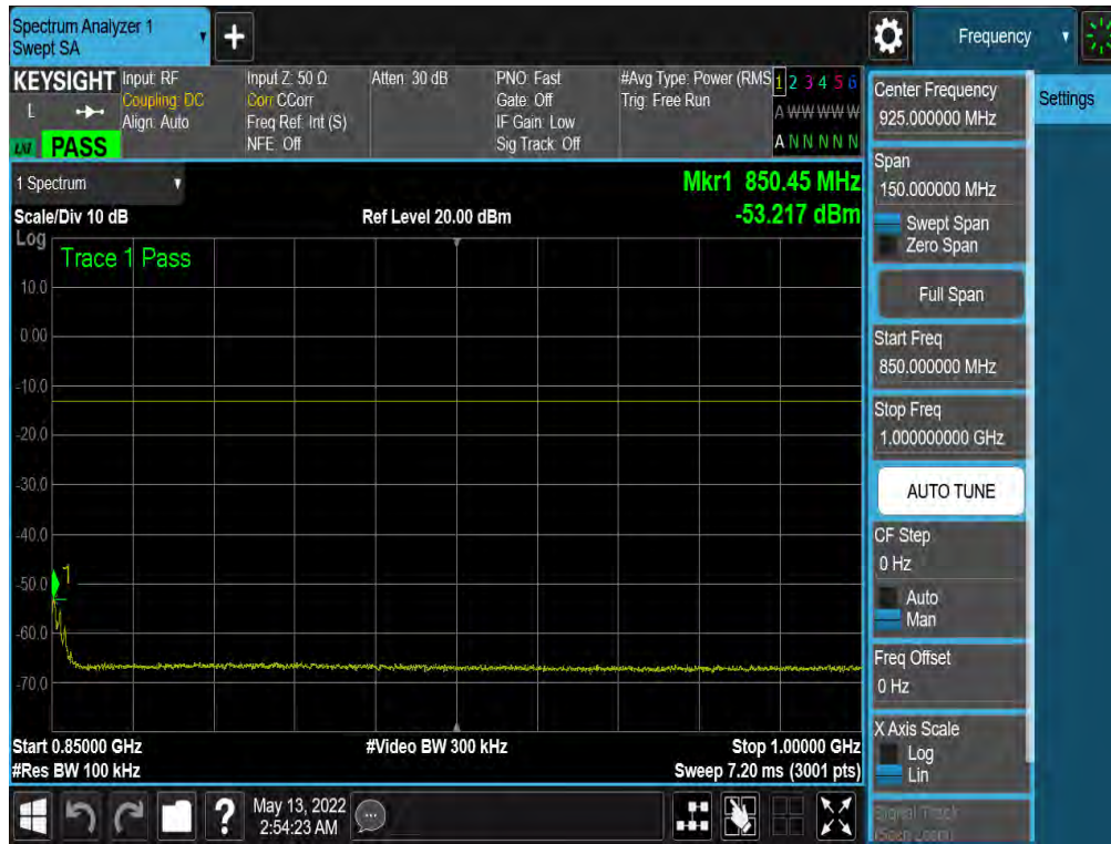
Plot 7-40. Conducted Spurious Plot (ULCA LTE Band 5 – 10+10MHz QPSK – PCC 1/0 SCC 1/49 - High Channel)
