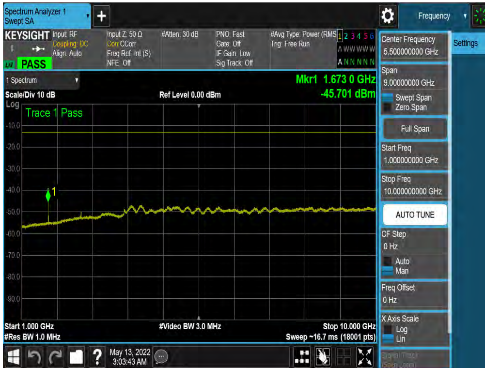
Plot 7-38. Conducted Spurious Plot (ULCA LTE Band 5 – 10+10MHz QPSK – PCC 1/49 SCC 1/0 - Mid Channel)
