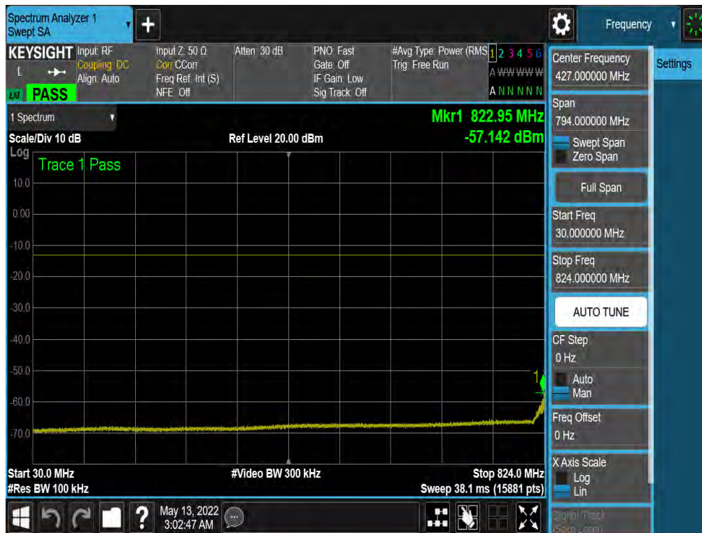
Plot 7-36. Conducted Spurious Plot (ULCA LTE Band 5 – 10+10MHz QPSK – PCC 1/49 SCC 1/0 - Mid Channel)
