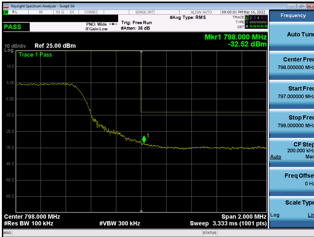
Plot 7-28. Upper Band Edge Plot (LTE Band 14, 10MHz QPSK - RB Size 50)
