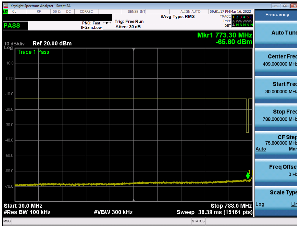
Plot 7-18. Conducted Spurious Plot (LTE Band 14 - 10MHz QPSK - RB Size 1, RB Offset 0)
