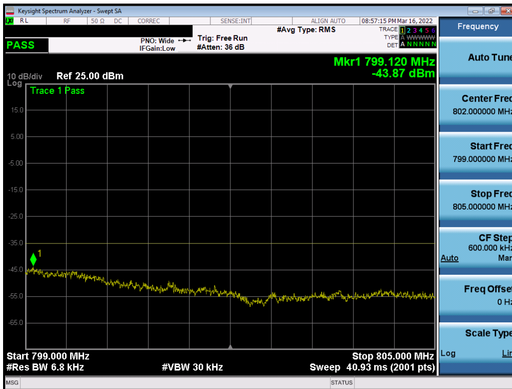
Plot 7-33. Upper Emission Mask Plot (LTE Band 14, 5MHz QPSK - RB Size 25)
