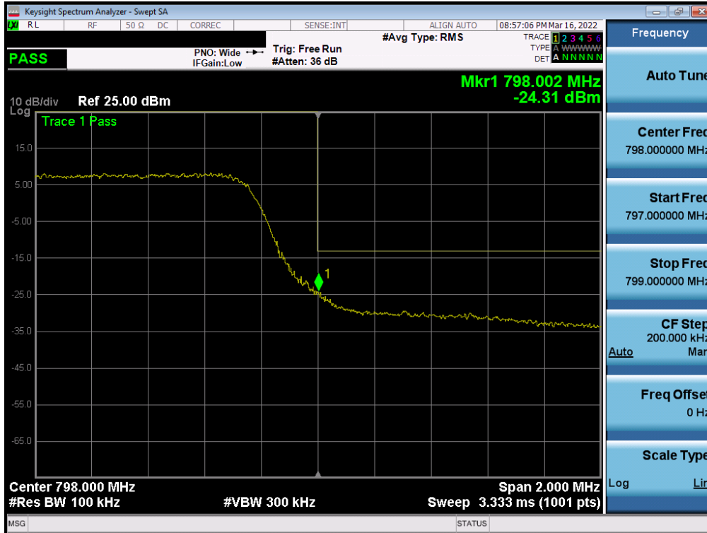
Plot 7-32. Upper Band Edge Plot (LTE Band 14, 5MHz QPSK - RB Size 25)
