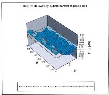
Probe isotropy for E<sub>tot</sub>: probe rotated  $\phi$  = 0° to 360°, tilted from field propagation direction  $\vec{k}$  Parallel to the field propagation ( $\psi$  =0° - 90°) at 60 GHz: deviation within ± 0.38 dB Parallel to the field propagation ( $\psi$  =0° - 90°) at 90 GHz: deviation within ± 0.36 dB
