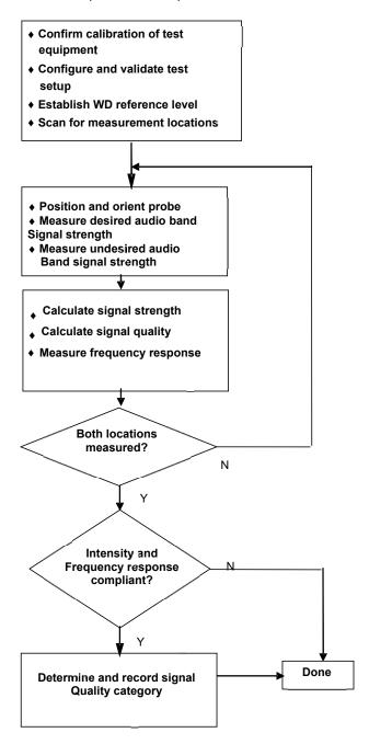
Figure 4-14 C63.19 T-Coil Signal Test Process
