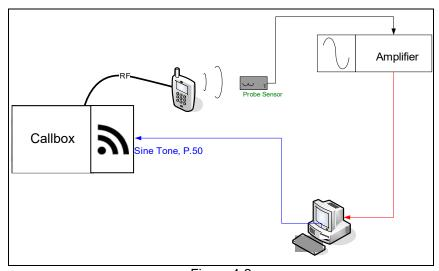
Figure 4-2 **T-Coil Test Setup**
