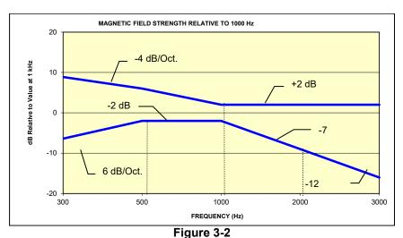
Magnetic Field frequency response for wireless devices with an axial field that exceeds
