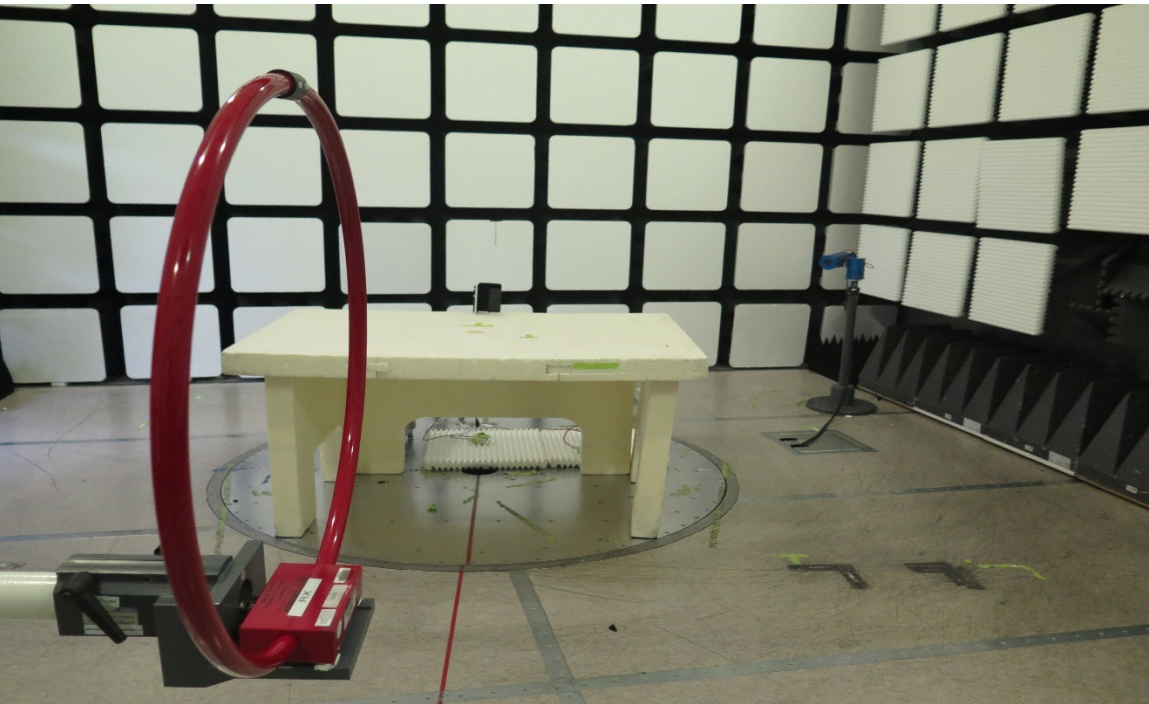
Figure 2 Radiated Spurious Emissions Test Setup (9k-30MHz) – Flat Posture – Z - Perpendicular
