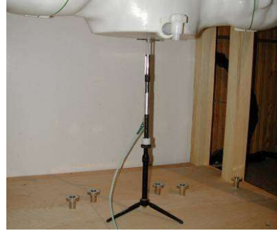
Figure 10-2 System Verification Setup Photo (> 13 MHz)
