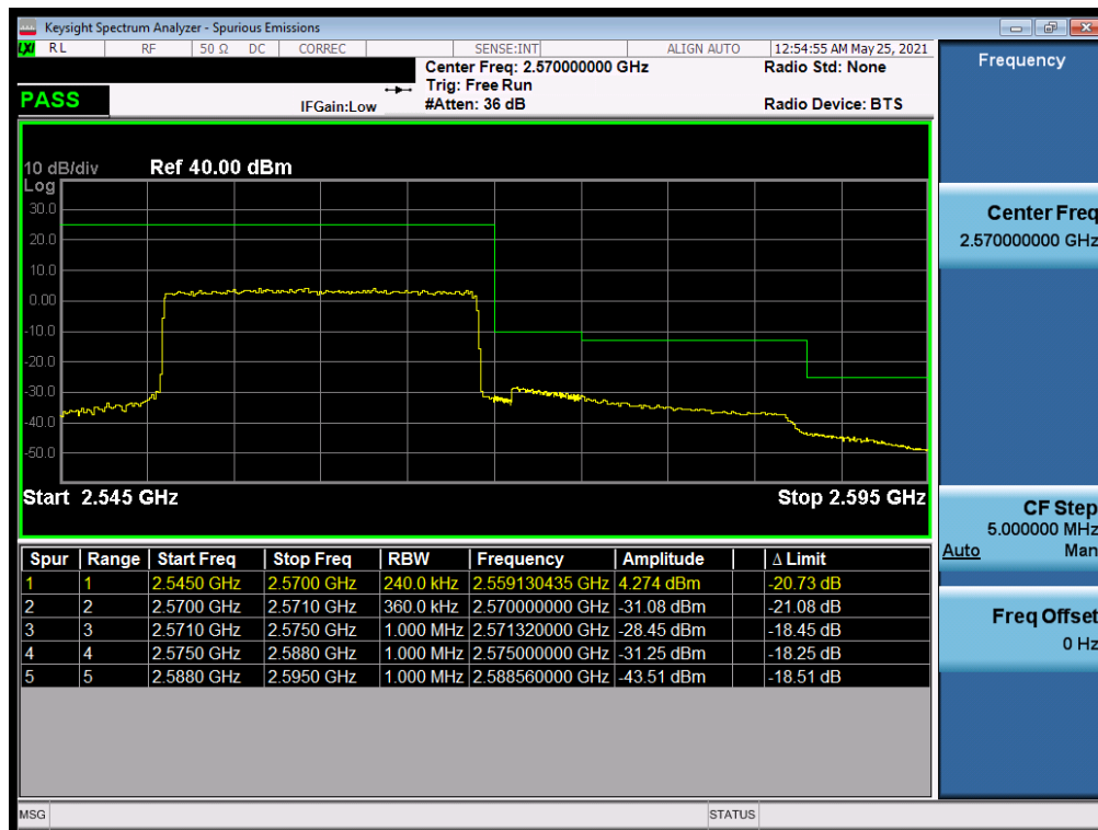
Plot 7-101. Upper ACP Plot (LTE Band 7 - 20MHz QPSK - Full RB)
