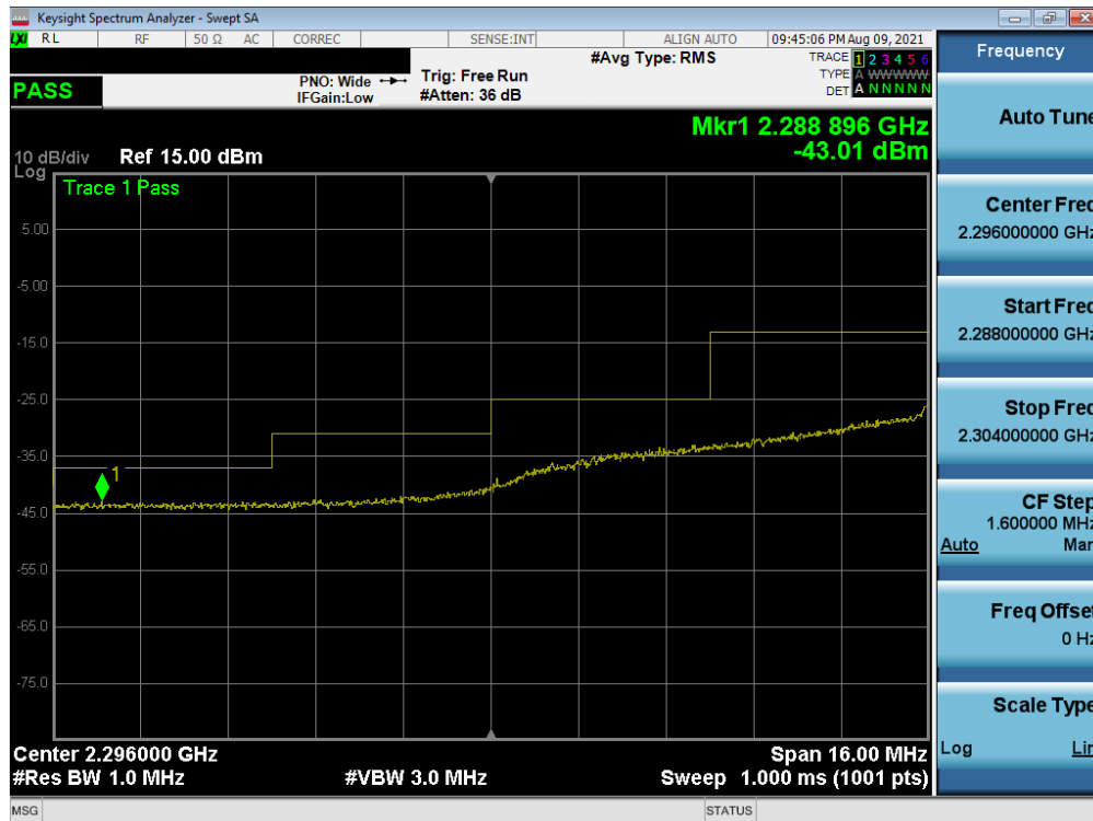
Plot 7-93. Extended Lower Band Edge Plot (LTE Band 30 - 10MHz QPSK - Full RB)
