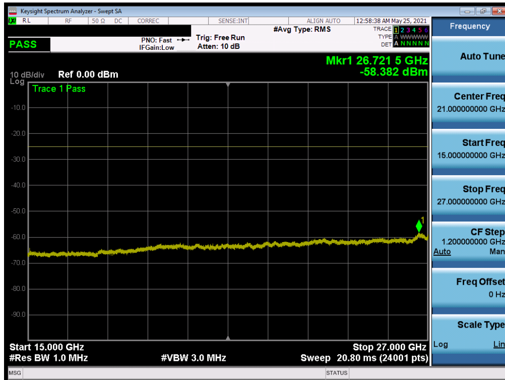
Plot 7-58. Conducted Spurious Plot (LTE Band 7 - 20MHz QPSK - RB Size 1, RB Offset 0 - Low Channel)
