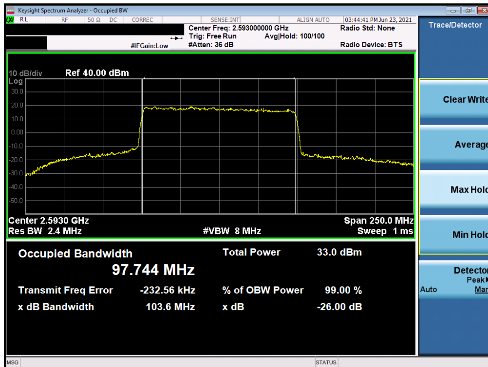
Plot 7-30. Occupied Bandwidth Plot (NR Band n41 - 100MHz QPSK - Full RB)
