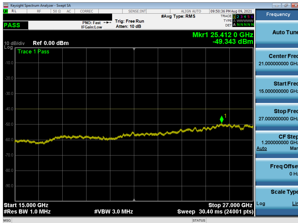
Plot 7-55. Conducted Spurious Plot (LTE Band 30 - 10MHz QPSK - RB Size 1, RB Offset 0)
