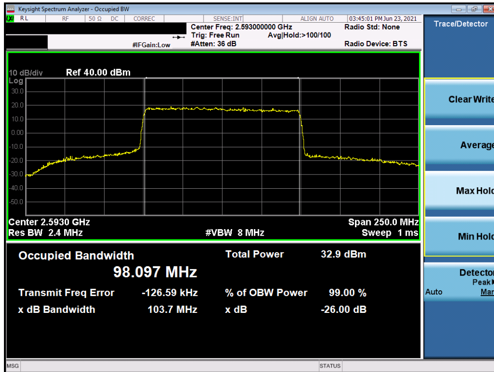
Plot 7-31. Occupied Bandwidth Plot (NR Band n41 - 100MHz 16-QAM - Full RB)
