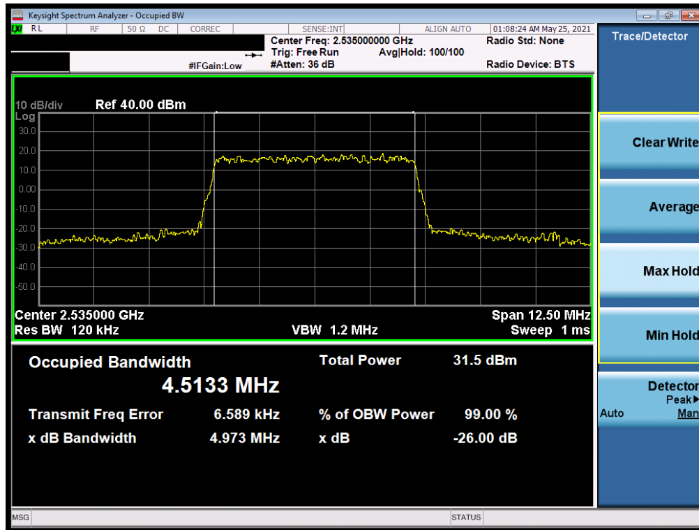
Plot 7-11. Occupied Bandwidth Plot (LTE Band 7 - 5MHz QPSK - Full RB)
