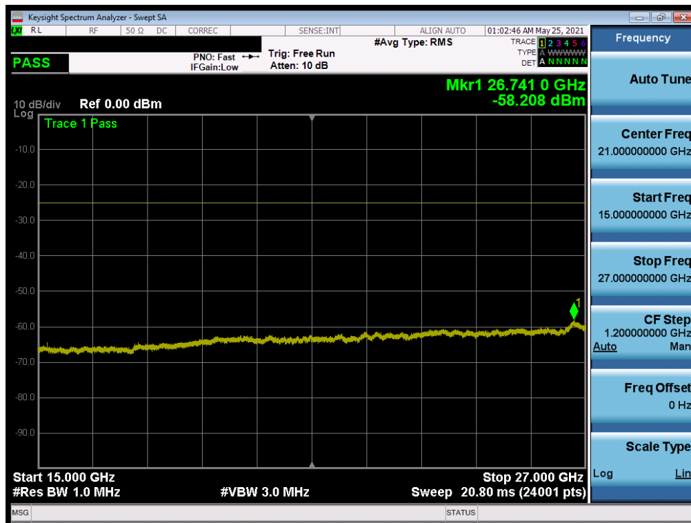
Plot 7-61. Conducted Spurious Plot (LTE Band 7 - 20MHz QPSK - RB Size 1, RB Offset 0 - Mid Channel)
