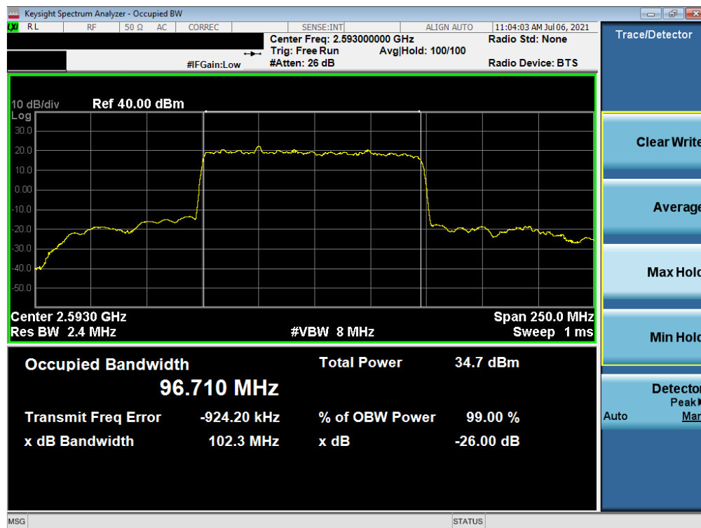
Plot 7-29. Occupied Bandwidth Plot (NR Band n41 - 100MHz \pi/2 BPSK - Full RB)
