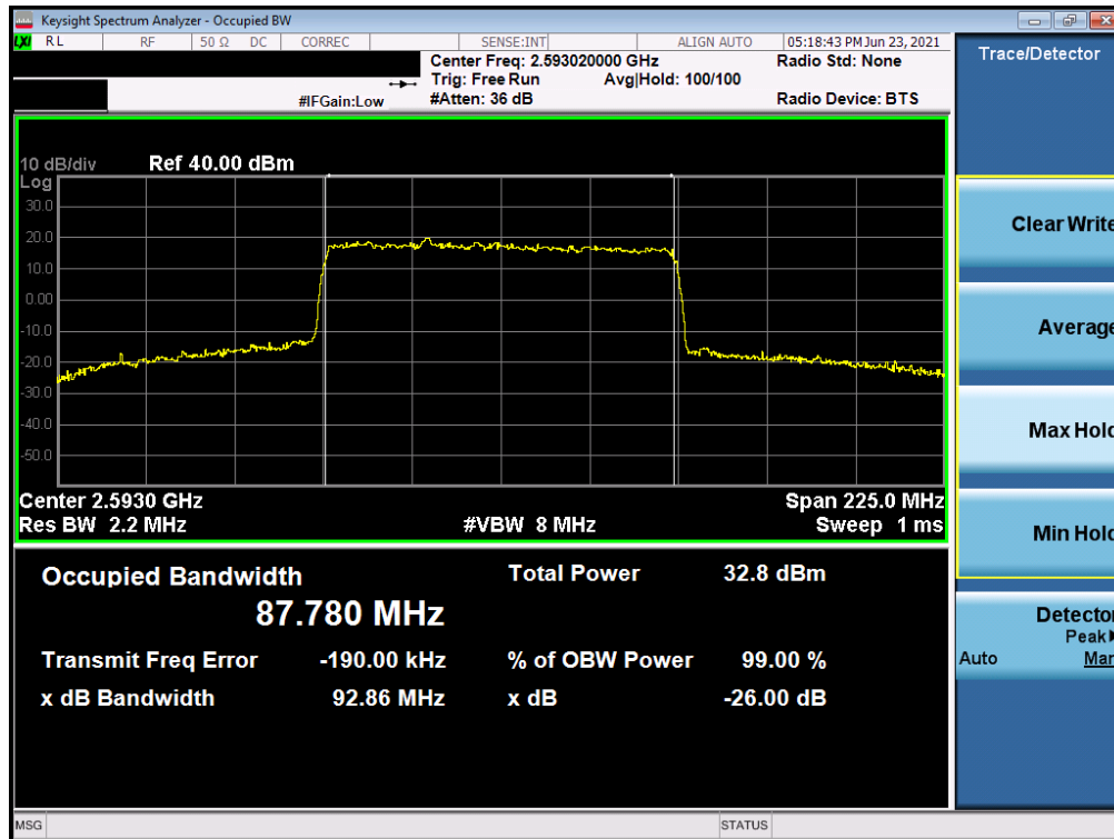
Plot 7-33. Occupied Bandwidth Plot (NR Band n41 - 90MHz QPSK - Full RB)
