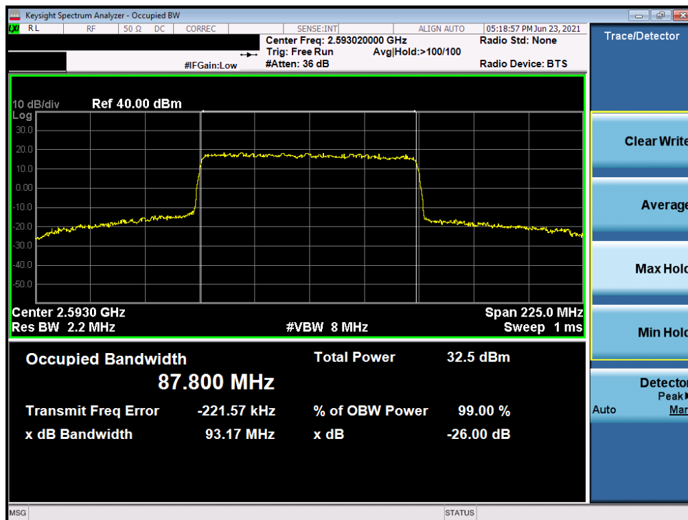
Plot 7-34. Occupied Bandwidth Plot (NR Band n41 - 90MHz 16-QAM - Full RB)
