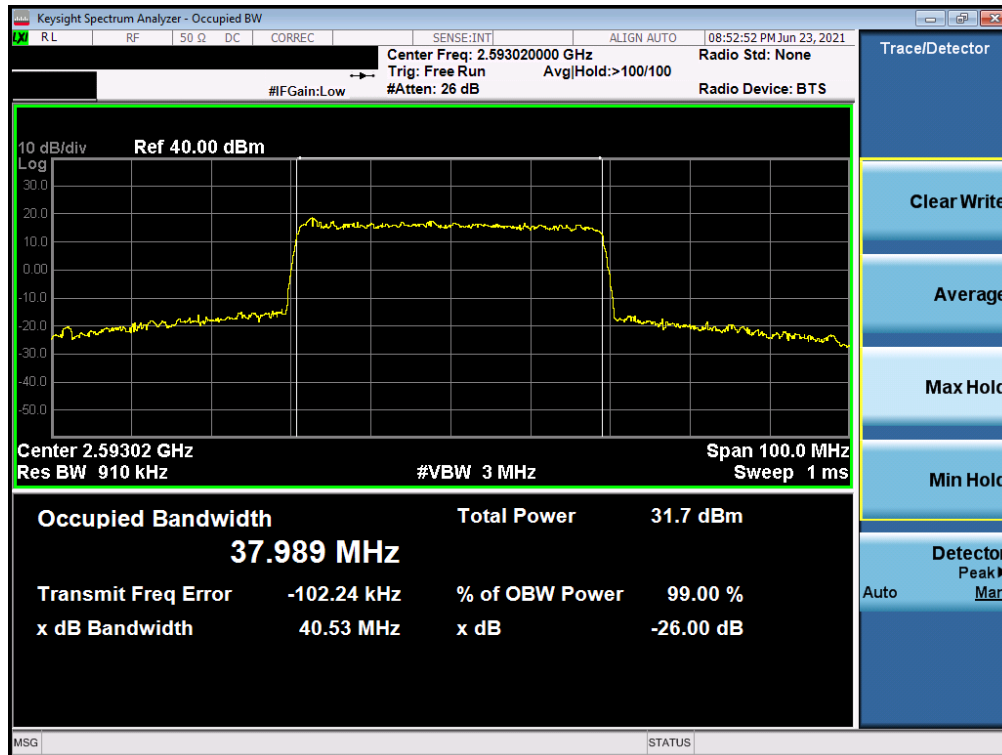
Plot 7-45. Occupied Bandwidth Plot (NR Band n41 - 40MHz QPSK - Full RB)
