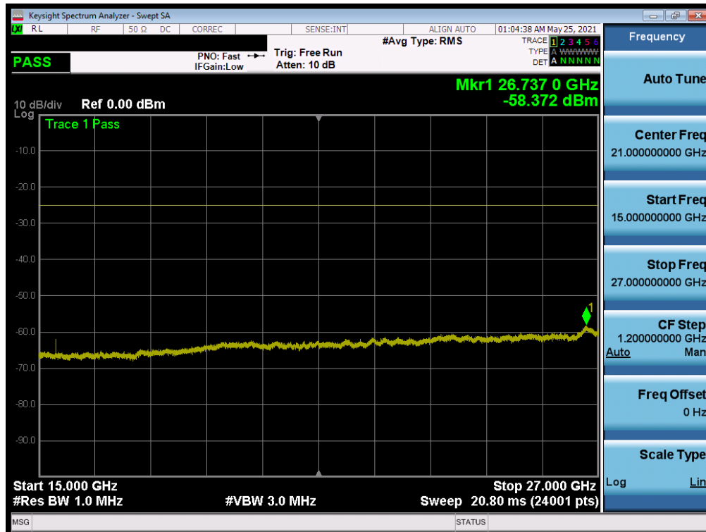
Plot 7-64. Conducted Spurious Plot (LTE Band 7 - 20MHz QPSK - RB Size 1, RB Offset 0 - High Channel)
