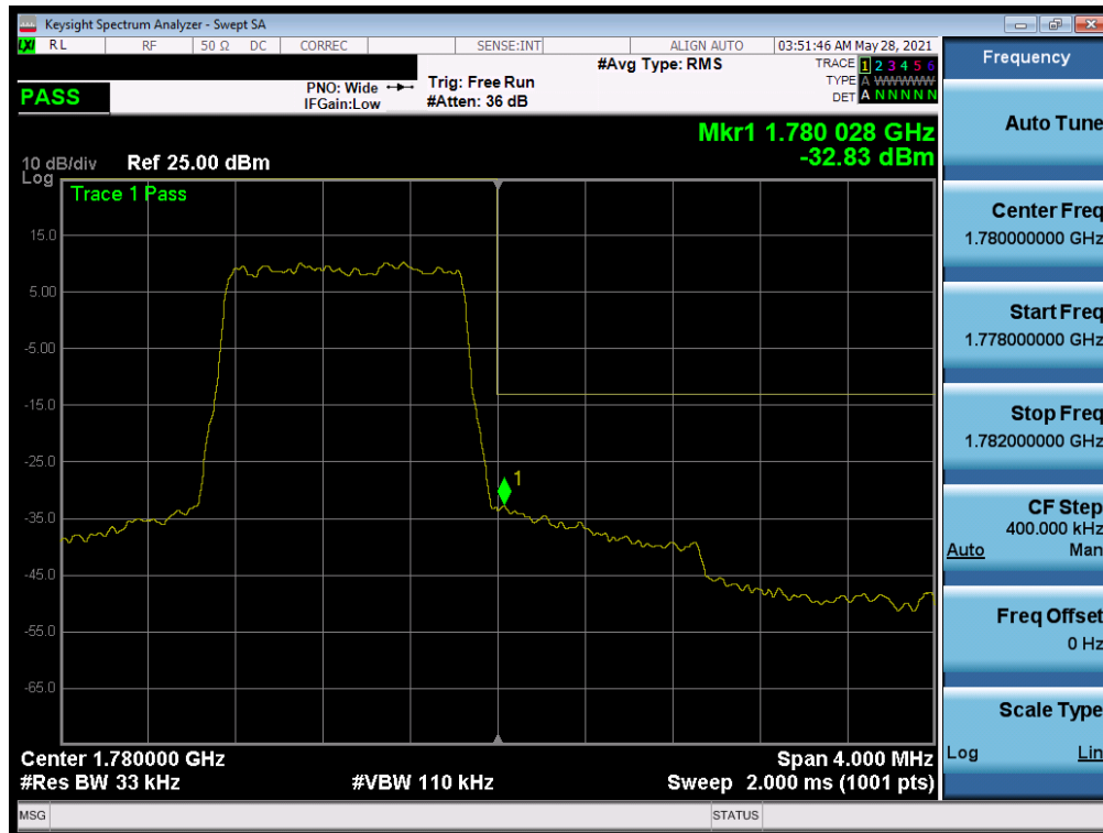
Plot 7-177. Upper Band Edge Plot (LTE Band 66 – 1.4MHz QPSK – Full RB)
