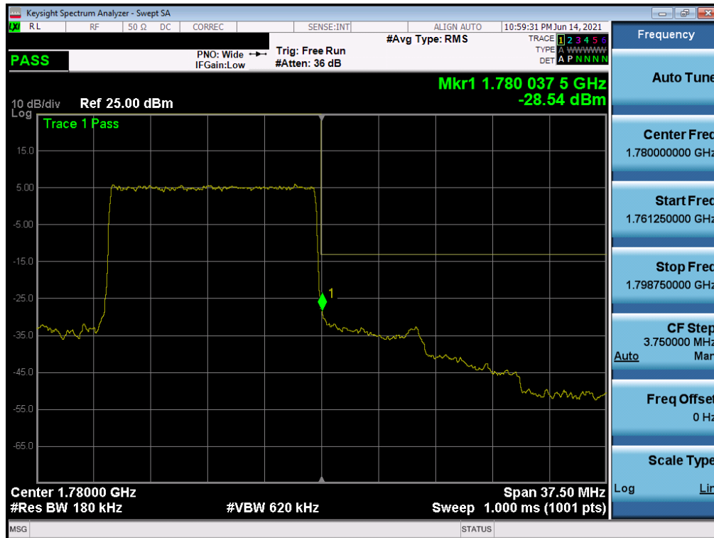
Plot 7-193. Upper Band Edge Plot (NR Band n66 - 15.0MHz - Full RB)
