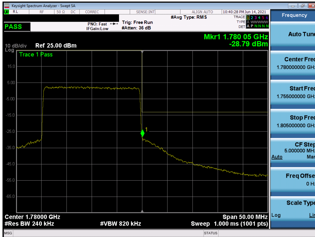
Plot 7-189. Upper Band Edge Plot (NR Band n66 - 20.0MHz - Full RB)
