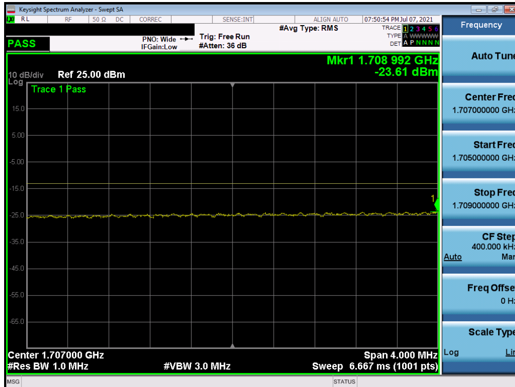
Plot 7-180. Lower Extended Band Edge Plot (NR Band n66 – 40.0MHz - Full RB)
