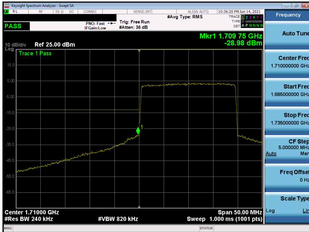
Plot 7-187. Lower Band Edge Plot (NR Band n66 – 20.0MHz - Full RB)
