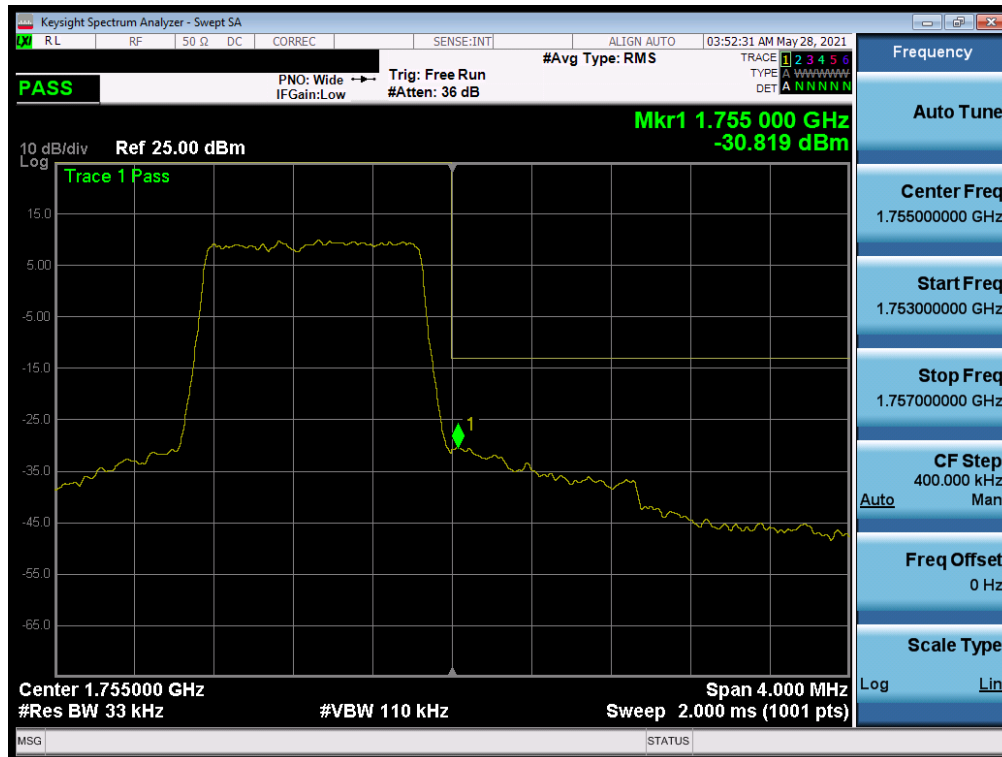
Plot 7-175. Upper Band Edge Plot (LTE Band 4 – 1.4MHz QPSK – Full RB)
