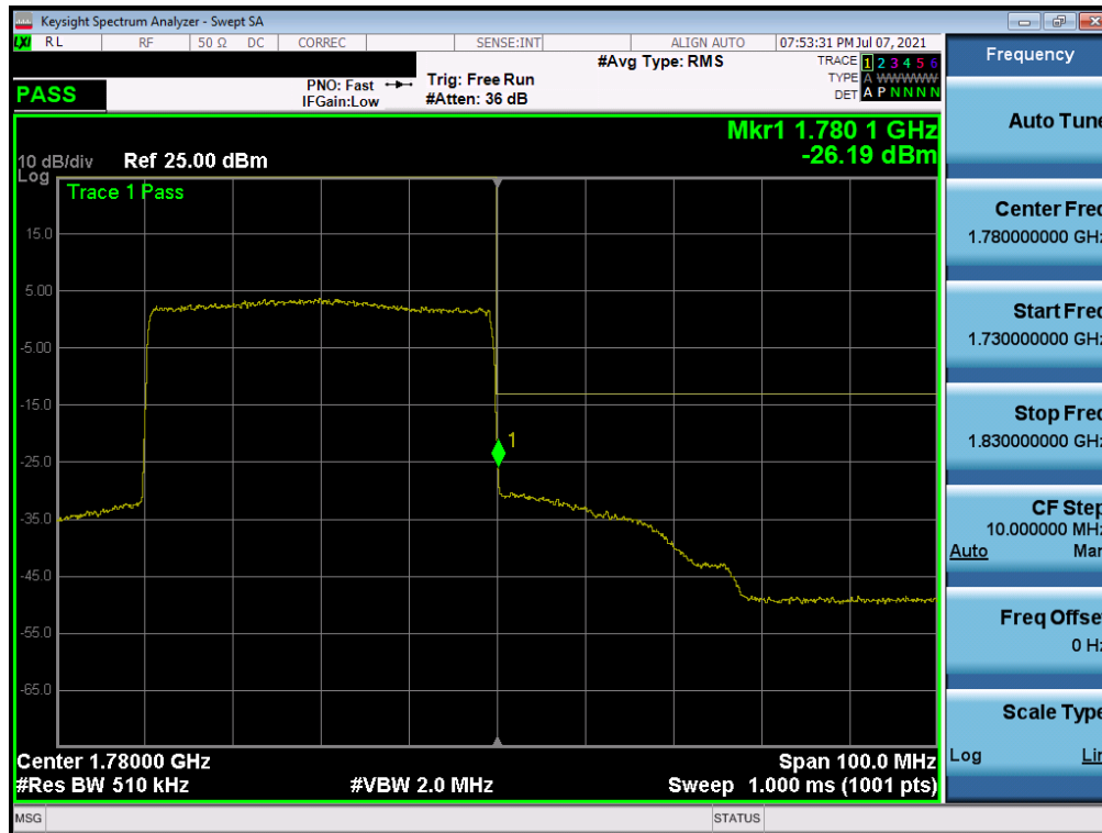
Plot 7-181. Upper Band Edge Plot (NR Band n66 – 40.0MHz - Full RB)
