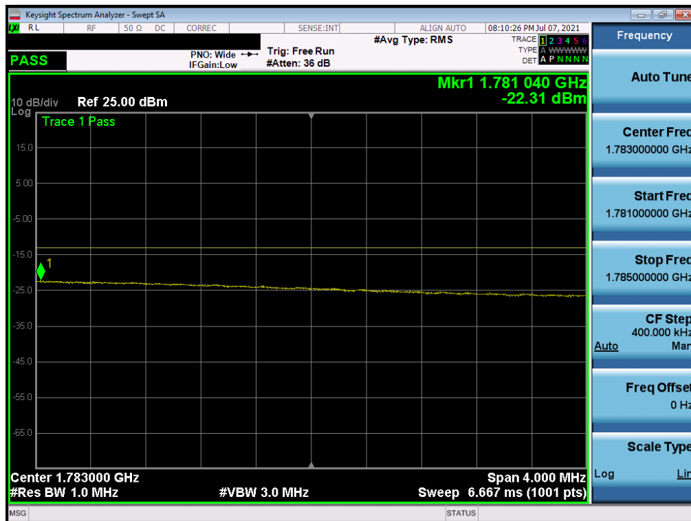
Plot 7-186. Upper Extended Band Edge Plot (NR Band n66 - 30.0MHz - Full RB)
