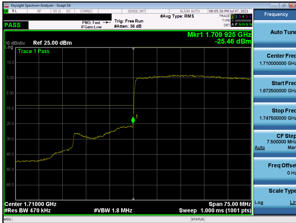
Plot 7-183. Lower Band Edge Plot (NR Band n66 – 30.0MHz - Full RB)
