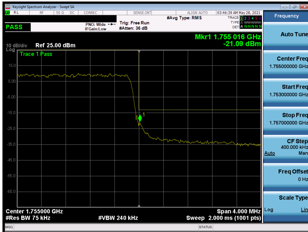
Plot 7-169. Upper Band Edge Plot (LTE Band 4 - 3MHz QPSK – Full RB)
