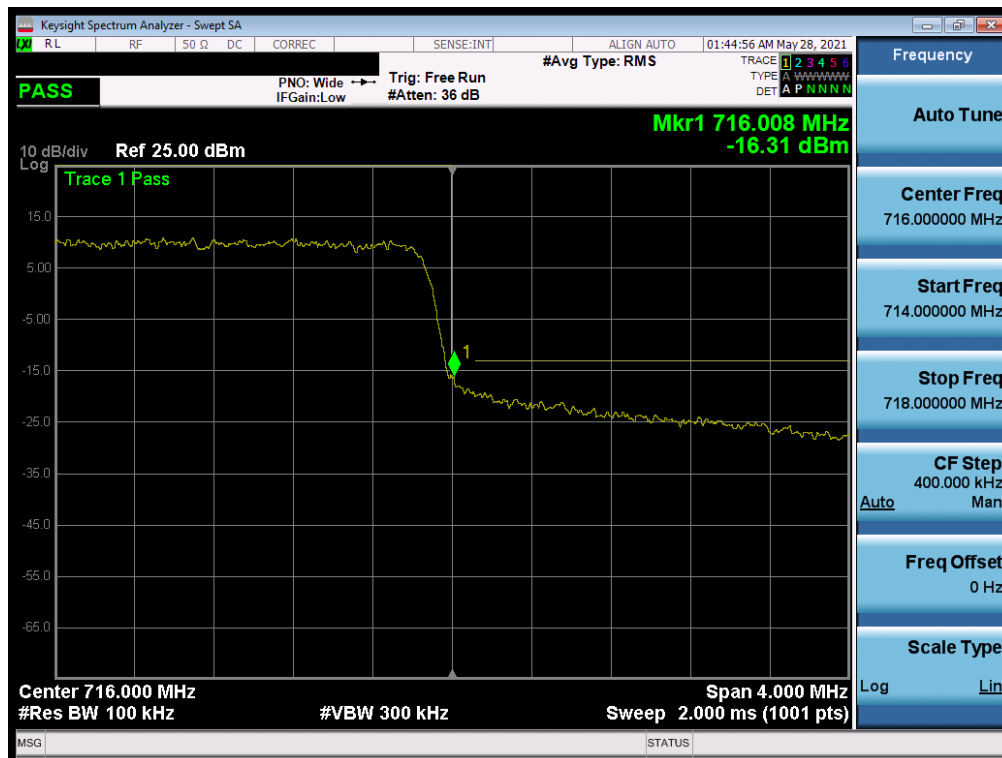
Plot 7-124. Upper Band Edge Plot (LTE Band 12 - 3MHz QPSK - Full RB)
