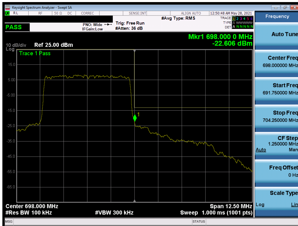
Plot 7-118. Upper Band Edge Plot (LTE Band 71 - 5MHz QPSK - Full RB)
