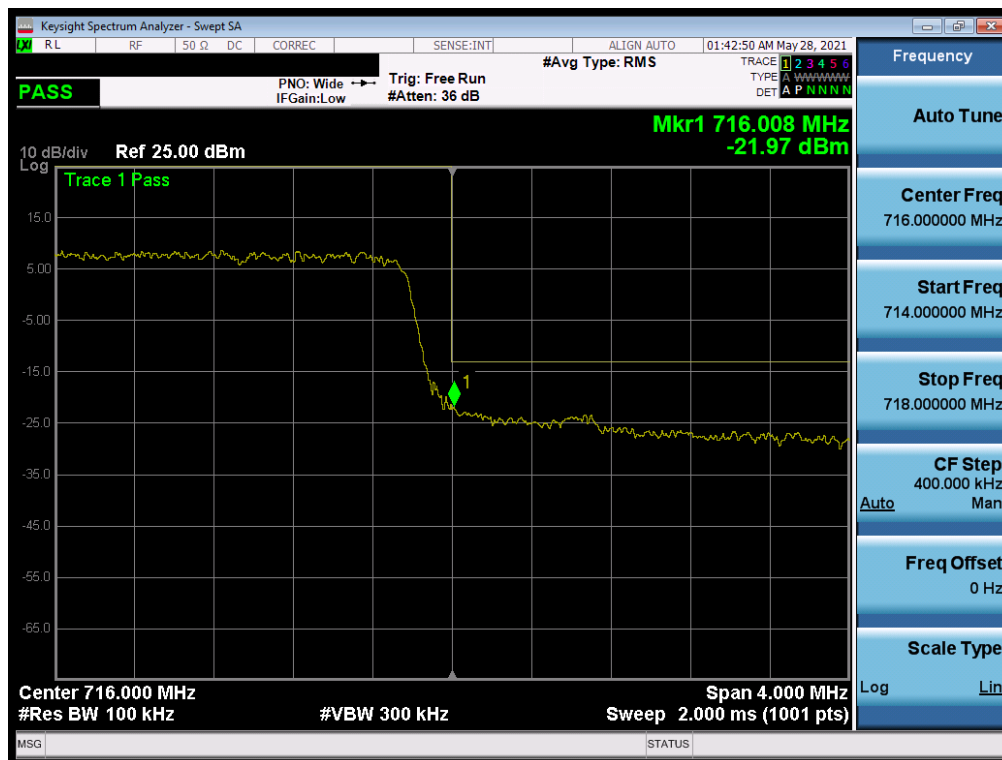
Plot 7-122. Upper Band Edge Plot (LTE Band 12 - 5MHz QPSK - Full RB)
