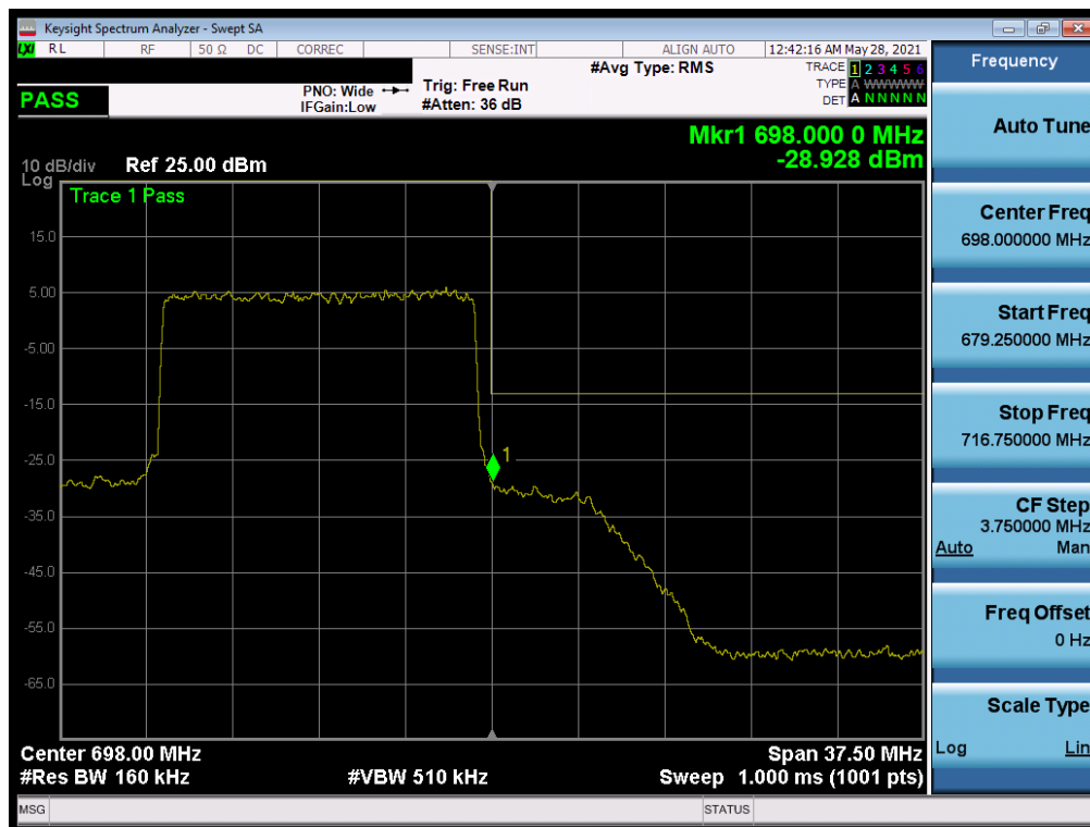
Plot 7-114. Upper Band Edge Plot (LTE Band 71 - 15MHz QPSK – Full RB)
