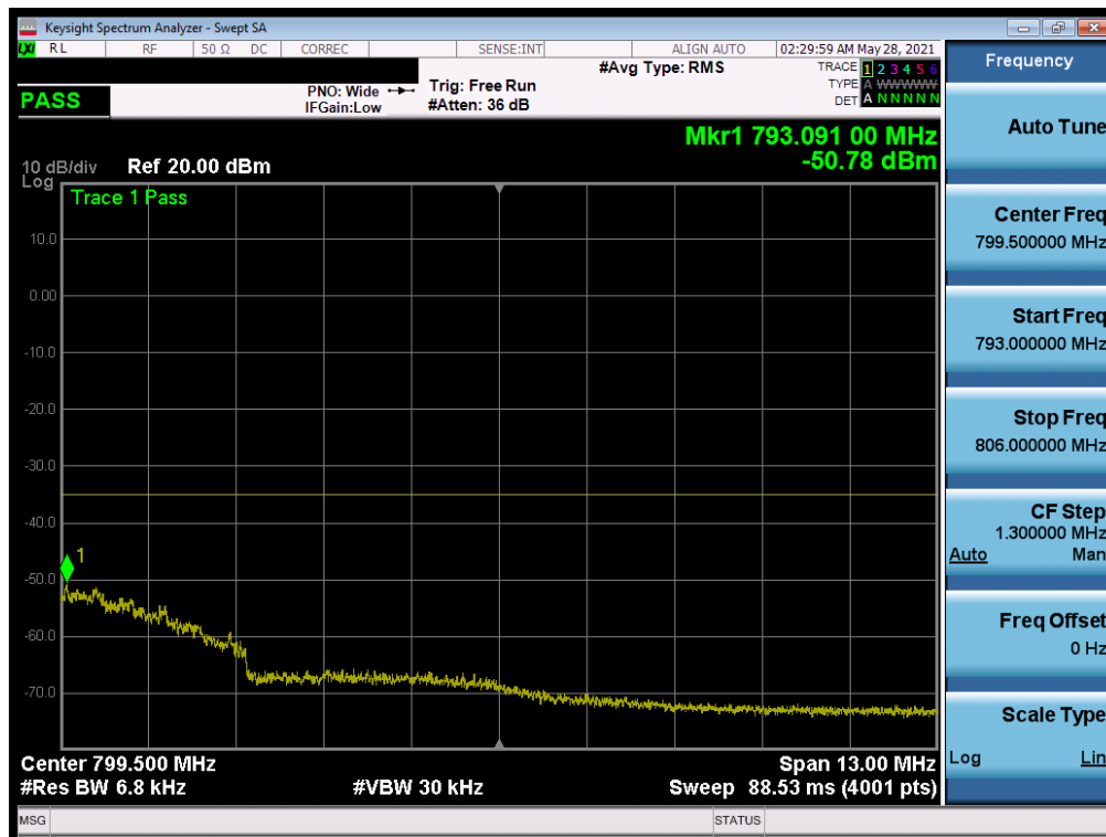
Plot 7-134. Upper Emission Mask Plot (LTE Band 13 - 5MHz QPSK - Full RB)
