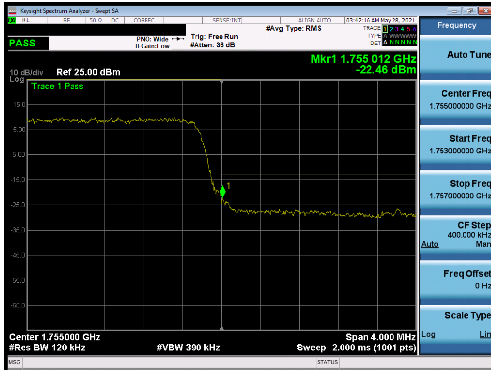
Plot 7-163. Upper Band Edge Plot (LTE Band 4 - 5MHz QPSK – Full RB)
