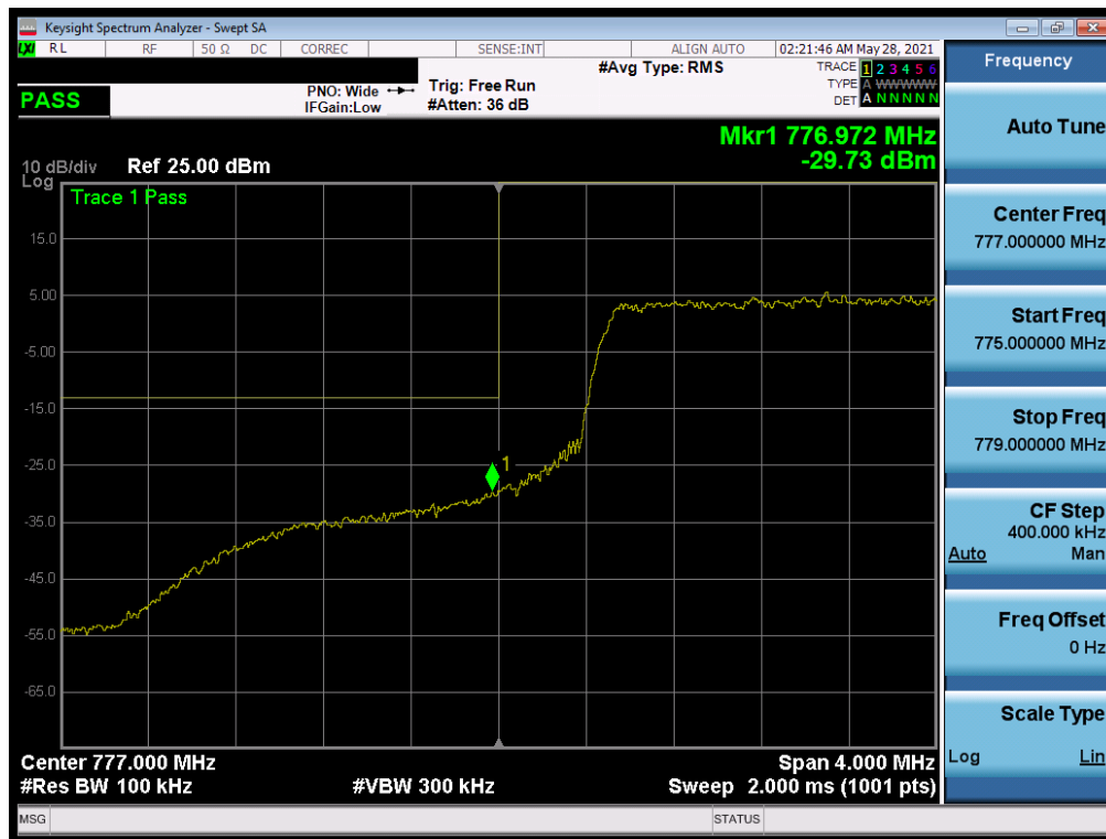
Plot 7-127. Lower Band Edge Plot (LTE Band 13 - 10MHz QPSK – Full RB)
