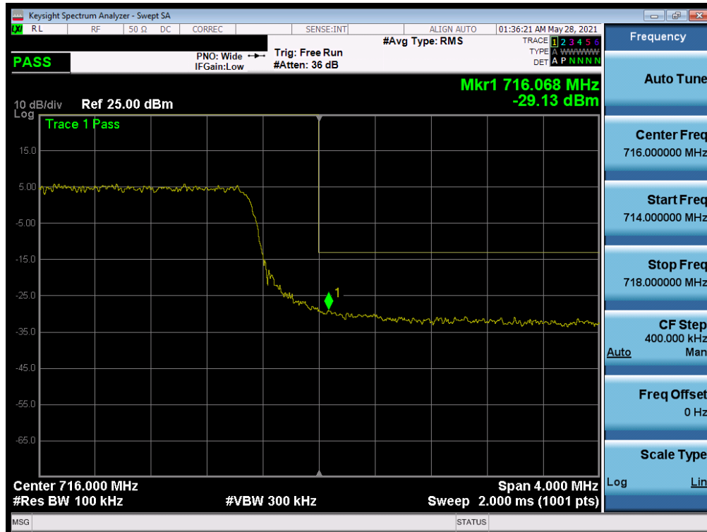
Plot 7-120. Upper Band Edge Plot (LTE Band 12 - 10MHz QPSK – Full RB)
