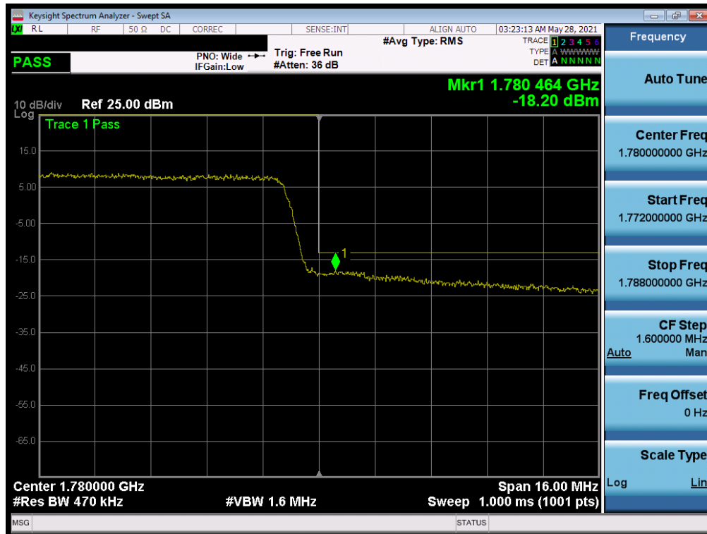
Plot 7-147. Upper Band Edge Plot (LTE Band 66 - 20MHz QPSK – Full RB)
