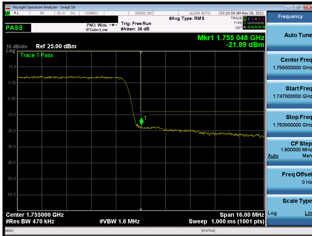
Plot 7-145. Upper Band Edge Plot (LTE Band 4 - 20MHz QPSK – Full RB)
