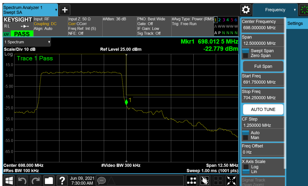
Plot 7-142. Upper Band Edge Plot (NR Band n71 – 5.0MHz - Full RB)
