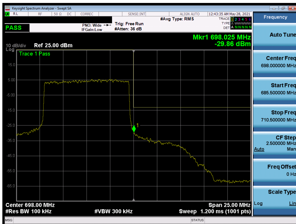
Plot 7-116. Upper Band Edge Plot (LTE Band 71 - 10MHz QPSK – Full RB)
