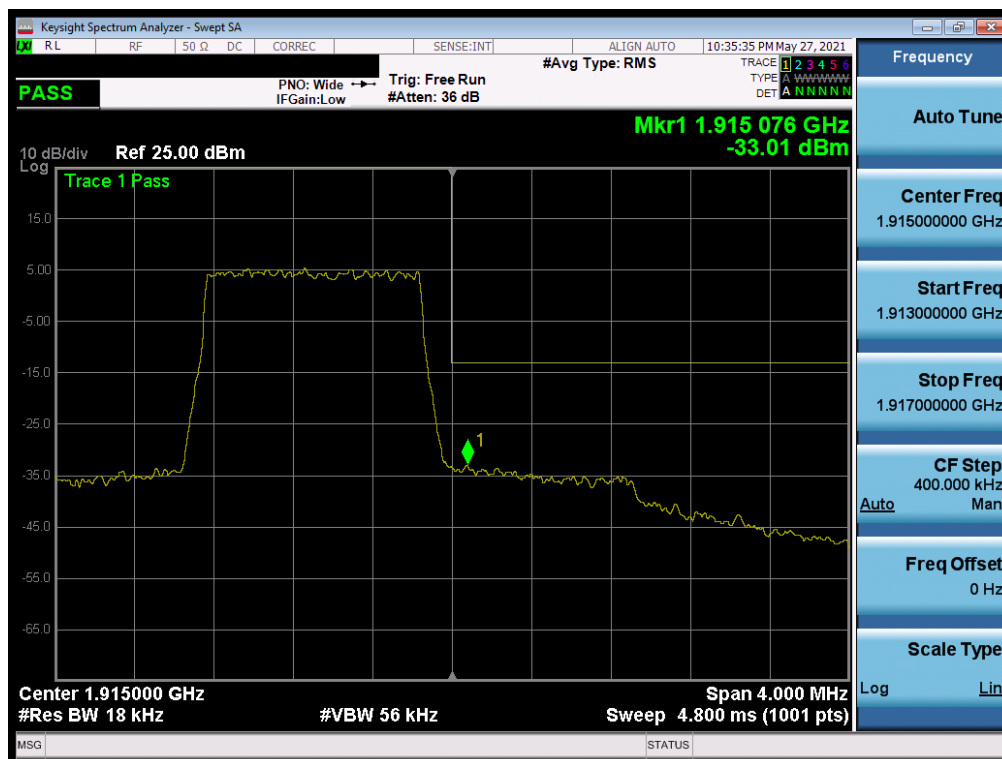
Plot 7-105. Upper Band Edge Plot (LTE Band 25 – 1.4MHz QPSK – Full RB)
