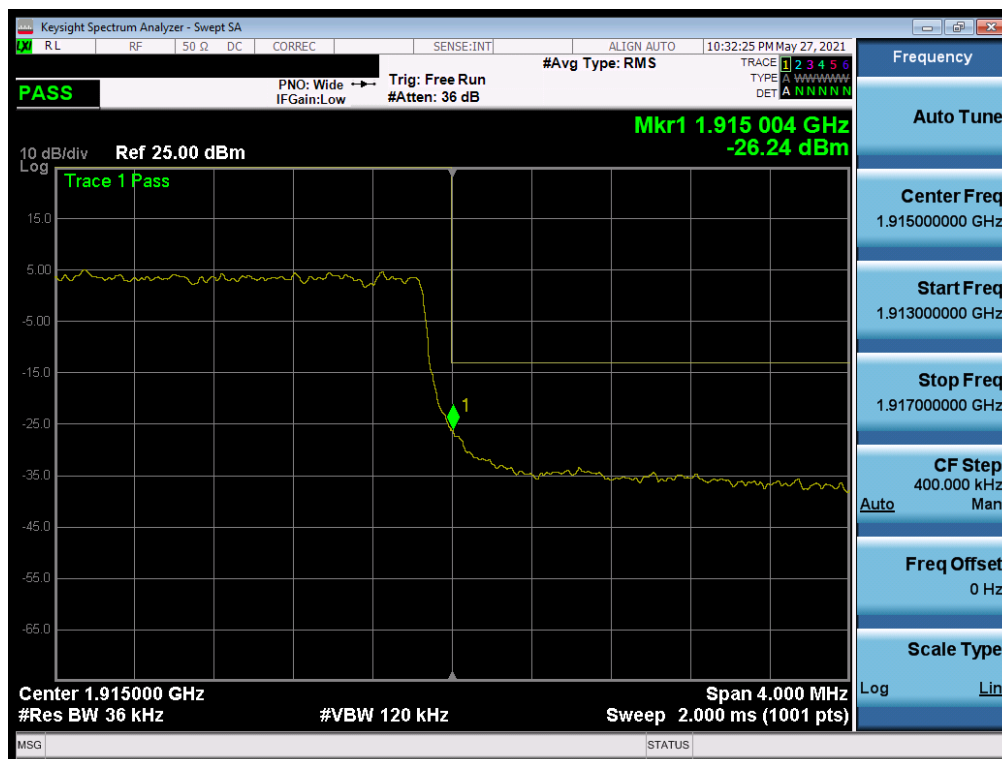
Plot 7-99. Upper Band Edge Plot (LTE Band 25 - 3MHz QPSK – Full RB)
