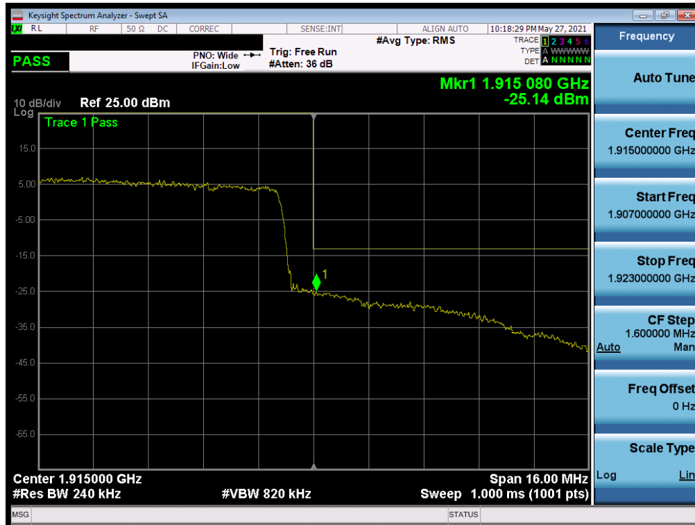
Plot 7-75. Upper Band Edge Plot (LTE Band 25 - 20MHz QPSK – Full RB)
