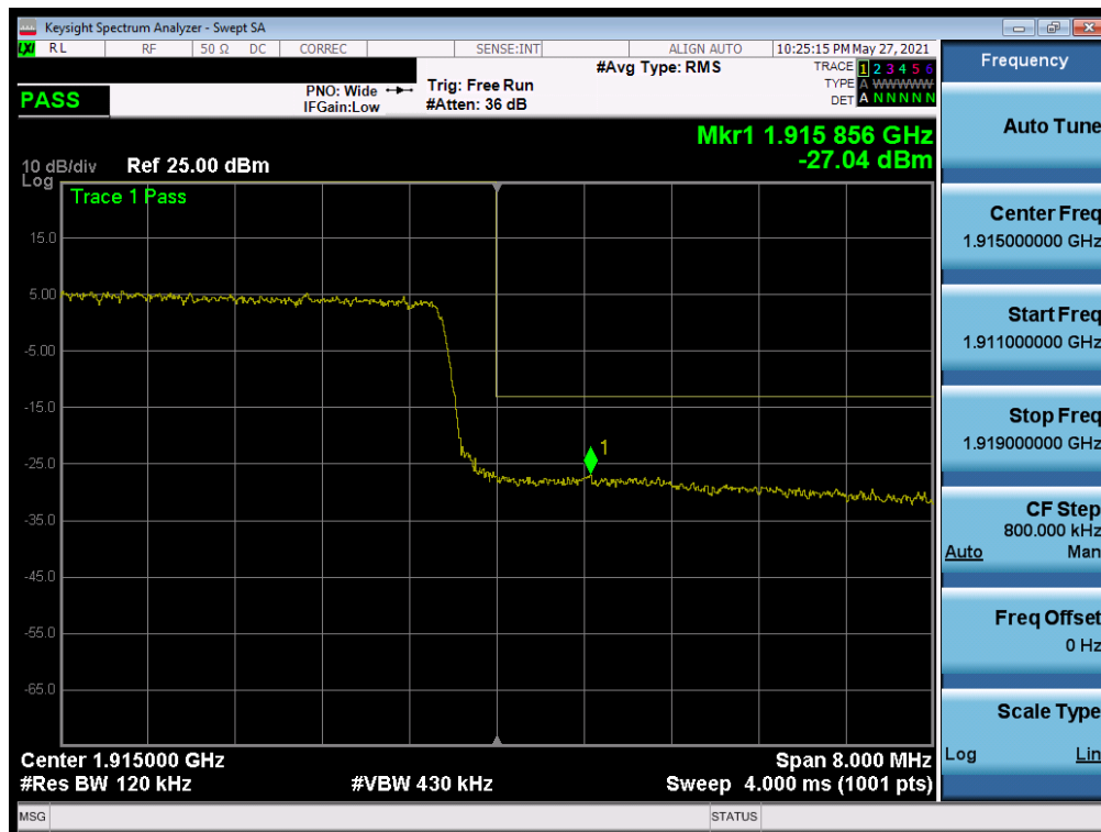
Plot 7-87. Upper Band Edge Plot (LTE Band 25 - 10MHz QPSK – Full RB)
