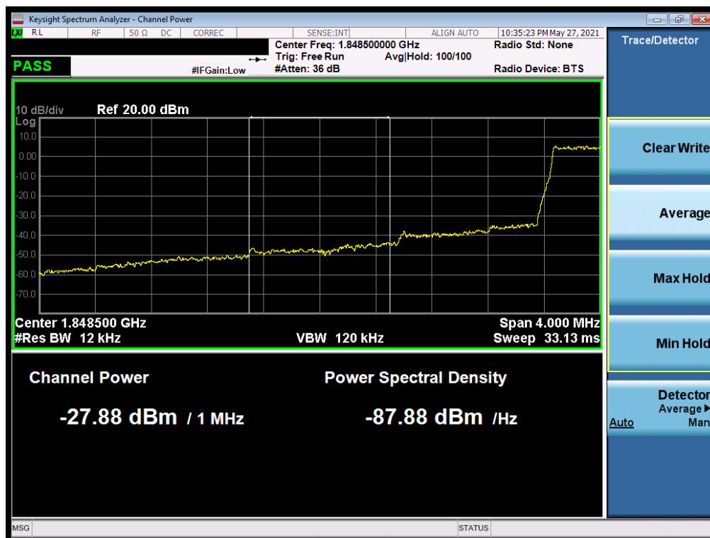
Plot 7-103. Extended Lower Band Edge Plot (LTE Band 25/2 – 1.4MHz QPSK – Full RB)
