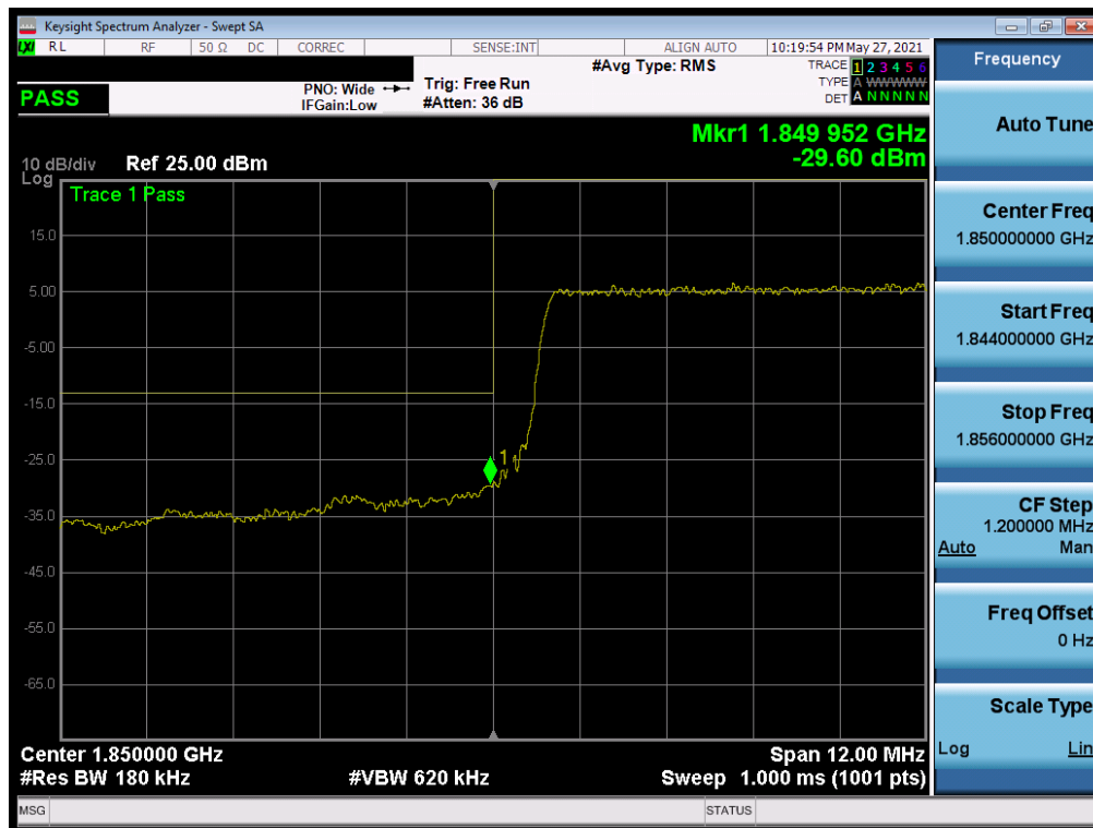
Plot 7-78. Lower Band Edge Plot (LTE Band 25/2 - 15MHz QPSK – Full RB)
