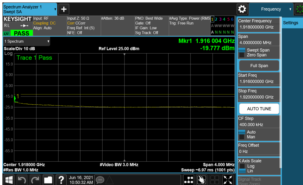
Plot 7-131. Extended Upper Band Edge Plot (NR Band n25 - 15MHz QPSK – Full RB)
