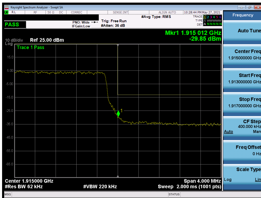
Plot 7-93. Upper Band Edge Plot (LTE Band 25 - 5MHz QPSK – Full RB)
