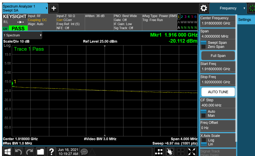
Plot 7-125. Extended Upper Band Edge Plot (NR Band n25 - 20MHz QPSK – Full RB)
