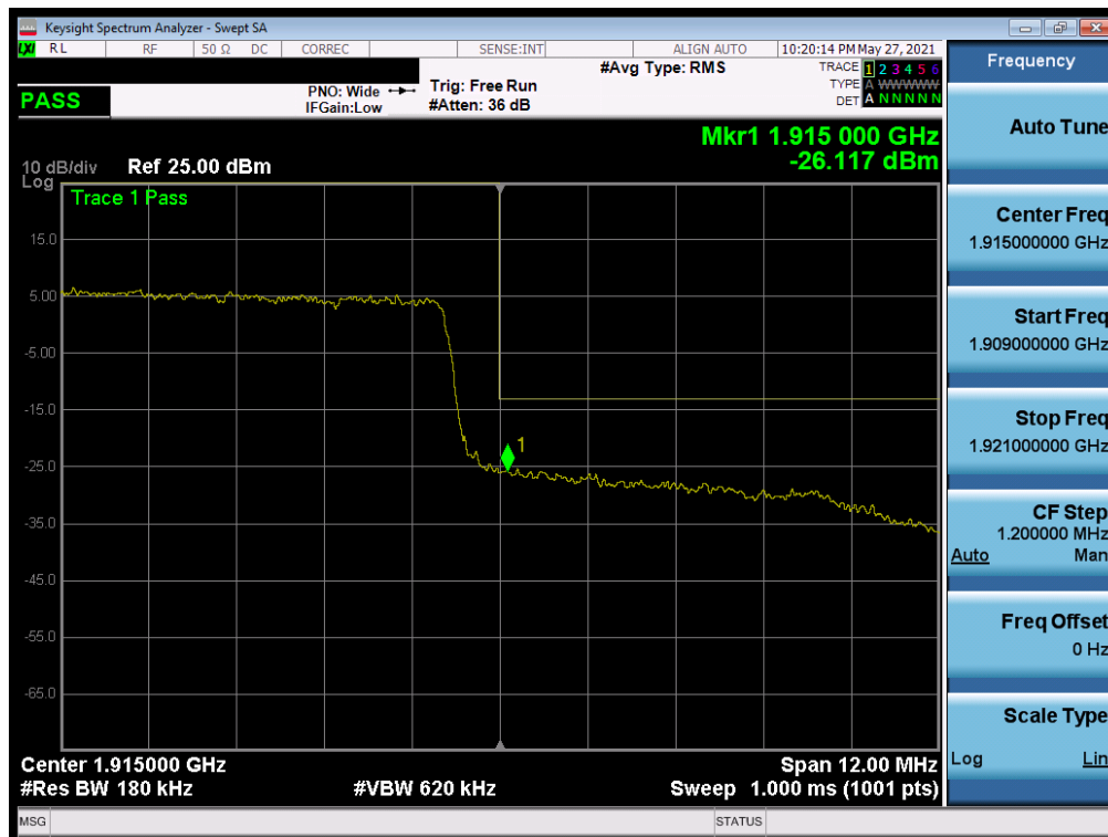
Plot 7-81. Upper Band Edge Plot (LTE Band 25 - 15MHz QPSK – Full RB)
