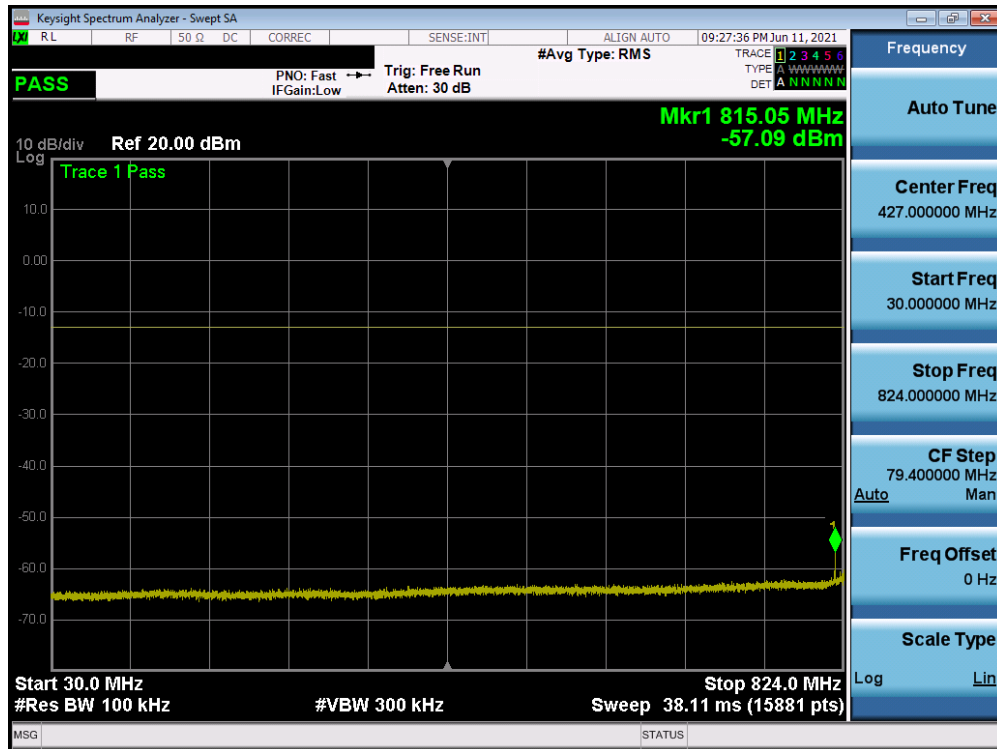
Plot 7-40. Conducted Spurious Plot (NR Band n5 - 20.0MHz - 1 RB - High Channel)
