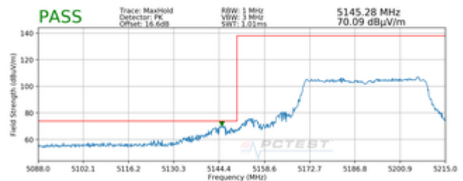
Plot 7-480. Radiated Lower Band Edge Plot SISO NORTH (Peak – UNII Band 1 – 484 Tones)
