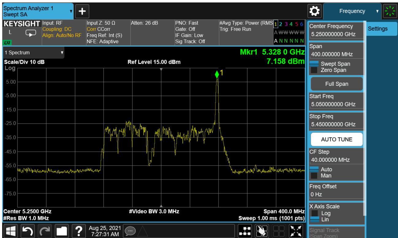
Plot 7-256. Power Spectral Density Plot MIMO SOUTH (160MHz BW (U) 802.11ax – 26 Tones (UNII Band 2A) – Ch. 50)
