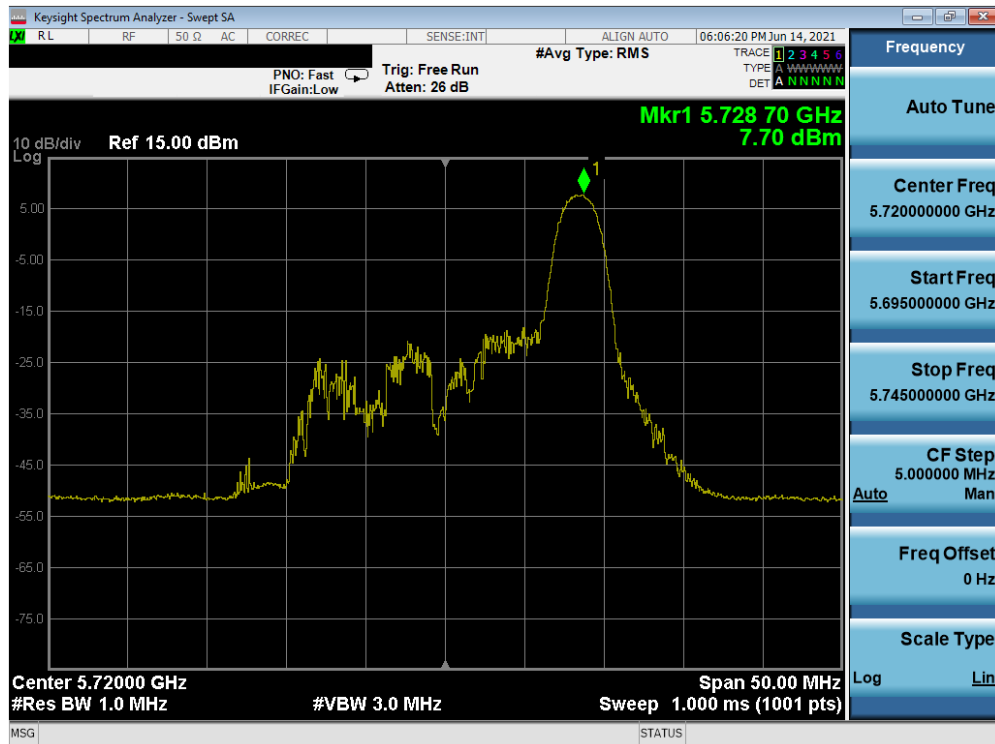
Plot 7-265. Power Spectral Density Plot MIMO SOUTH (20MHz BW 802.11ax – 26 Tones (UNII Band 2C) – Ch. 144)
