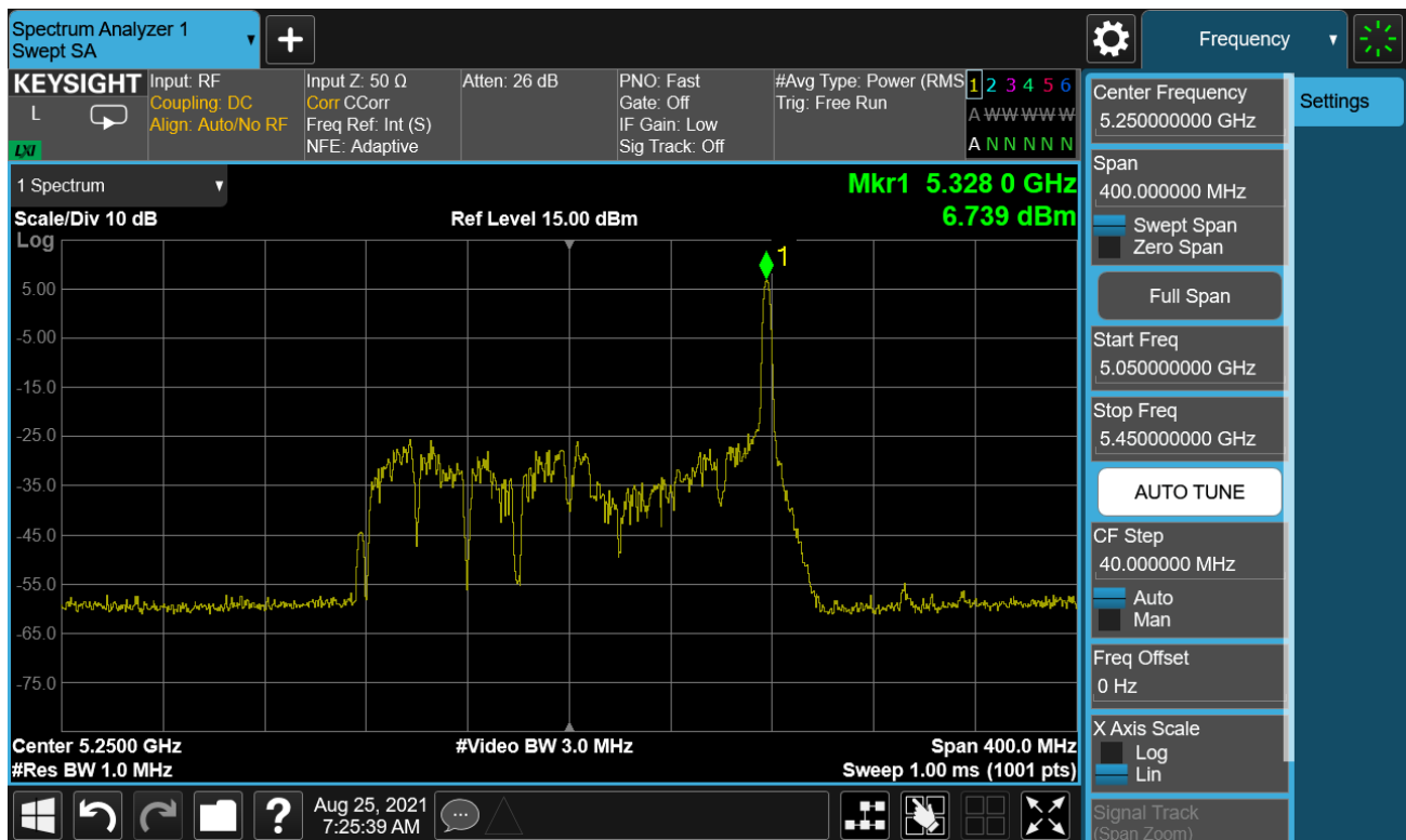
Plot 7-318. Power Spectral Density Plot MIMO NORTH (160MHz BW (U) 802.11ax – 26 Tones (UNII Band 2A) – Ch. 50)
