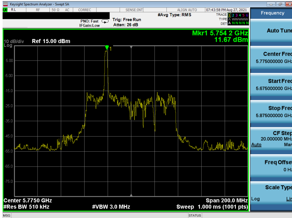
Plot 7-341. Power Spectral Density Plot MIMO NORTH (80MHz BW 802.11ax – 26 Tones (UNII Band 3) – Ch. 155)
