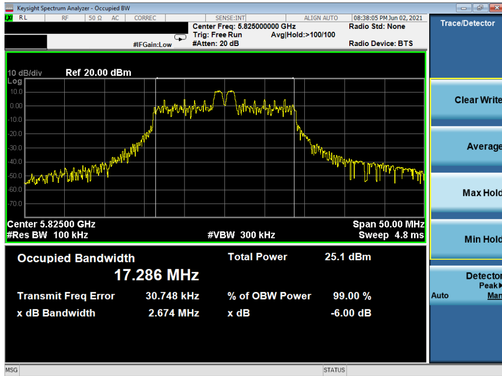
Plot 7-115. 6dB Bandwidth Plot SISO NORTH (20MHz BW 802.11ax – 26 Tones (UNII Band 3) – Ch. 165)
