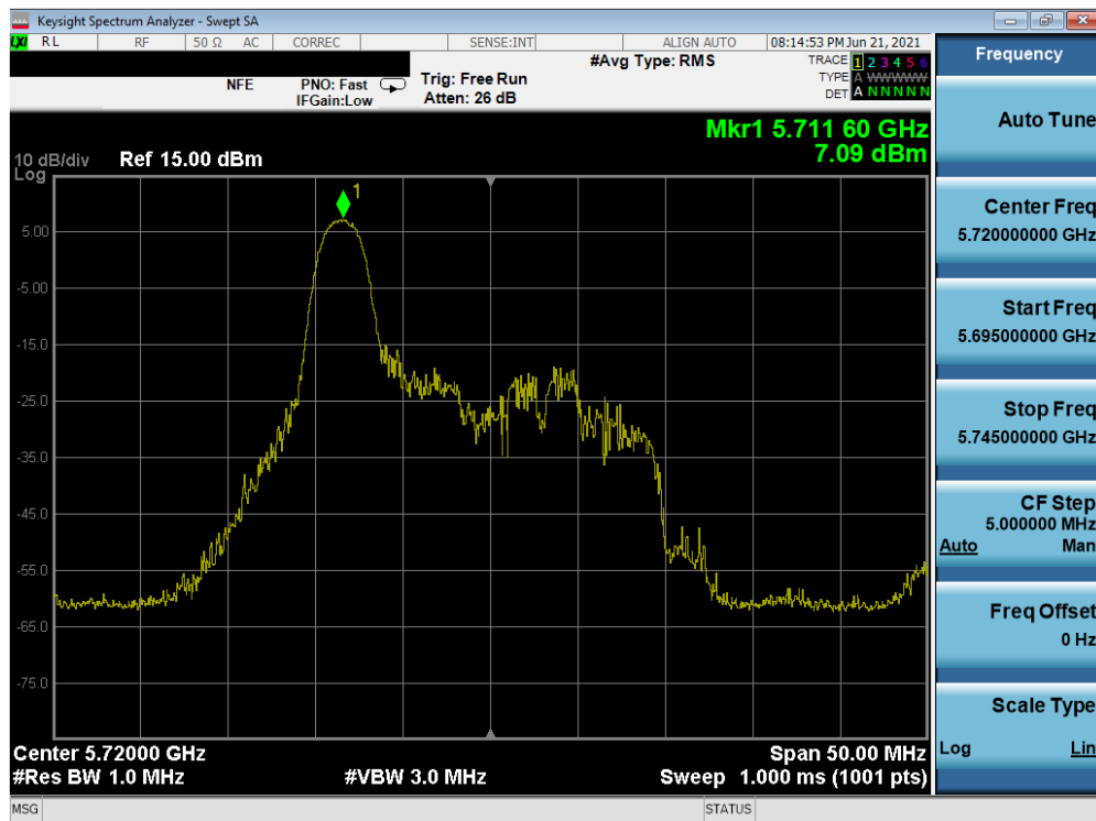
Plot 7-141. Power Spectral Density Plot SISO SOUTH (20MHz BW 802.11ax – 26 Tones (UNII Band 2C) – Ch. 144)
