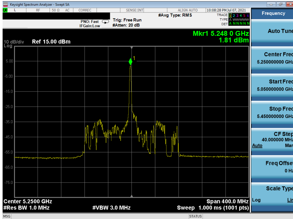
Plot 7-131. Power Spectral Density Plot SISO SOUTH (160MHz BW (L) 802.11ax – 26 Tones (UNII Band 1) – Ch. 50)
