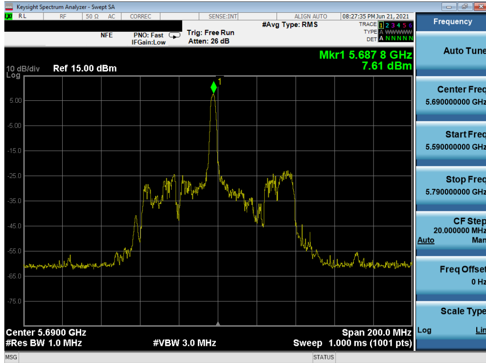
Plot 7-147. Power Spectral Density Plot SISO SOUTH (80MHz BW 802.11ax – 26 Tones (UNII Band 2C) – Ch. 138)
