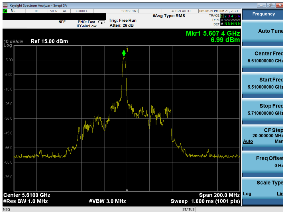
Plot 7-146. Power Spectral Density Plot SISO SOUTH (80MHz BW 802.11ax – 26 Tones (UNII Band 2C) – Ch. 122)
