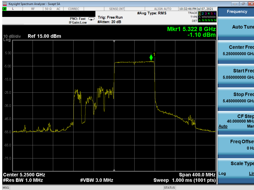
Plot 7-163. Power Spectral Density Plot SISO SOUTH (160MHz BW (U) 802.11ax – Full Tones (UNII Band 2A) – Ch. 50)
