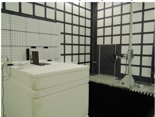
Radiated Emission Set up Photos (Above 18GHz)
