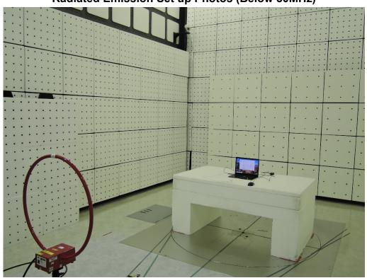
Radiated Emission Set up Photos (Below 1GHz)
