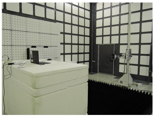
Radiated Emission Set up Photos (Above 18GHz)
