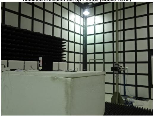
Radiated Emission Set up Photos (Above 18GHz)
