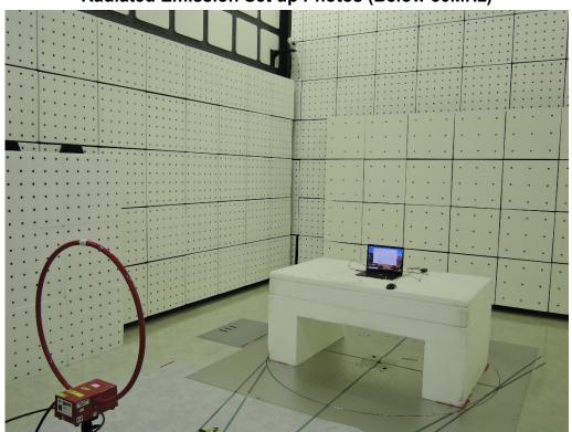
Radiated Emission Set up Photos (Below 1GHz)
