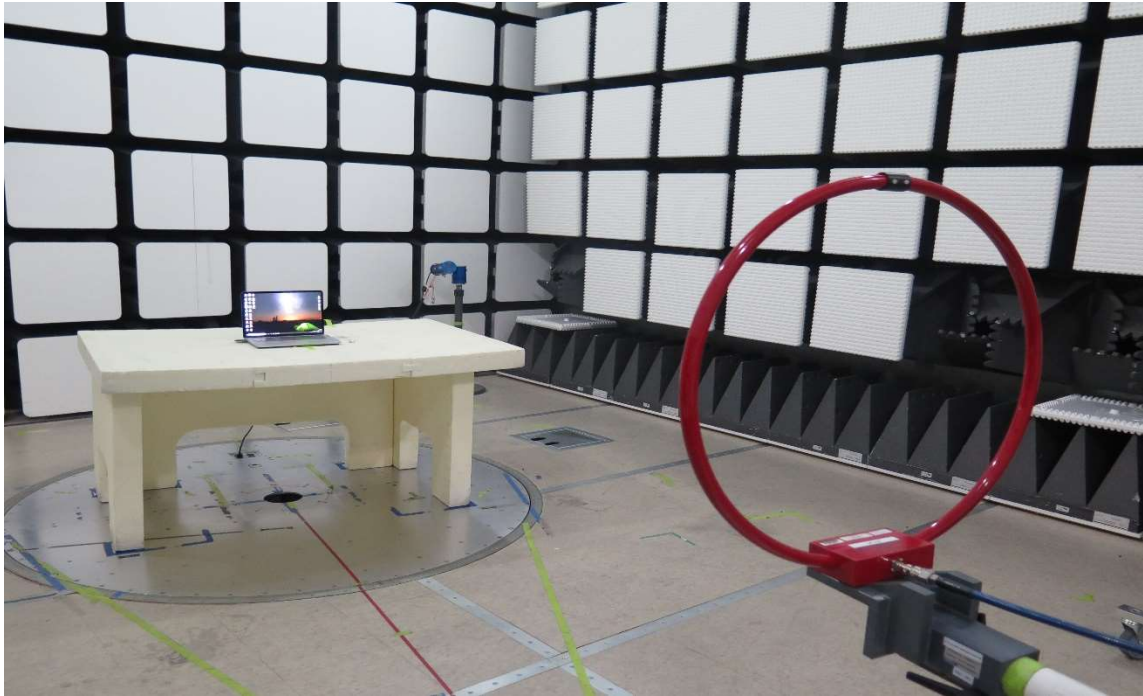
Figure 1 Radiated Spurious Emissions Test Setup (9K-30MHz) – Upright Posture - Parallel
