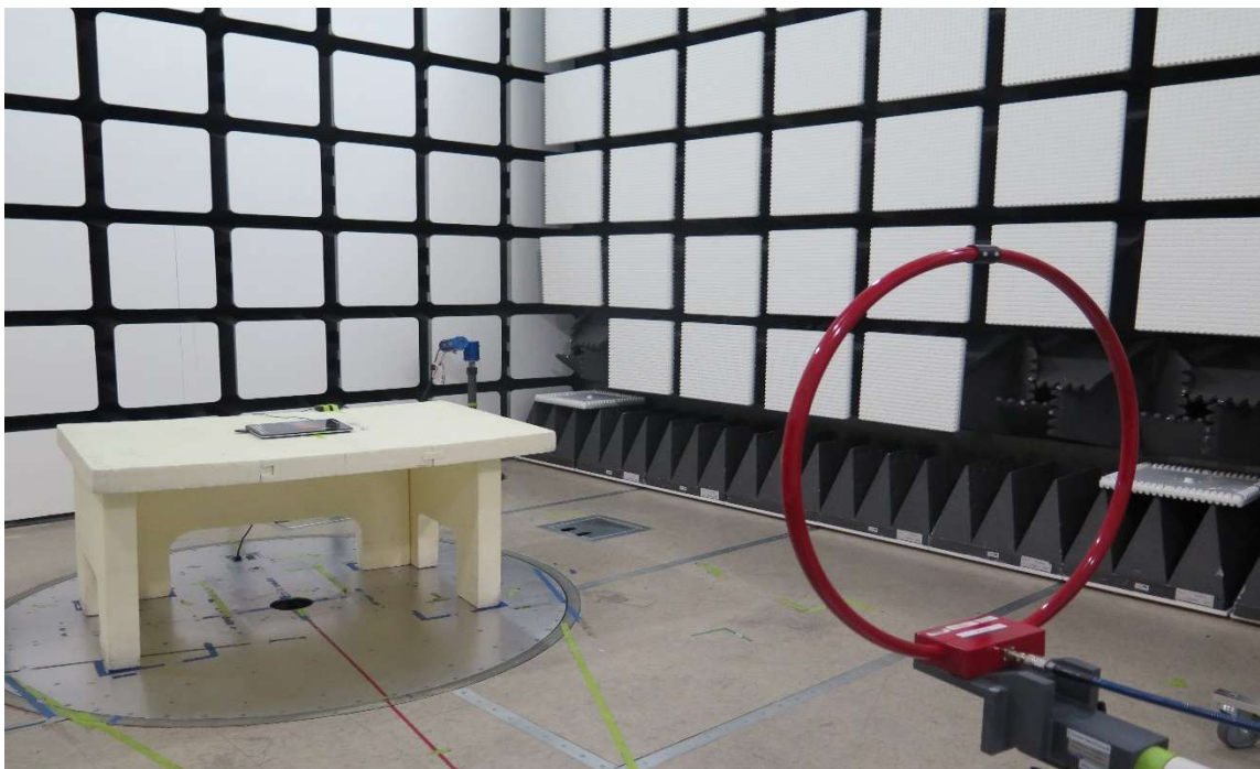
Figure 2 Radiated Spurious Emissions Test Setup (9k-30MHz) – Flat Posture – X - Parallel
