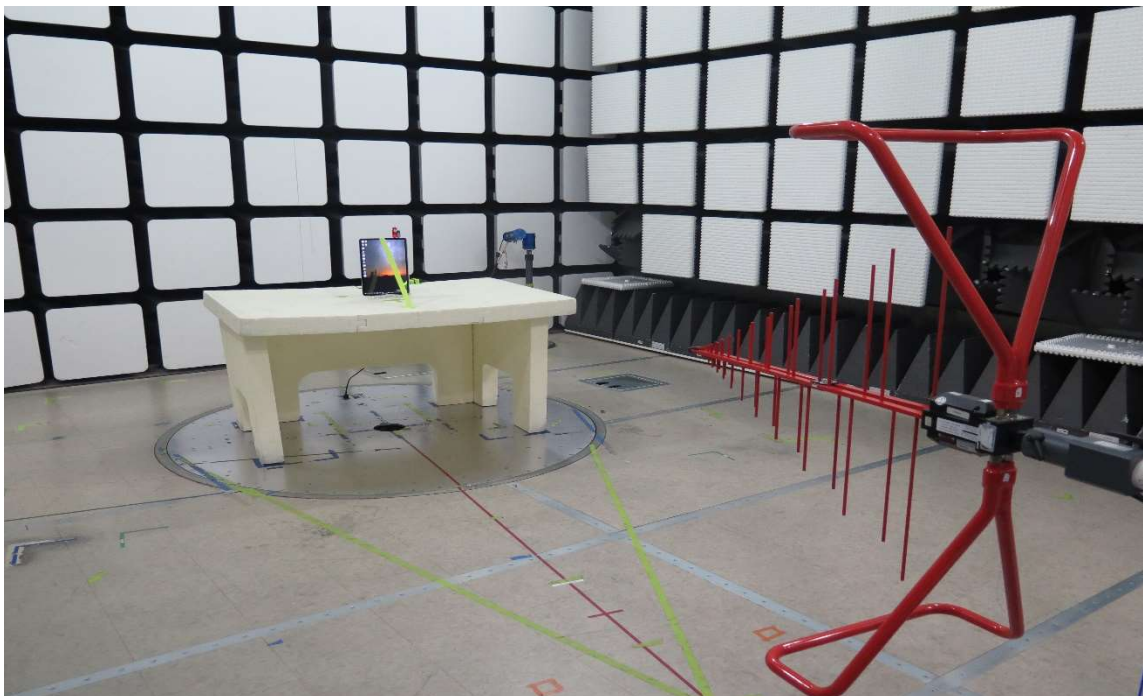
Figure 8 Radiated Spurious Emissions Test Setup (30M-1GHz) – Flat Posture – Z - Parallel.
