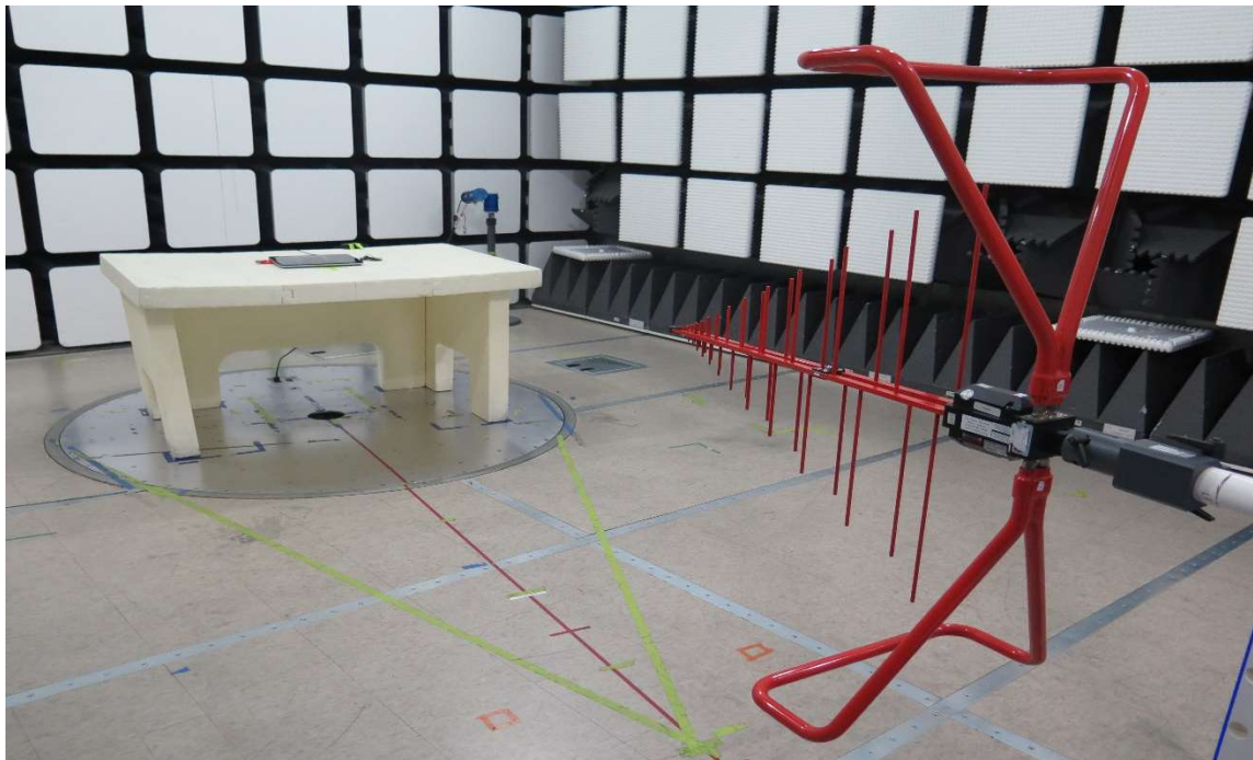
Figure 6 Radiated Spurious Emissions Test Setup (30M-1GHz) – Flat Posture – X - Parallel
