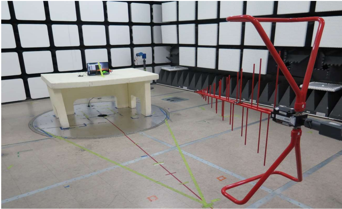
Figure 7 Radiated Spurious Emissions Test Setup (30M-1GHz) – Flat Posture – Y - Parallel.
