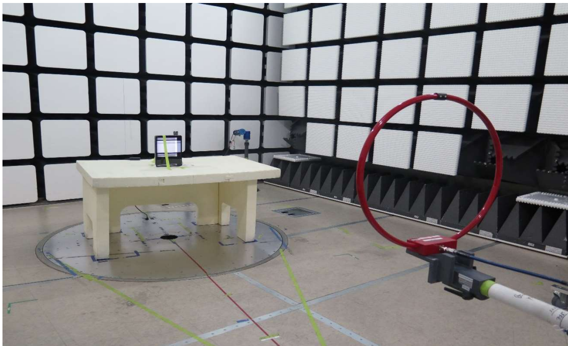
Figure 4 Radiated Spurious Emissions Test Setup (9k-30MHz) – Flat Posture – Z - Parallel
