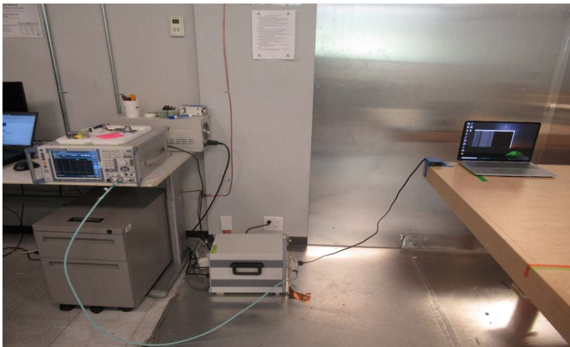
Figure 10 AC Line Conducted Emissions Test Setup
