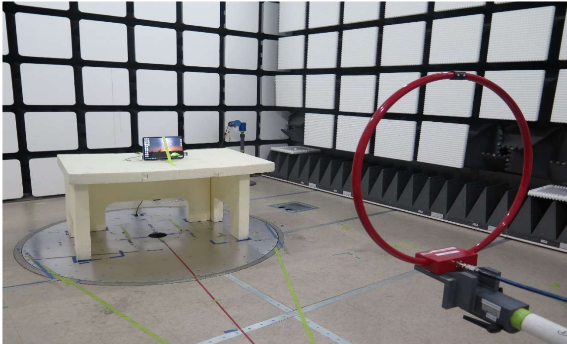
Figure 3 Radiated Spurious Emissions Test Setup (9k-30MHz) – Flat Posture – Y - Parallel
