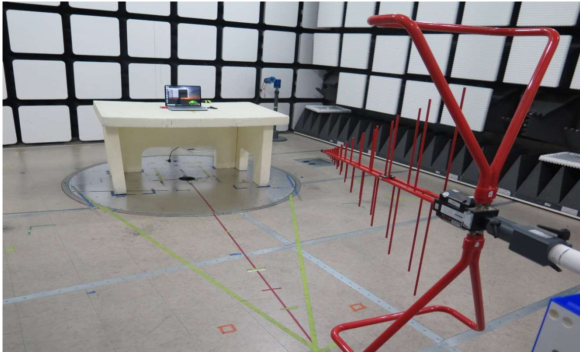
Figure 5 Radiated Spurious Emissions Test Setup (30M-1GHz) – Upright Posture - Parallel
