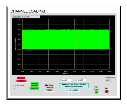
The level of traffic loading on the channel by the EUT is 40.15%
