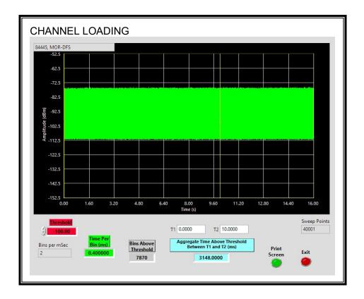
The level of traffic loading on the channel by the EUT is 31.48%
