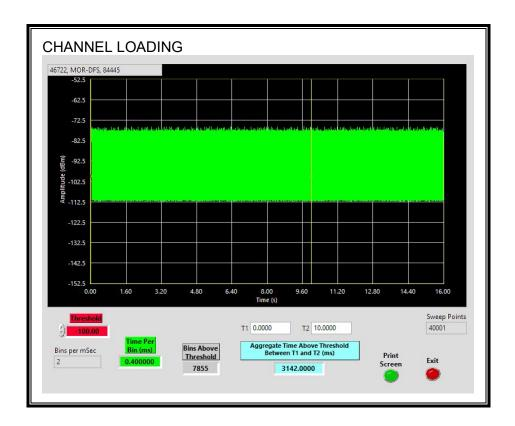
The level of traffic loading on the channel by the EUT is 31.42%
