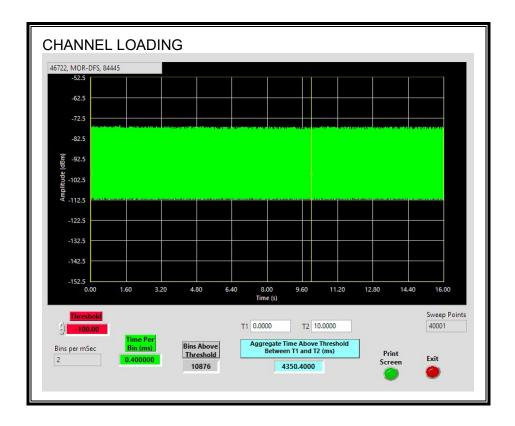
The level of traffic loading on the channel by the EUT is 43.5%
