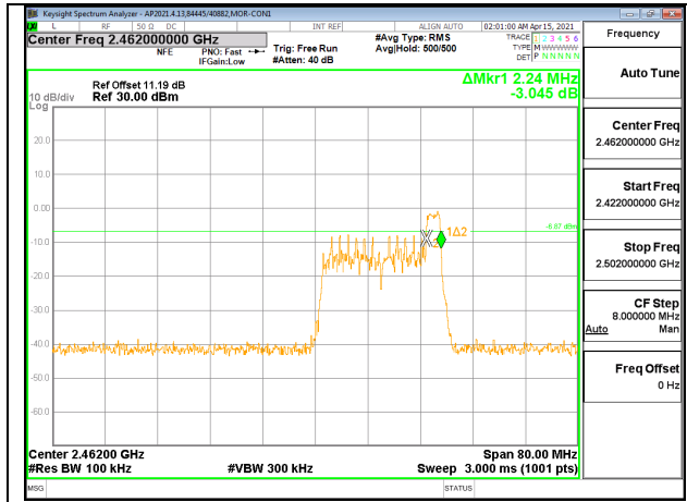
HIGH CHANNEL 11 Antenna A
