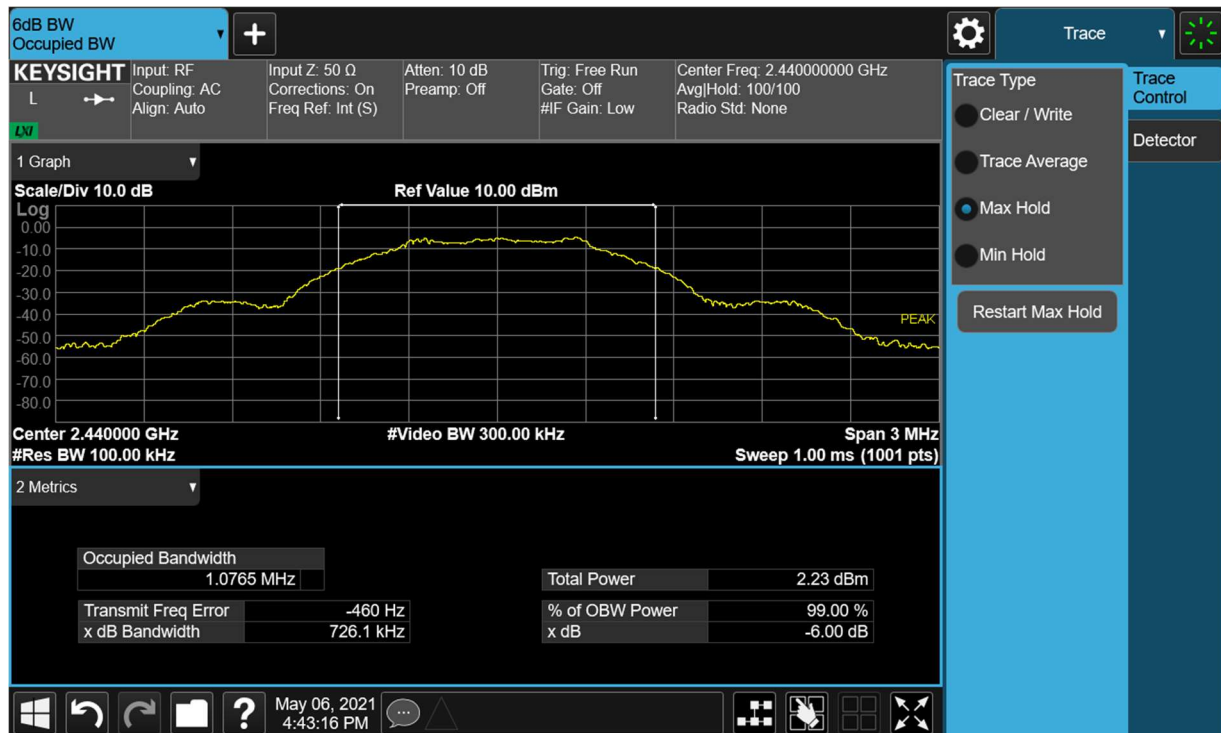
Figure 9-3 6dB Bandwidth (Ch. 19)
