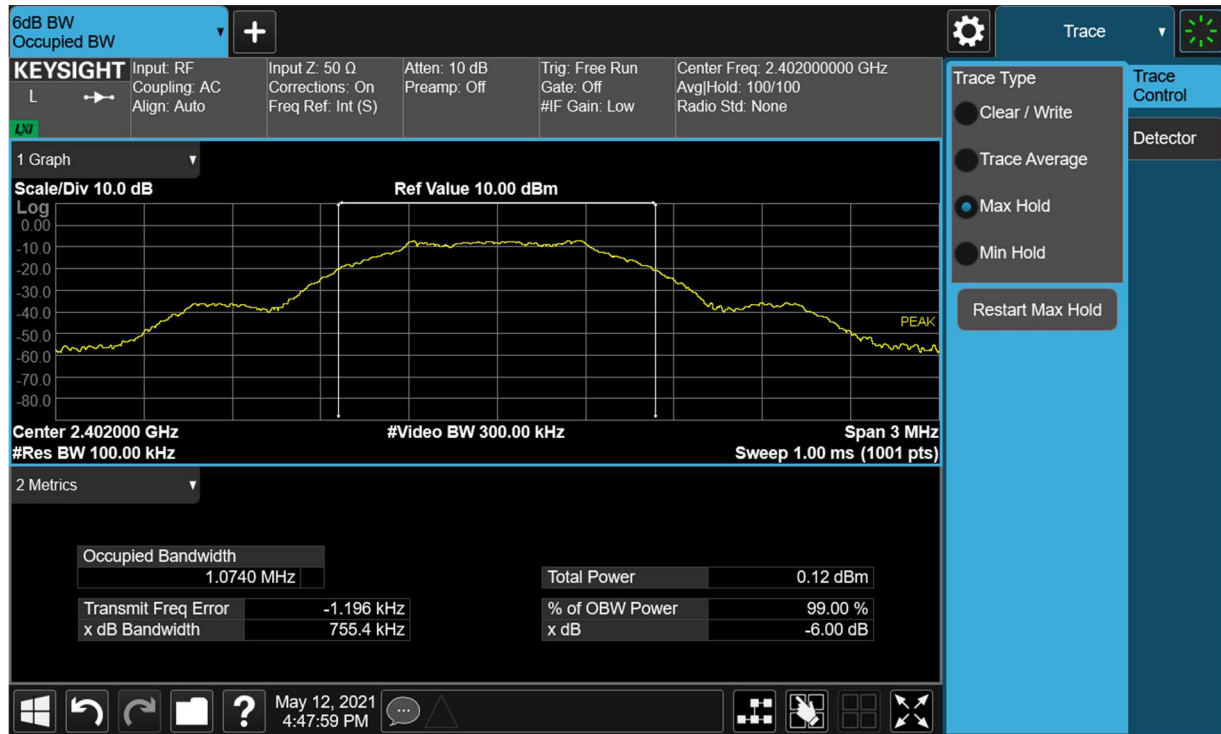
Figure 9-2 6dB Bandwidth (Ch. 0)
