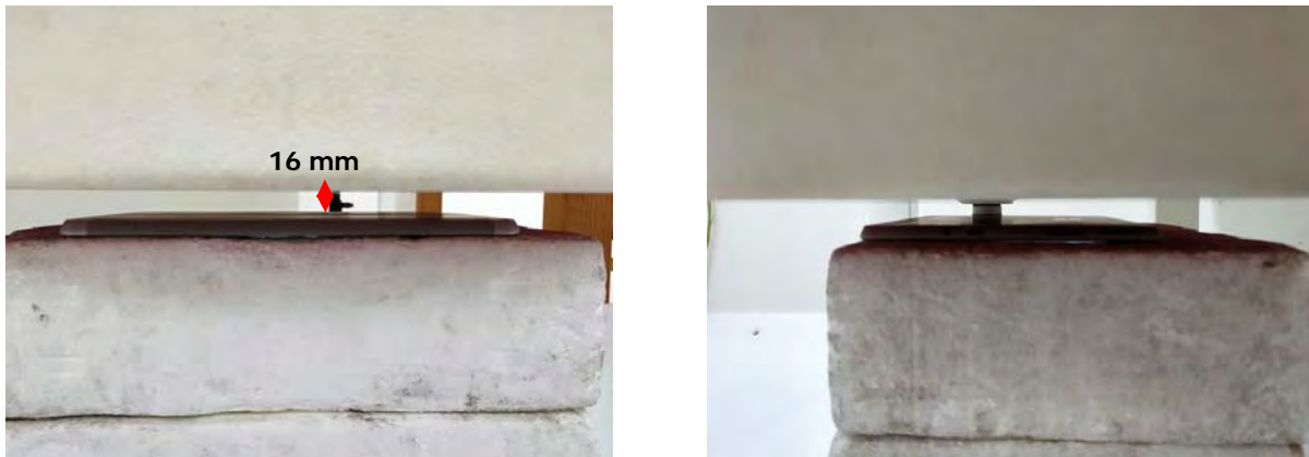
Fig.11 EUT Back side to flat phantom
