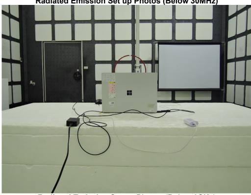
Radiated Emission Set up Photos (Below 1GHz)
