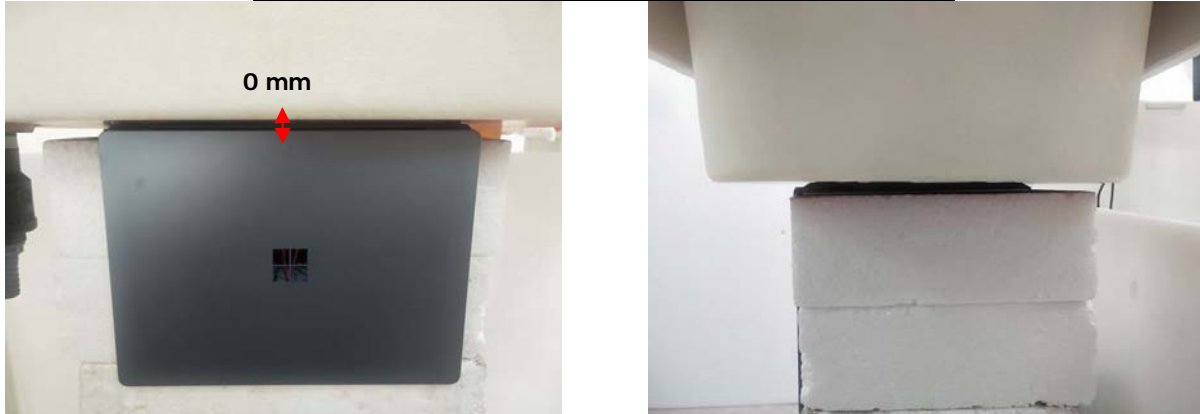
Fig.3 EUT Bottom side to flat phantom
