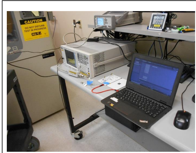
RF ANTENNA PORT CONDUCTED
