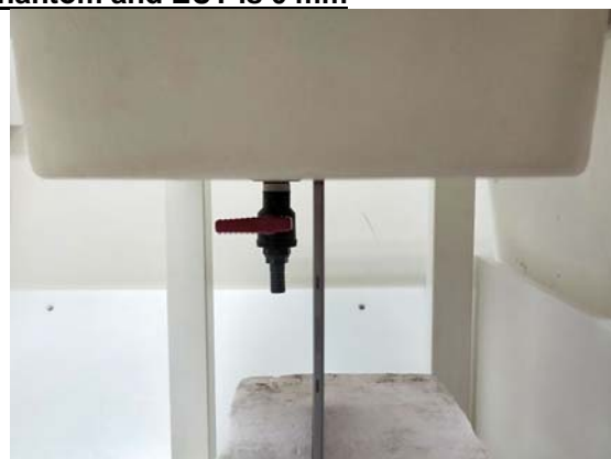
Fig.6 EUT Right side to flat phantom
