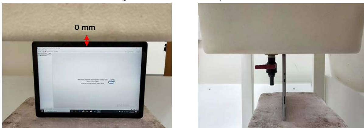
Fig.4 EUT Top side to flat phantom
