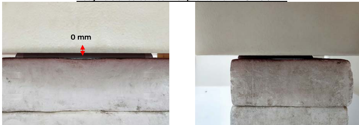
Fig.3 EUT Back side to flat phantom
