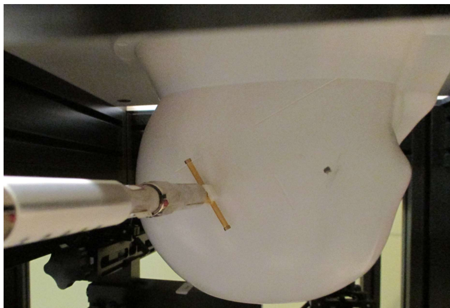
2.4 GHz Dipole Placed at Location A in 90° Orientation (10mm Spacer)
