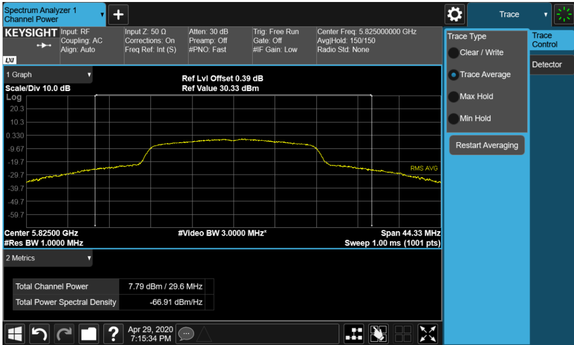
Plot 9-59. Maximum Conducted Output Power Chain A 802.11a (Ch. 165)
