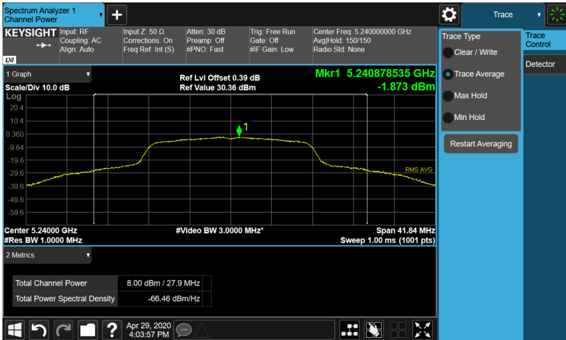
Plot 9-33. Maximum Conducted Output Power and PSD Chain A 802.11a (Ch. 48)
