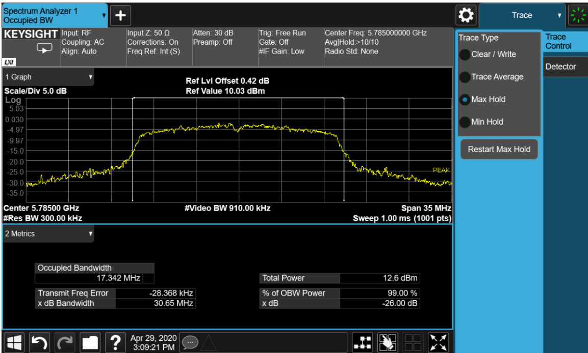
Plot 9-11. 26-dB Emission Bandwidth and 99% OBW Chain A 802.11a (Ch. 157)
