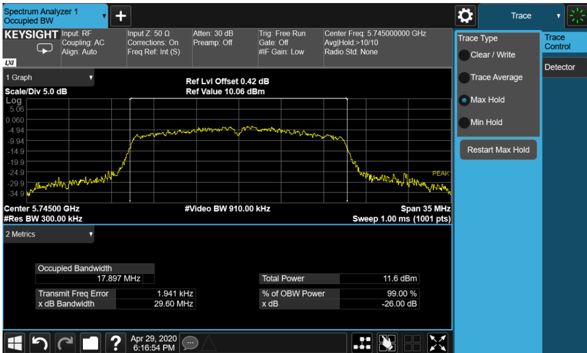
Plot 9-22. 26-dB Emission Bandwidth and 99% OBW Chain A 802.11n HT20 (Ch. 149)
