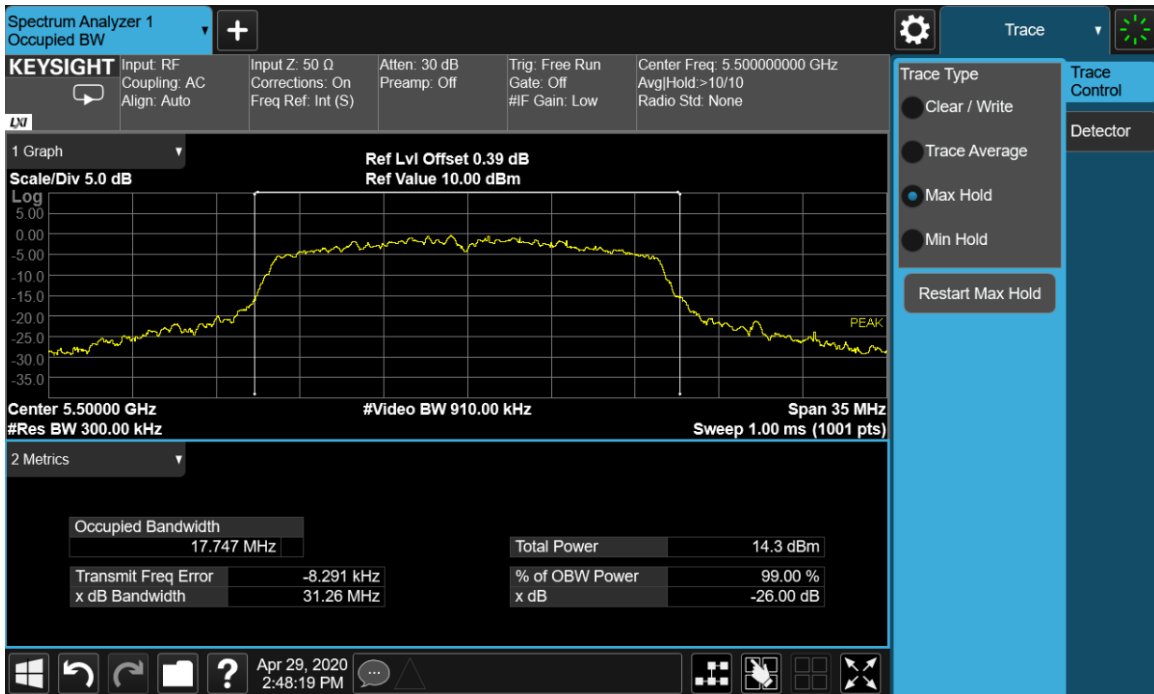
Plot 9-7 . 26-dB Emission Bandwidth and 99% OBW Chain A 802.11a (Ch. 100)
