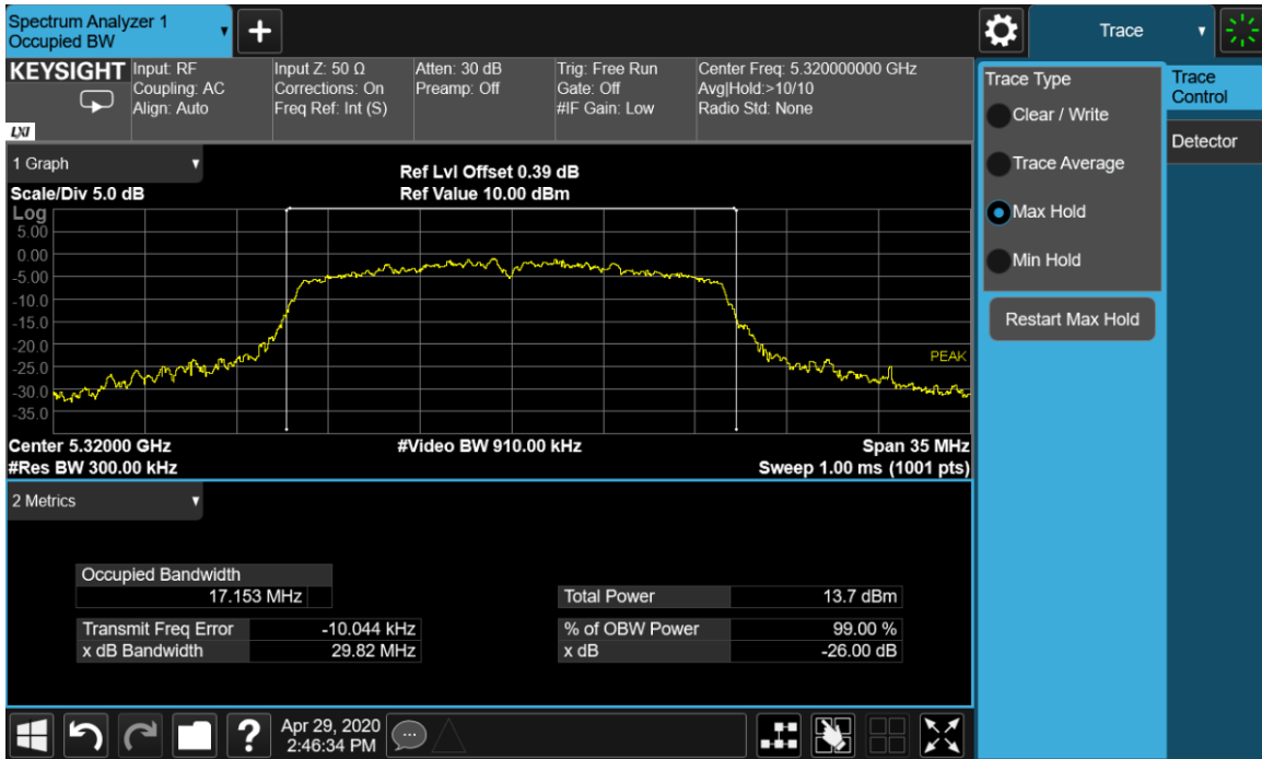
Plot 9-6. 26-dB Emission Bandwidth and 99% OBW Chain A 802.11a (Ch. 64)
