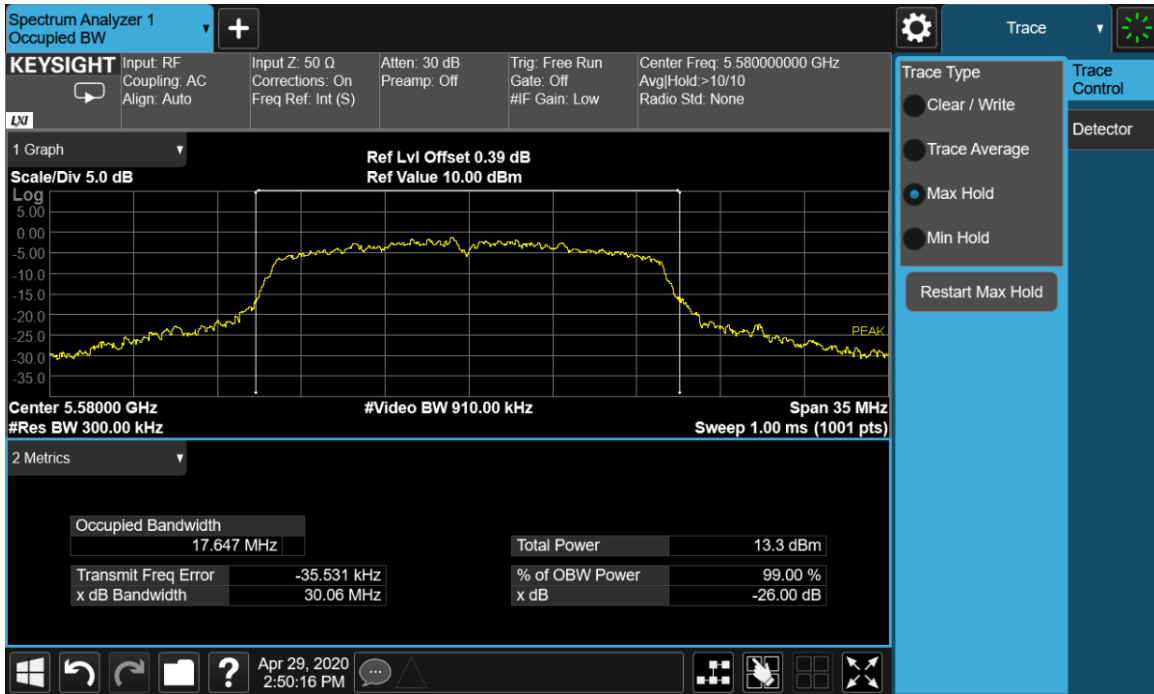
Plot 9-8. 26-dB Emission Bandwidth and 99% OBW Chain A 802.11a (Ch. 116)
