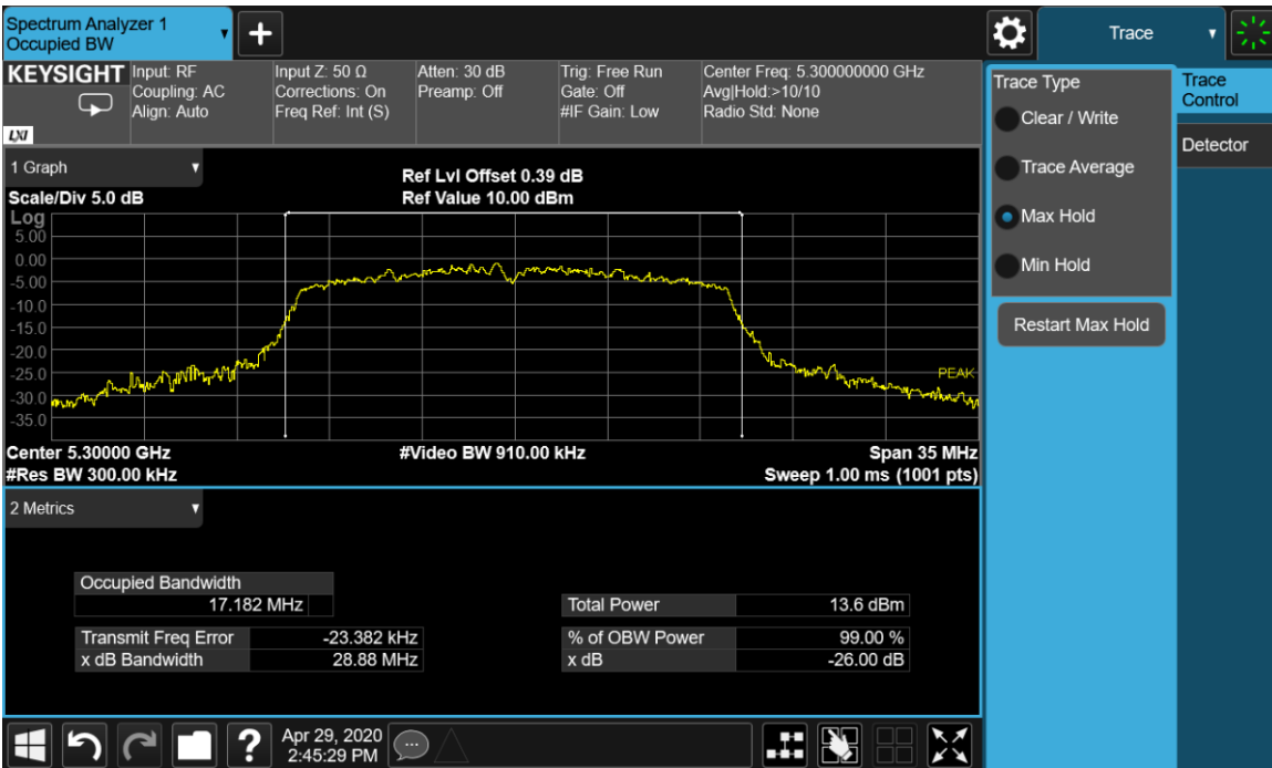
Plot 9-5. 26-dB Emission Bandwidth and 99% OBW Chain A 802.11a (Ch. 60)
