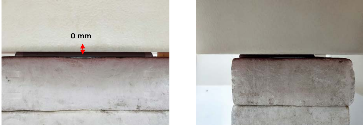
Fig.3 EUT Back side to flat phantom
