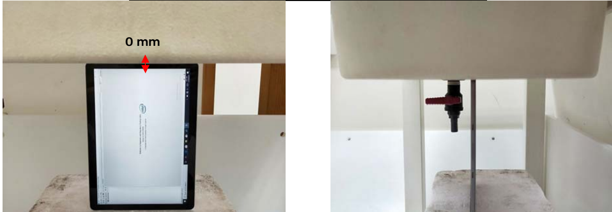
Fig.6 EUT Right side to flat phantom
