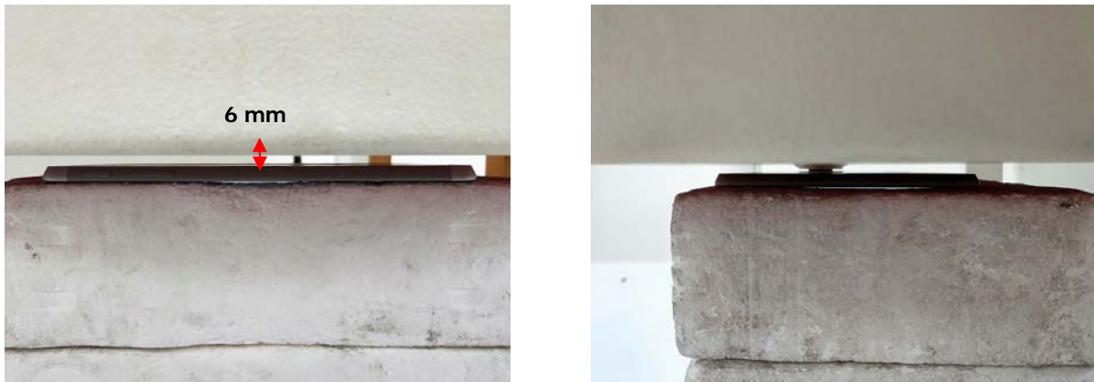
Fig.10 EUT Back side to flat phantom
