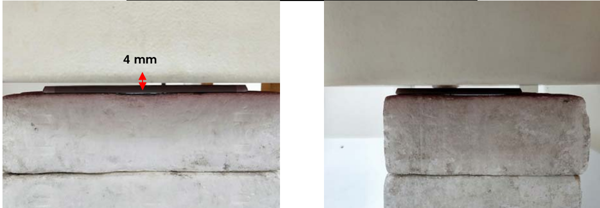
Fig.8 EUT Back side to flat phantom
