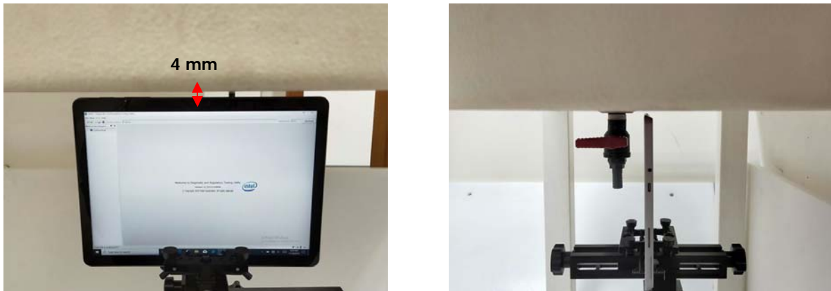
Fig.9 EUT Top side to flat phantom
