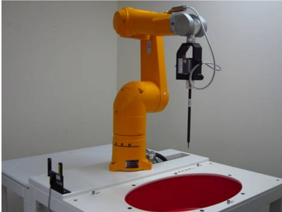
Fig.1 Photograph of the SAR measurement system
