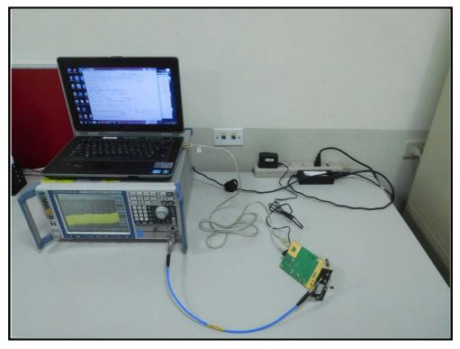
CONDUCTED EMISSION TEST (Chain 1)
