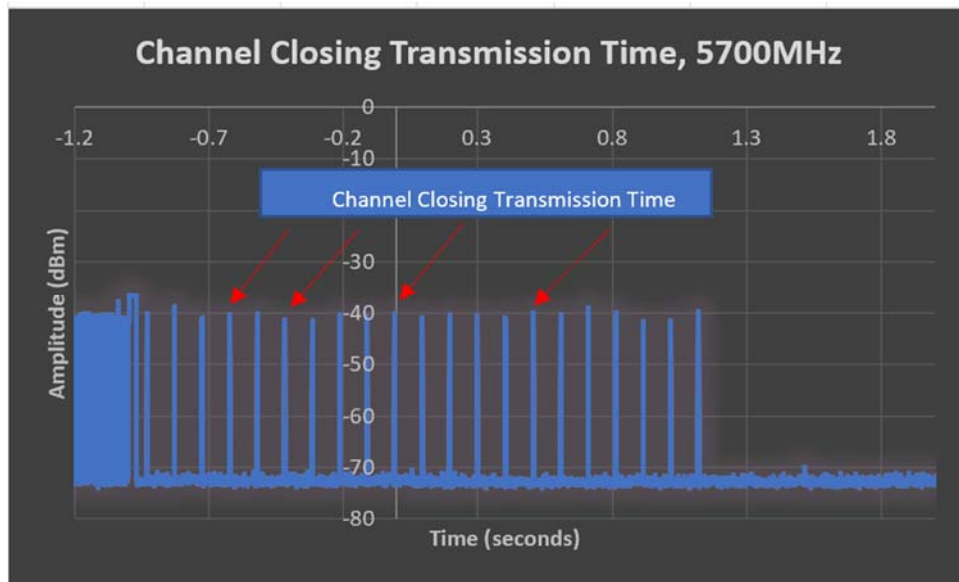
Figure 27. Channel Closing Transmission Time (5700MHz), 20MHz Bandwidth
