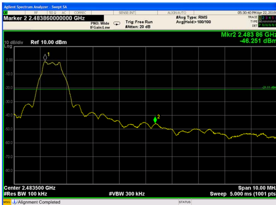
Figure 9-24 Conducted- High Band Edge (Ch. 39)
