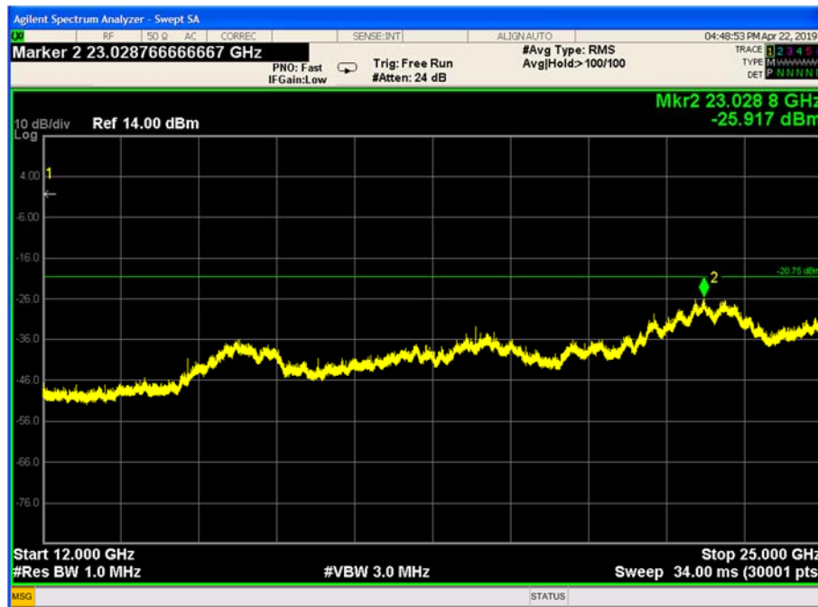
Figure 9-16 Conducted Spurious Emissions 12-25 GHz (Ch.0)
