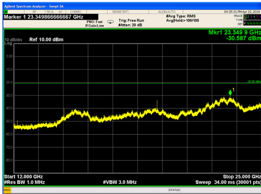
Figure 9-19 Conducted Spurious Emissions 12-25 GHz (Ch. 19)
