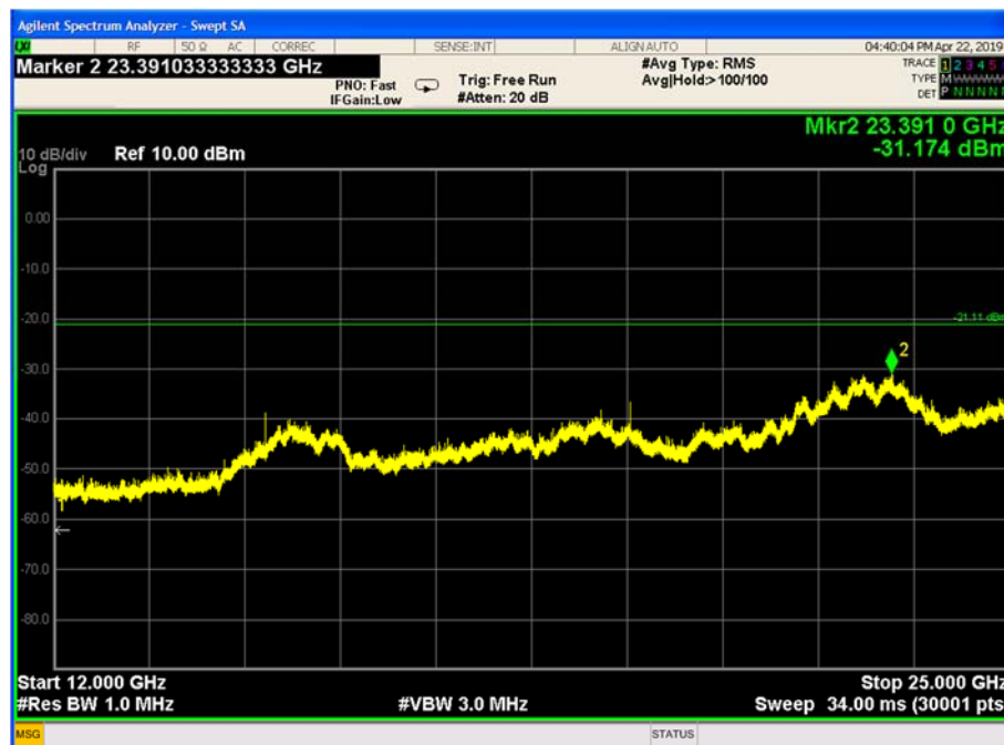
Figure 9-22 Conducted Spurious Emissions 12-25GHz (Ch.39)
