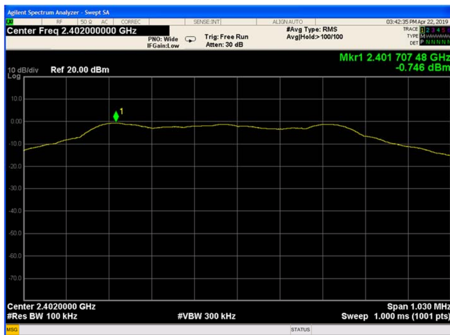
Figure 9-14 Reference Level Measurement (Ch.0)
