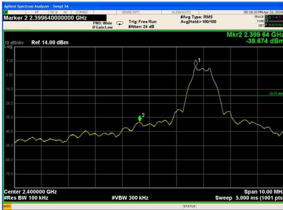
Figure 9-23 Conducted-Low Band Edge (Ch. 0)
