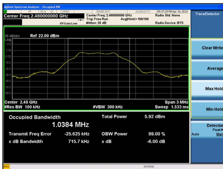
Figure 9-4 6dB Bandwidth (Ch. 39)
