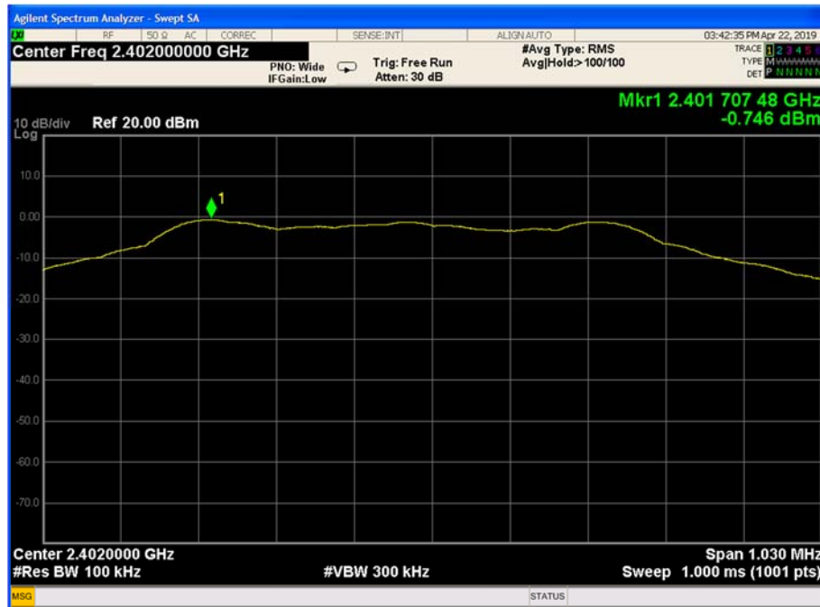
Figure 9-11 Power Spectral Density (Ch. 0)
