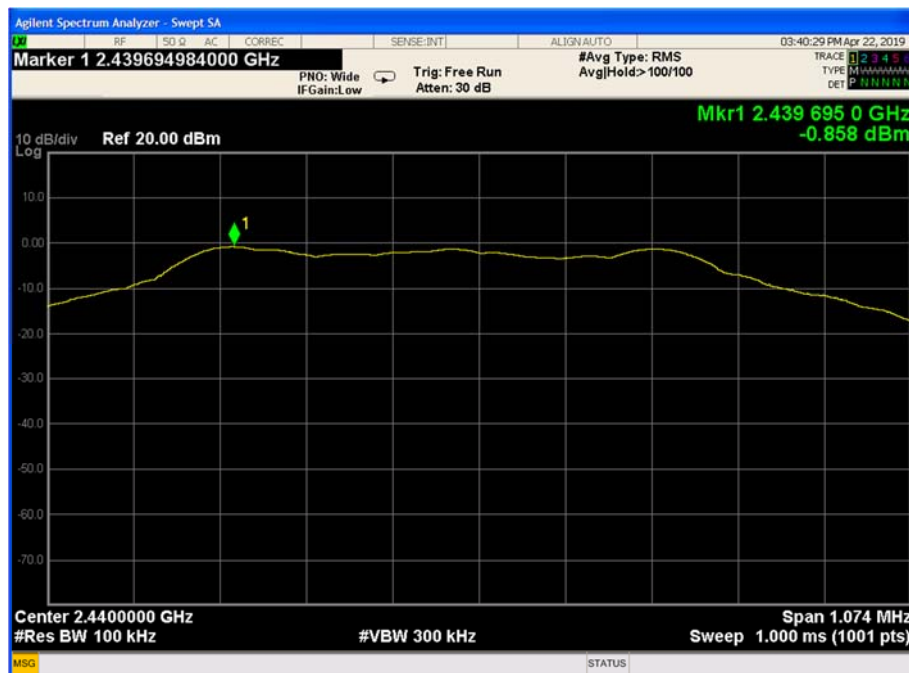
Figure 9-12 Power Spectral Density (Ch. 19)
