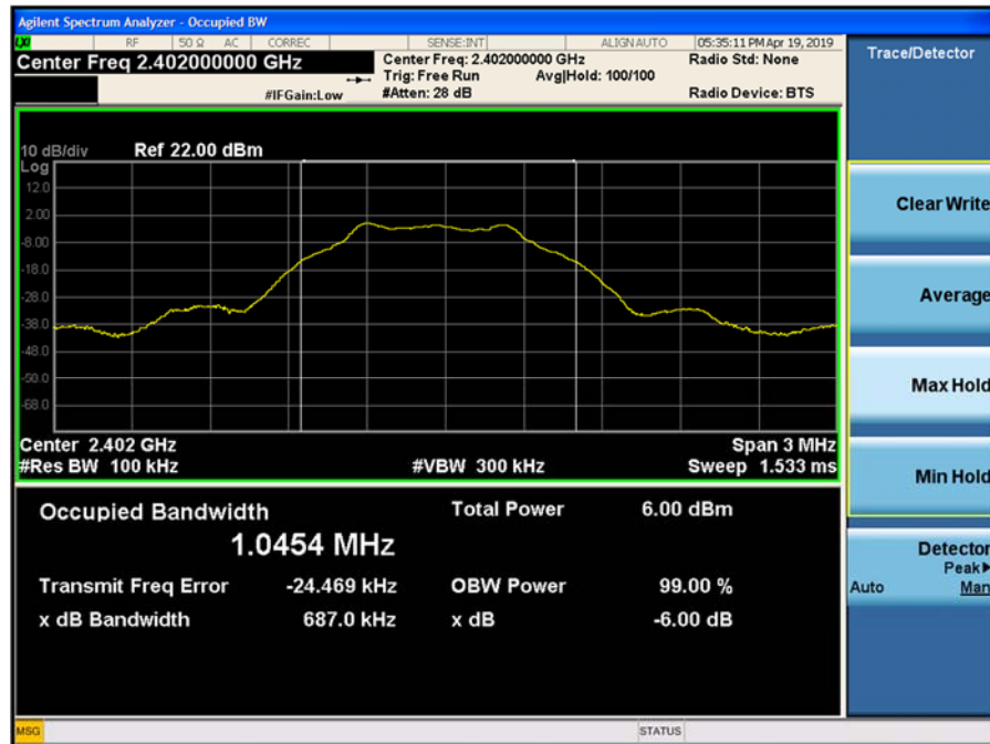
Figure 9-2 6dB Bandwidth (Ch. 0)
