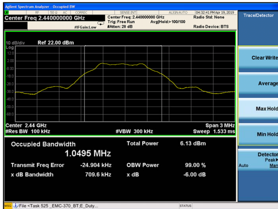
Figure 9-3 6dB Bandwidth (Ch. 19)
