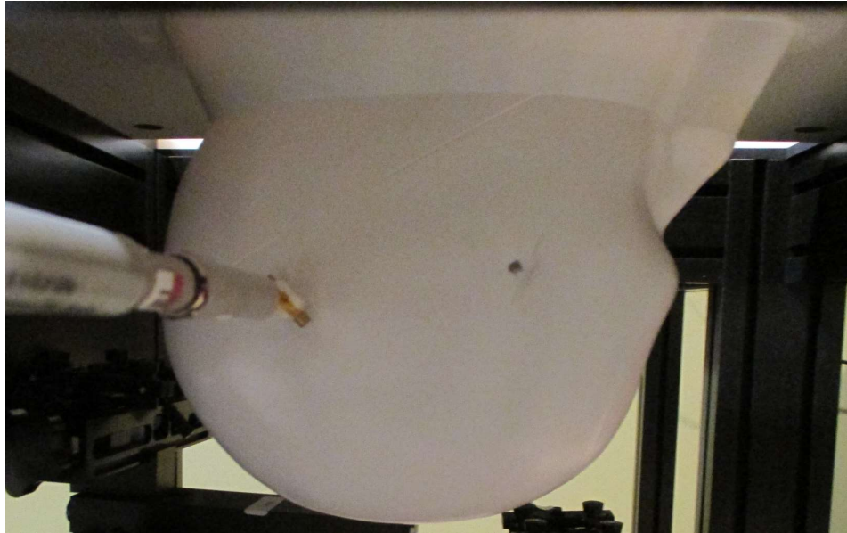
5 GHz Dipole Placed at Location A in 90° Orientation (10mm Spacer)
