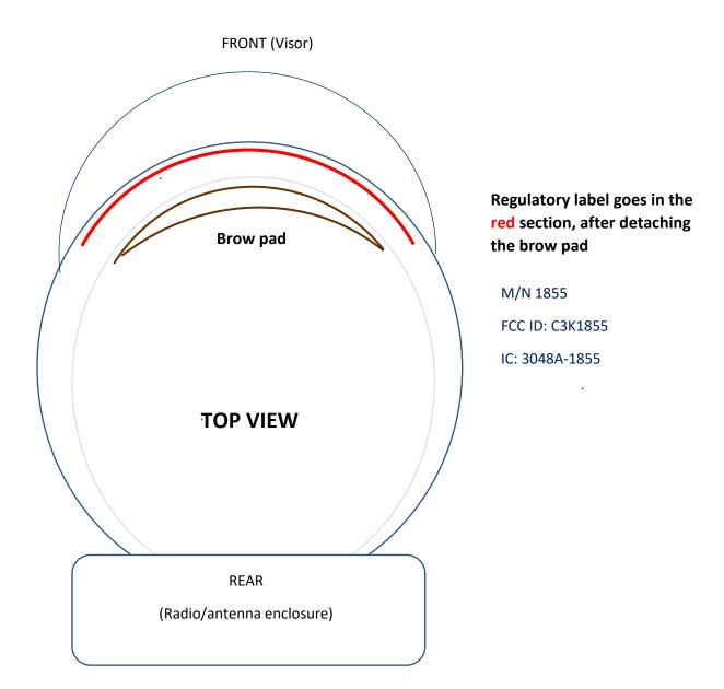
Label located on the front side, behind the visor and is visible after the brow pad is detached.
