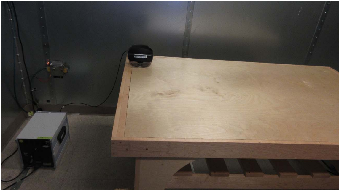
Figure 7 AC Line Conducted Emissions Test Setup -Front View
