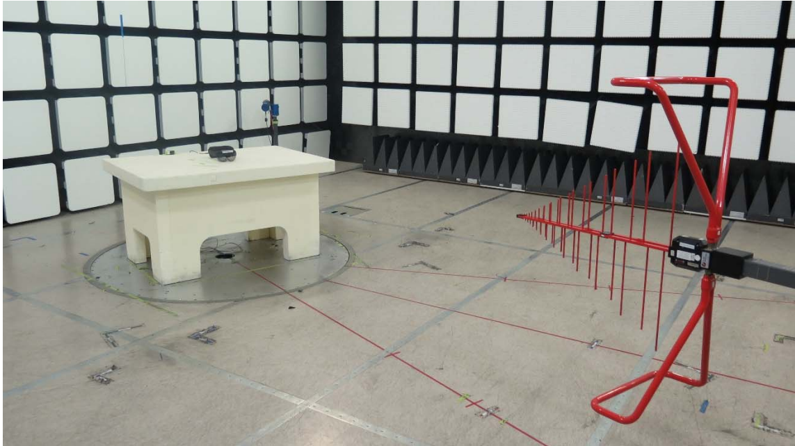
Figure 1 Radiated Spurious Emissions Test Setup (30M-1GHz)
