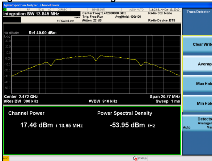
Figure 9-97 Chain 0 Average Power 802.11b - Ch.13
