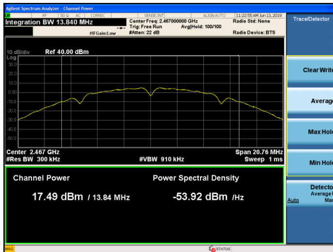
Figure 9-95 Chain 0 Average Power 802.11b - Ch.12
