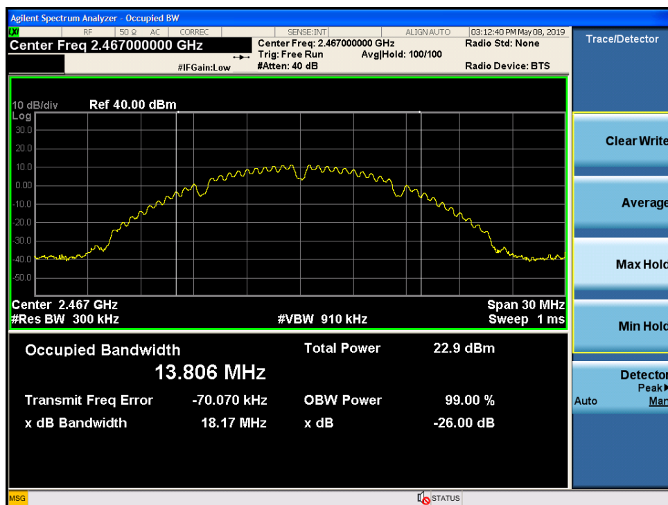
Figure 9-56 Chain 1 99% Bandwidth 802.11b - Ch.12
