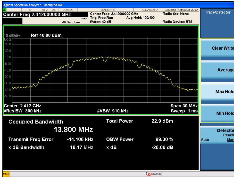
Figure 9-50 Chain 1 99% Bandwidth 802.11b - Ch.1
