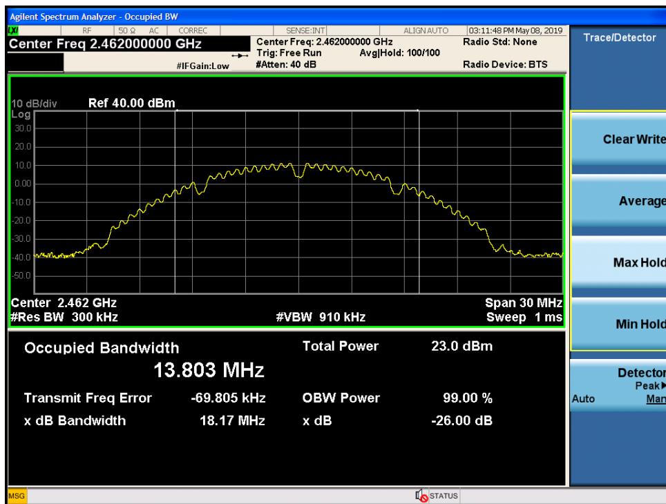
Figure 9-54 Chain 1 99% Bandwidth 802.11b - Ch.11
