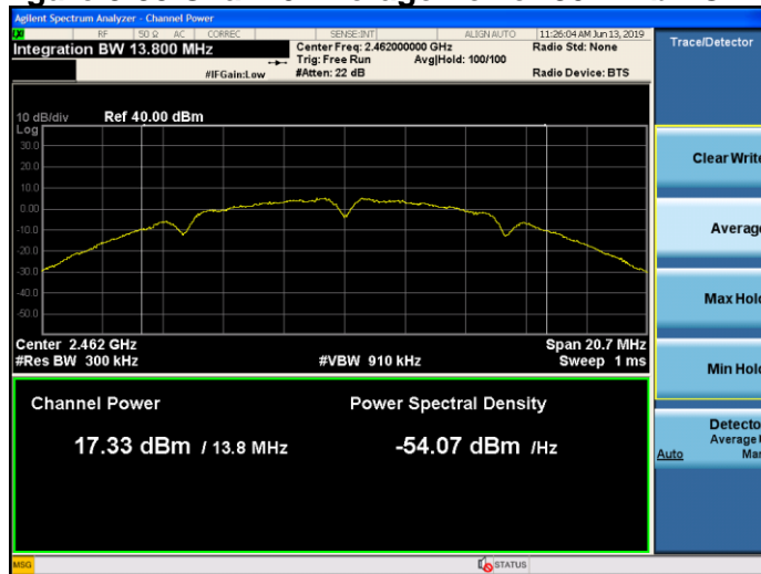
Figure 9-94 Chain 1 Average Power 802.11b - Ch.11
