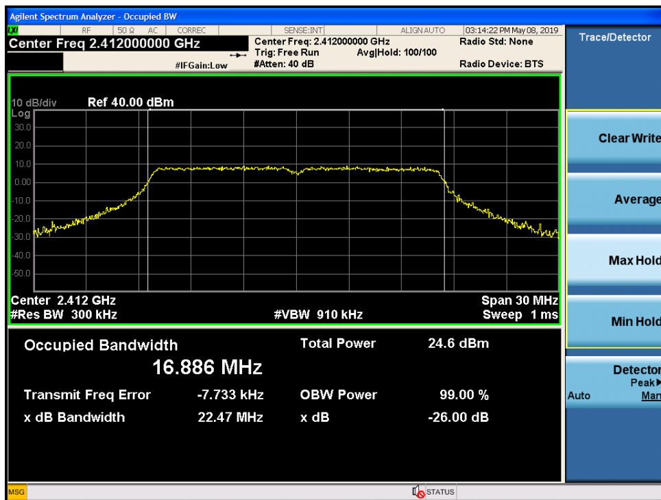
Figure 9-60 Chain 1 99% Bandwidth 802.11g - Ch.1
