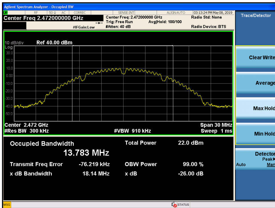
Figure 9-58 Chain 1 99% Bandwidth 802.11b - Ch.13
