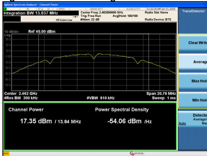
Figure 9-93 Chain 0 Average Power 802.11b - Ch.11
