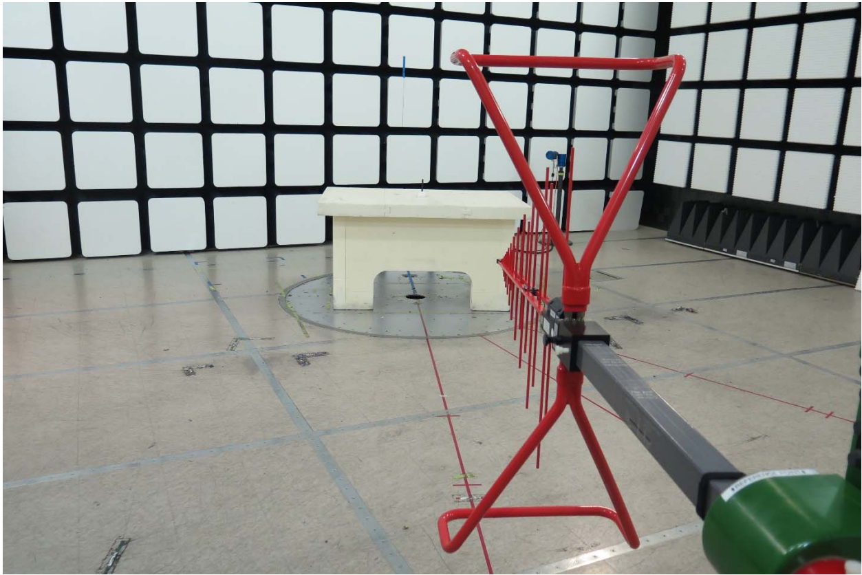
Figure 2 Radiated Spurious Emissions Test Setup (30M-1GHz)
