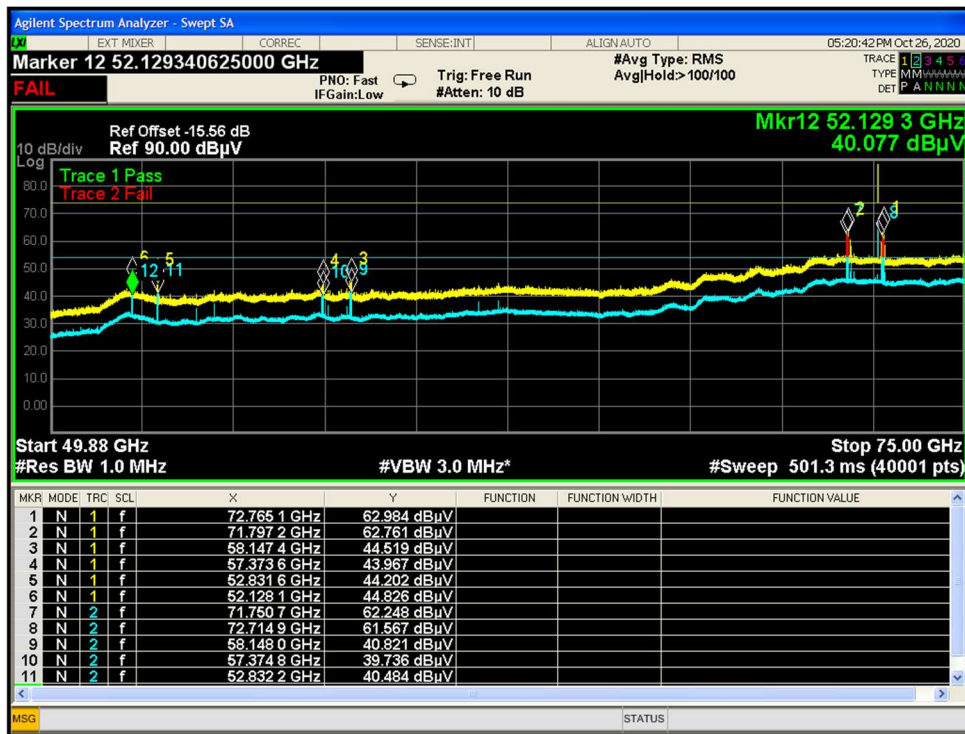
Figure 9-14. Radiated Spurious Emissions 24.2 GHz SRD_Pre Scan_Horizontal (50-75 GHz)
