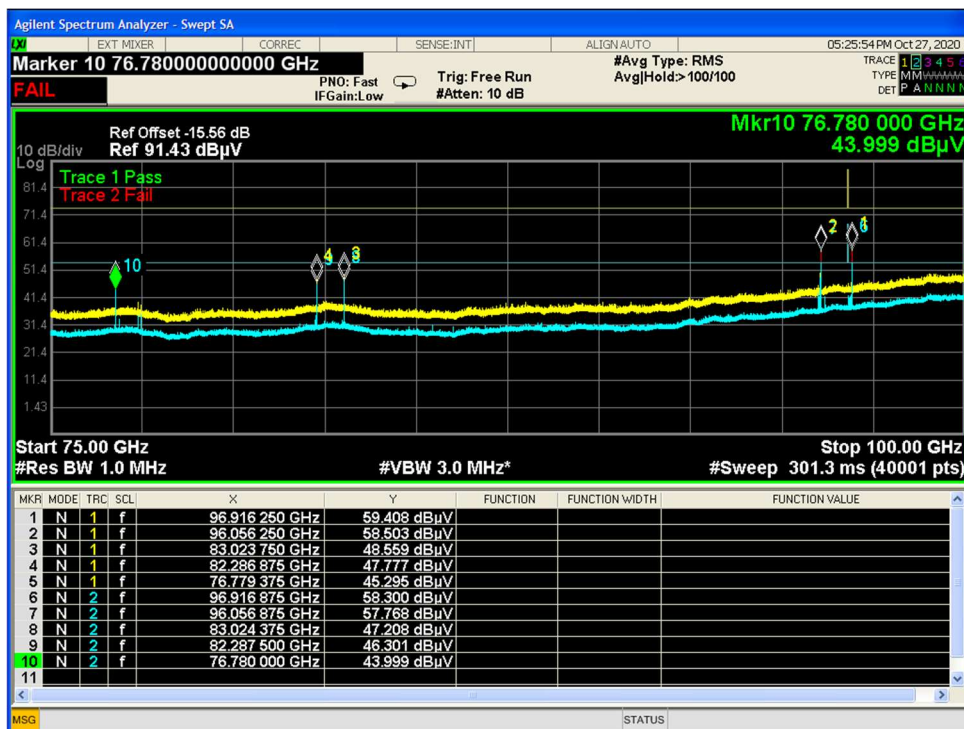
Figure 9-18. Radiated Spurious Emissions 24.2 GHz SRD_Pre Scan_Horizontal (75-100 GHz)
