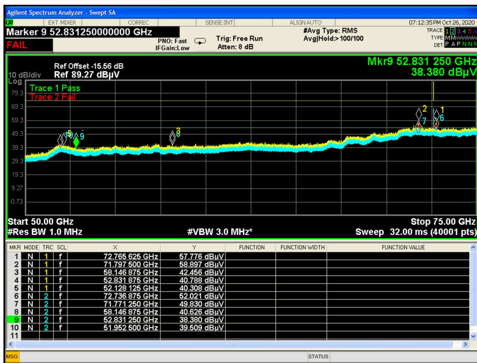
Figure 9-13. Radiated Spurious Emissions 24.2 GHz SRD_Pre Scan_Vertical_(50-75 GHz)
