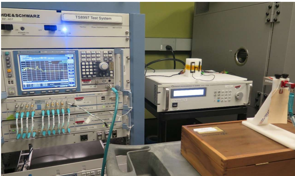
Figure 9: Occupied Bandwidth Measurement Setup
