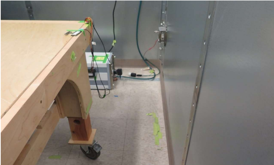
Figure 10: AC Line Conducted Emission Setup
