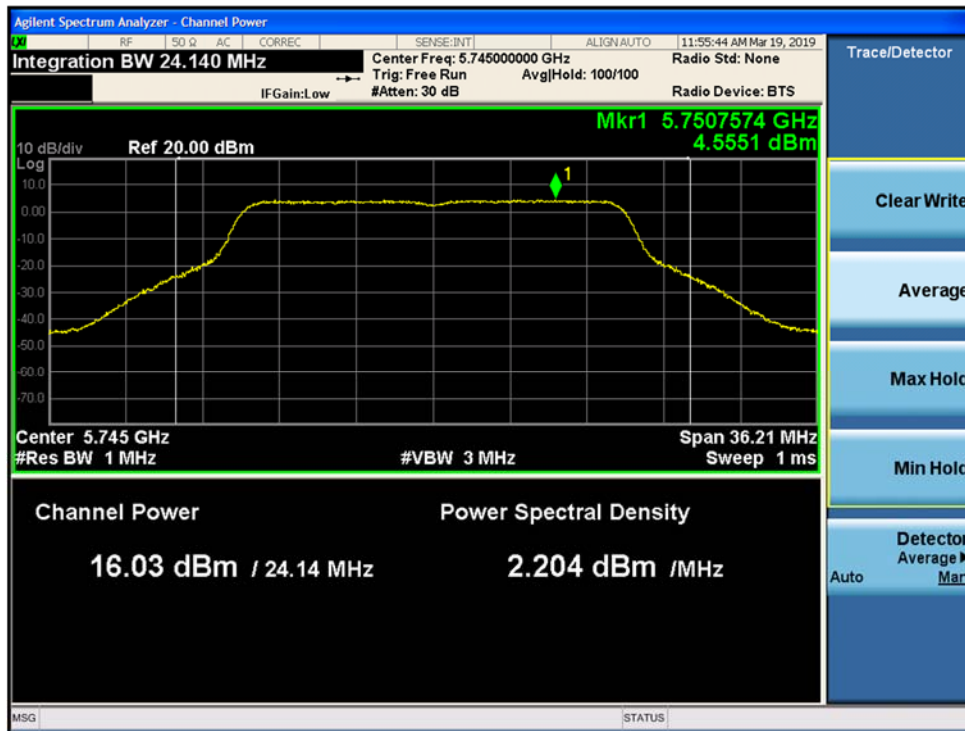
Figure 9-255. Maximum Conducted Output Power and PSD MIMO Chain A 802.11ac VHT20 (Ch. 149)
