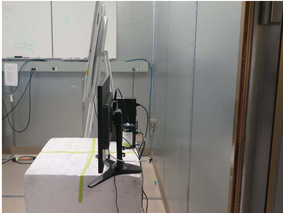
Figure 9 AC Line Conducted Emissions Test Setup -Side View
