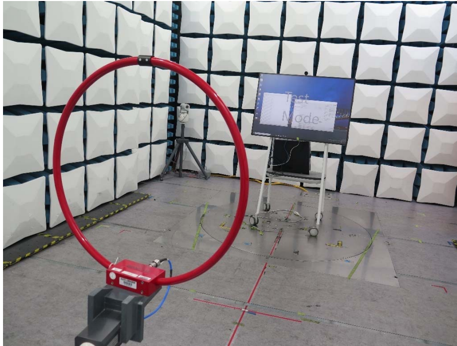
Figure 1 Radiated Spurious Emissions Test Setup (9k-30M)
