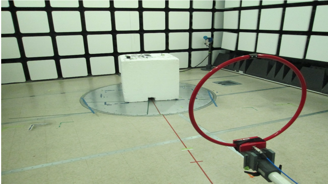
Figure 1 Radiated Spurious Emissions Test Setup (9K-30MHz)
