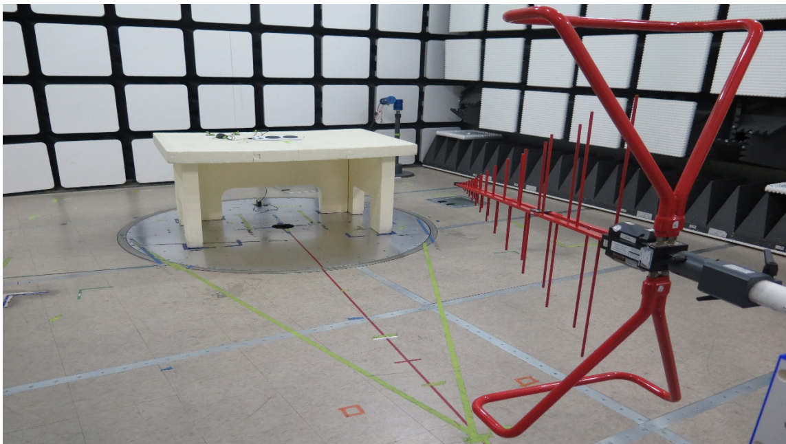
Figure 2 Radiated Spurious Emissions Test Setup (30M-1GHz)
